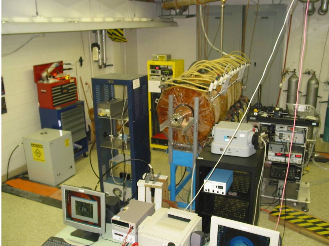
Figure 5.1: The ASTRAL helicon plasma source.
