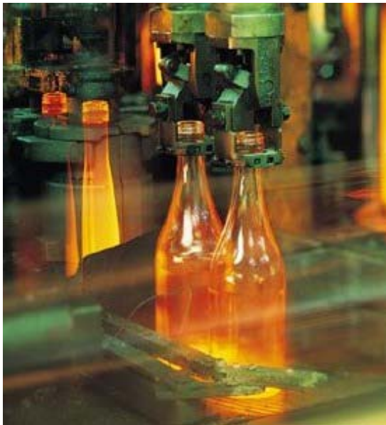
Figure 5: Bottle production equipment
