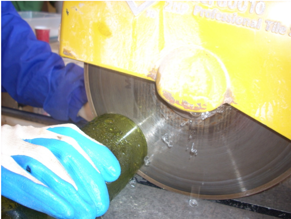
Figure 12: Cutting with a wet tile saw
