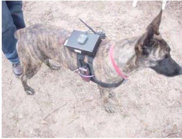
Figure 4.1: Remotely Commanded Canine with Radio and GPS/INS Receiver
