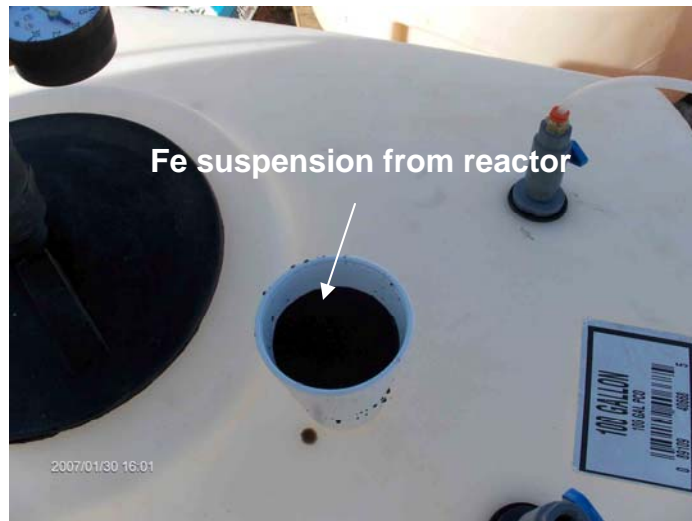
Figure 8-3. A picture of the CMC-stabilized Fe-Pd particles (Fe = 1g/L) taken from the reactor 5 min after preparation.
