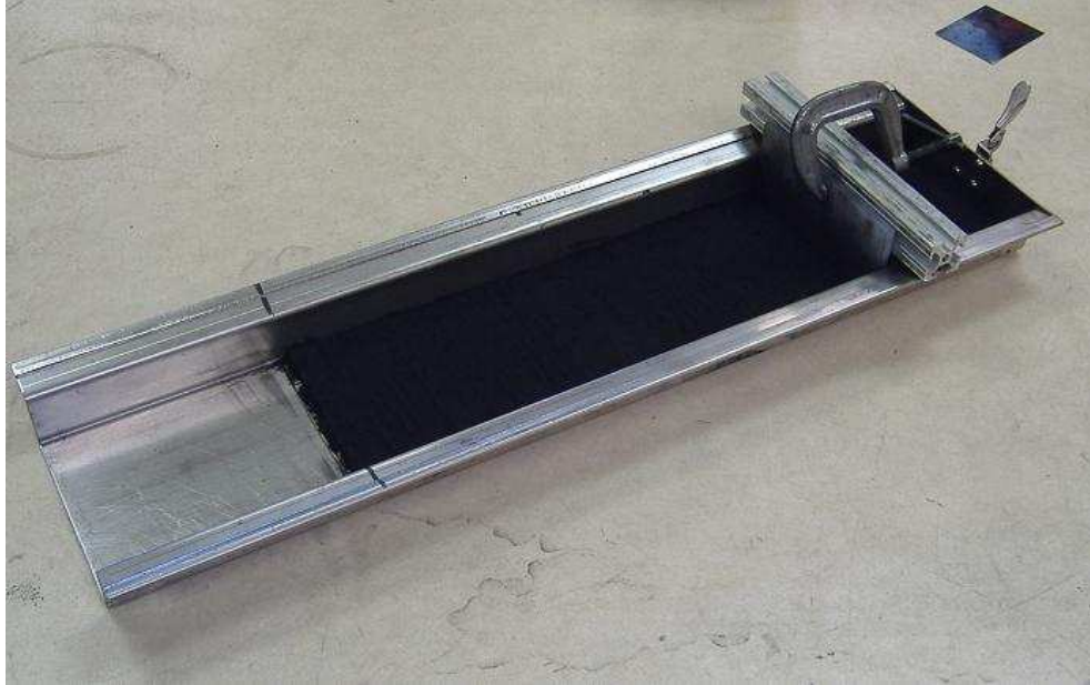
Figure 5.15: Loading Tray with leveling Tool
