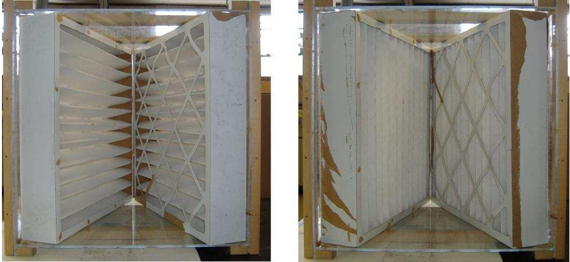
Figure 7.11: Horizontally-Oriented (Left) & Vertically-Oriented (Right) Banks
