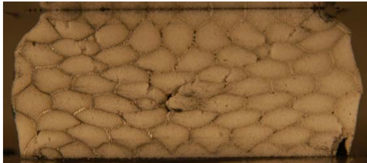
Figure 4.7: Deformation sequence for a SFH-30 sample at a applied strain of (1):0%, (2):3.2%, (3):5.8%, (4):8.8%, (5):12.6%, (6):16%, (7):24.6%, (8):30.2%, (9):36%, (10):42%
