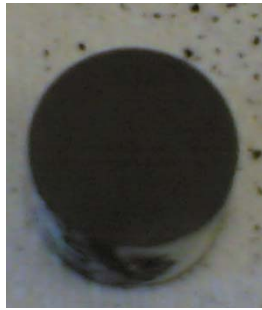
Figure 3.2: Syntactic foam sample with coating of graphite powder
