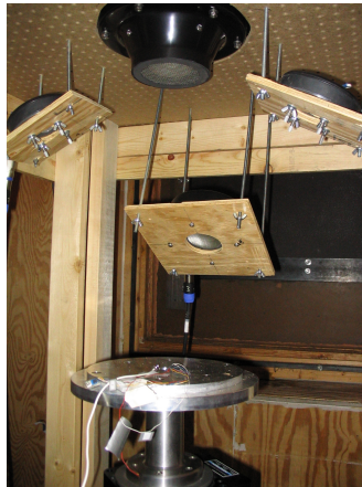
Figure 3.28: Configuration of the four drivers relative to the rate table
