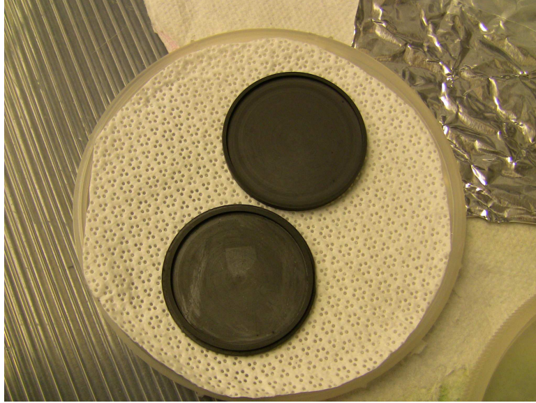
Fig. 4.8: Sample holder carbon box for implant activation.
