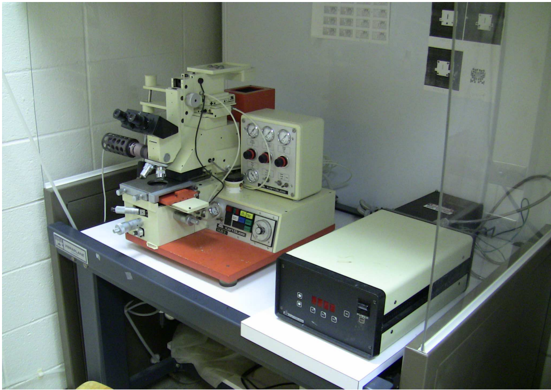
Fig. 4.4: Mask aligner for photo-lithography.
