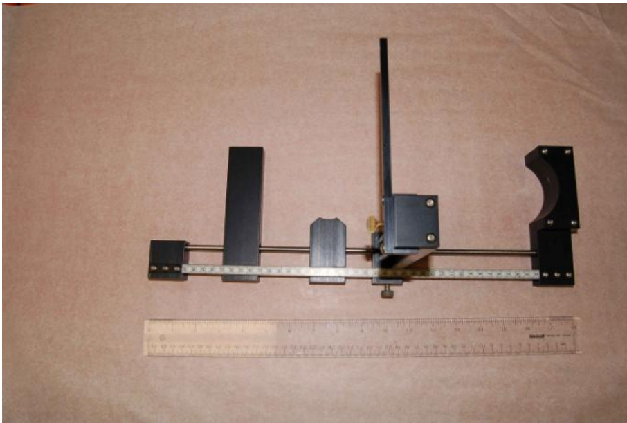
Figure 13. Arch Height Measurement Index device.
