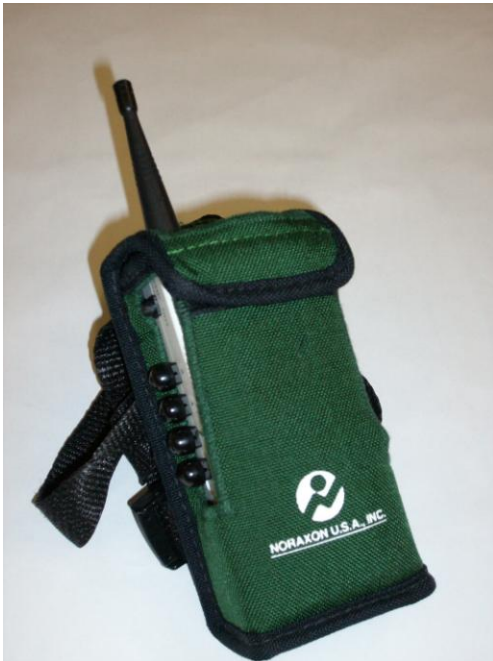
Figure 24. Noraxon Telemetry 2400T V2 wireless transmitter
