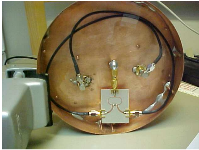
Figure 4.9: Power Splitter connected to the ports of the antenna
