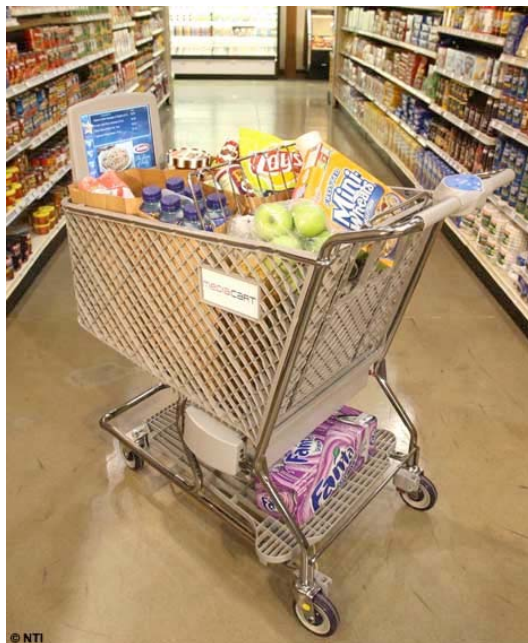
Figure 4. Mediacart (The Hi-tech Shopping Trolley That Tells You Where To Find Things in a Supermarket, 2008)
