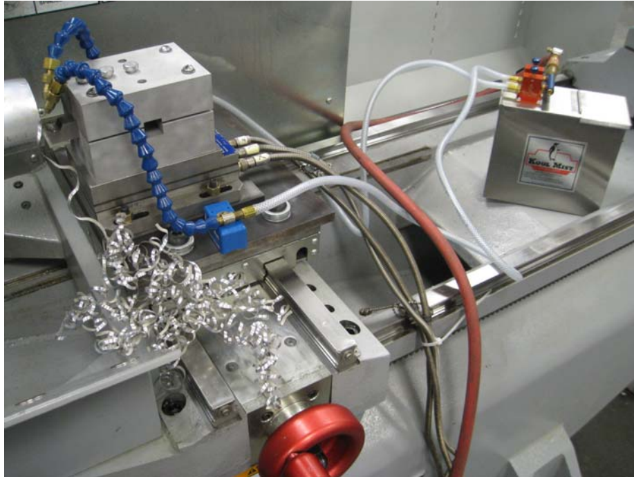
Figure 24: Turning at Spray Coolant Environment
