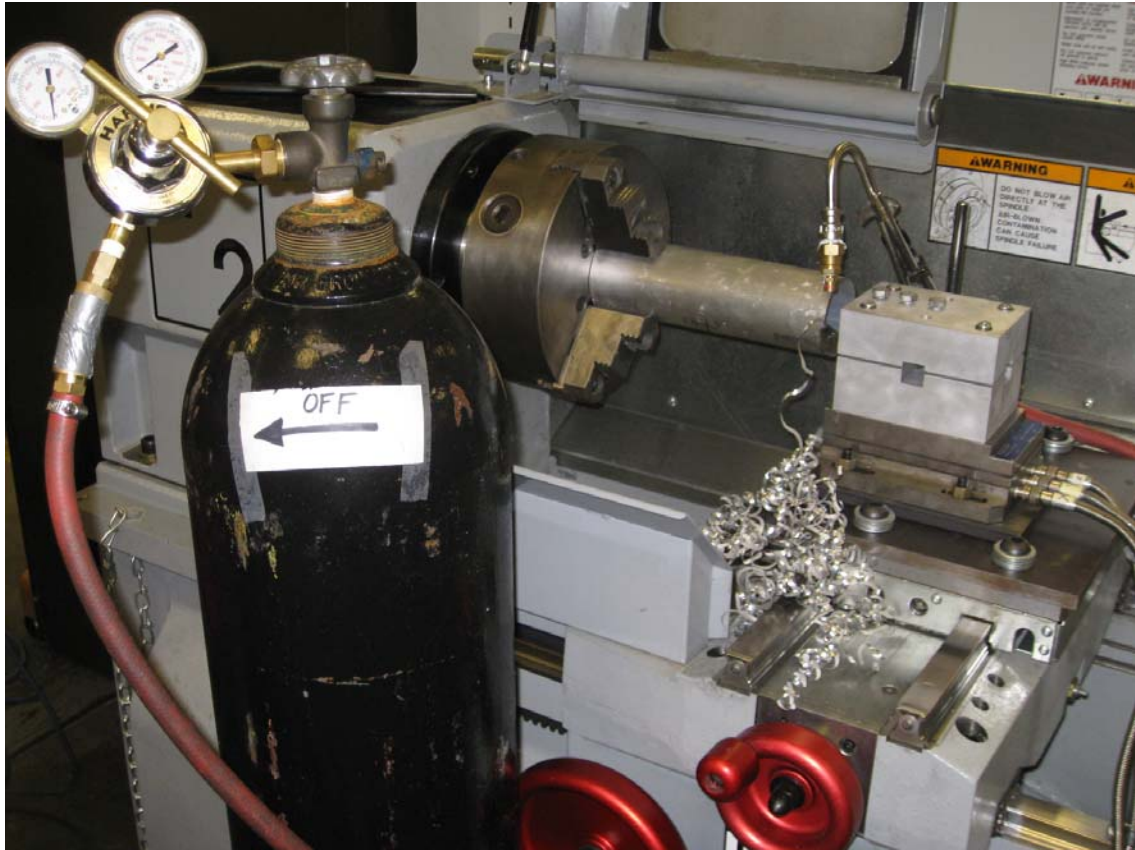
Figure 23: Turning at Nitrogen Gas Environment
