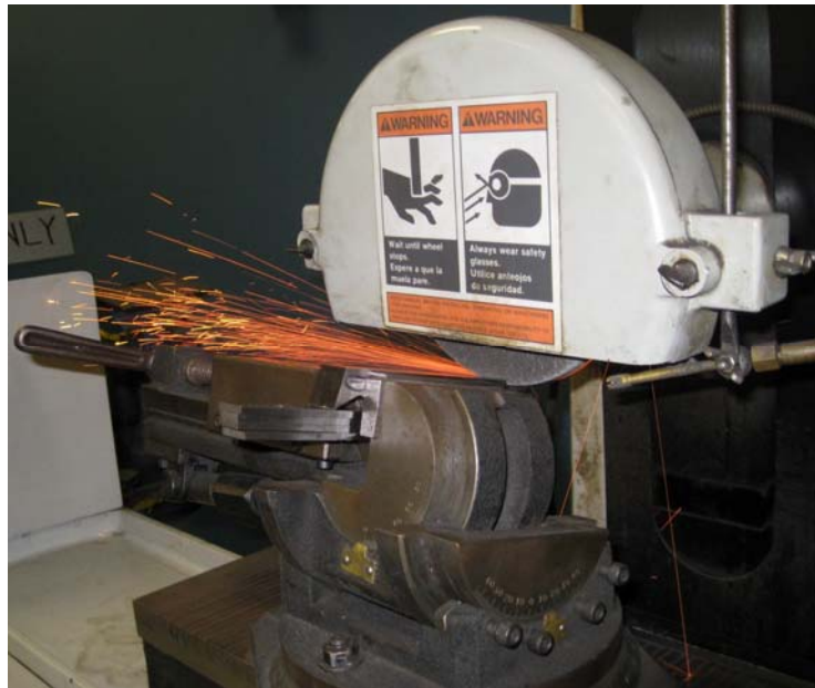
Figure 29: Machining a 30 degree tool on a HARIG 618 Automatic Surface Grinder
