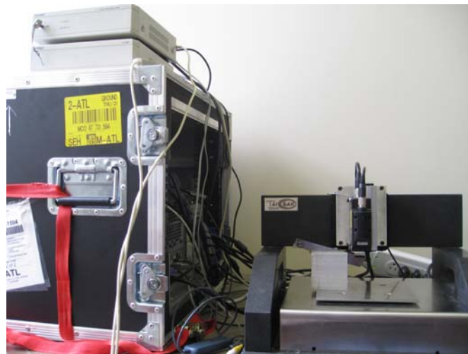
Figure 13: TaiCaan XYRIS Series Surface Profiler with a LT-8010 Sensor head, LT-V201 Camera Unit and a LT-8105 Controller unit.
