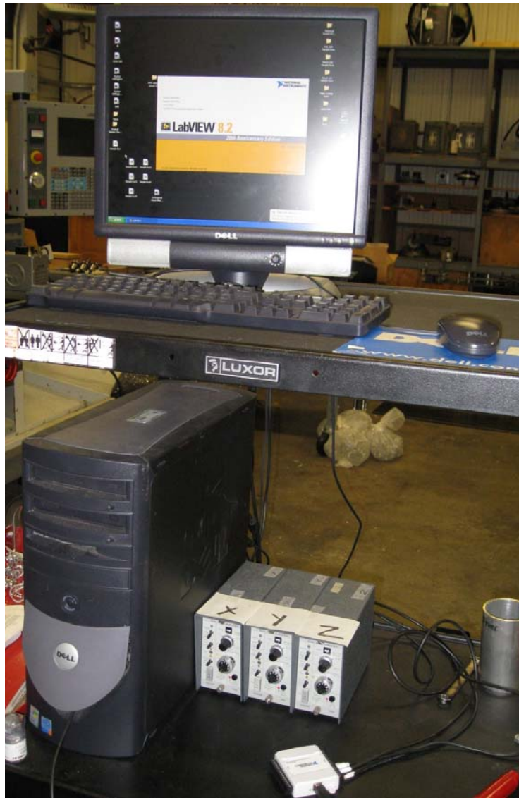
Figure 19: Charge Amplifiers and USB DAQ system module connected to the LABVIEW 8.2 system software
