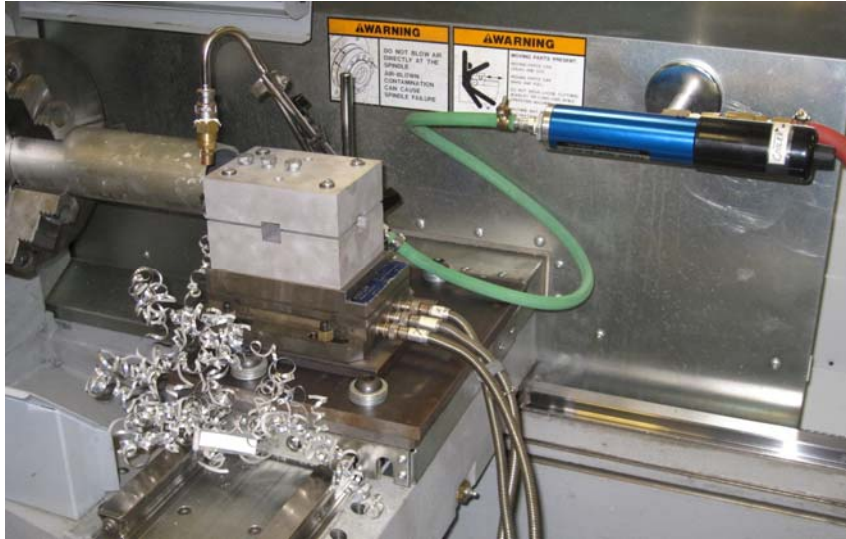
Figure 22: Turning at Cold Compressed Air Environment with Vortex Air Gun
