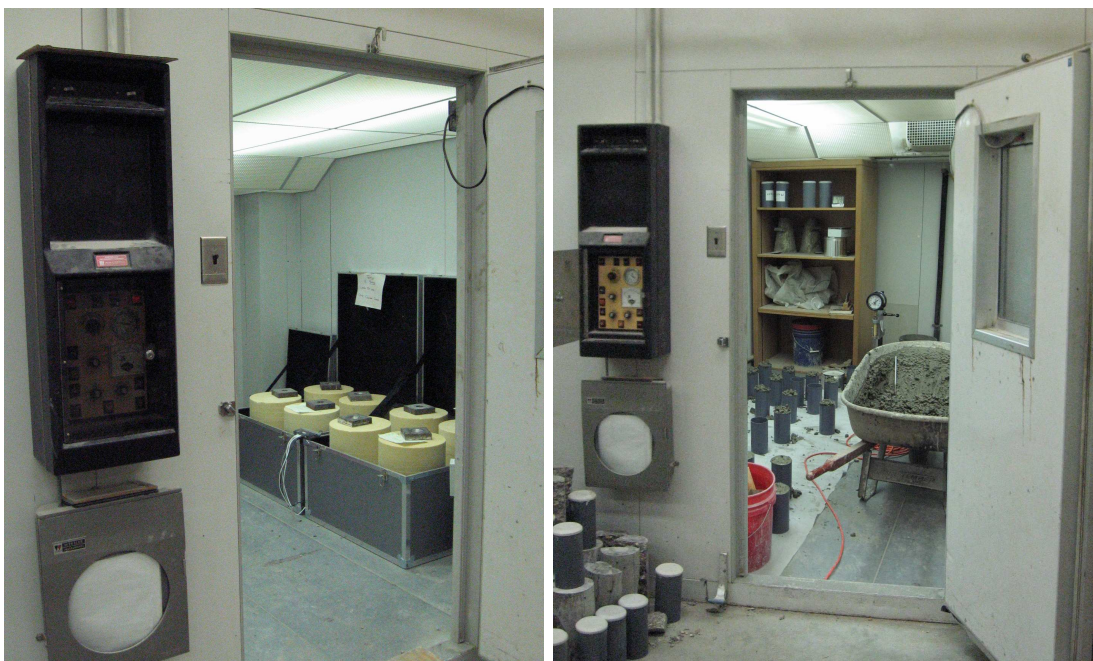
Figure 4.2: Insulated temperature controlled environmental chamber
