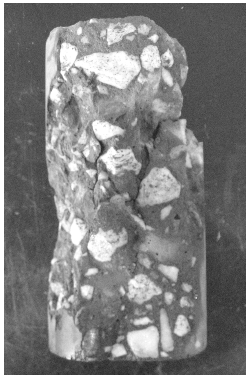
Figure 5.3: 30 % C-Cold Strength specimen which was visually inspected for signs of segregation
