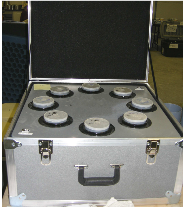
Figure B.4: Example of the Category II – 3x6 Device used by Groups 3, 5, 6, 7, 9, and 10
