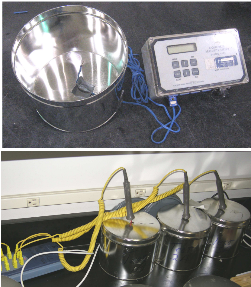
Figure 3.3: Temperature measuring devices for Group 3 (top) and Group 10 (bottom)
