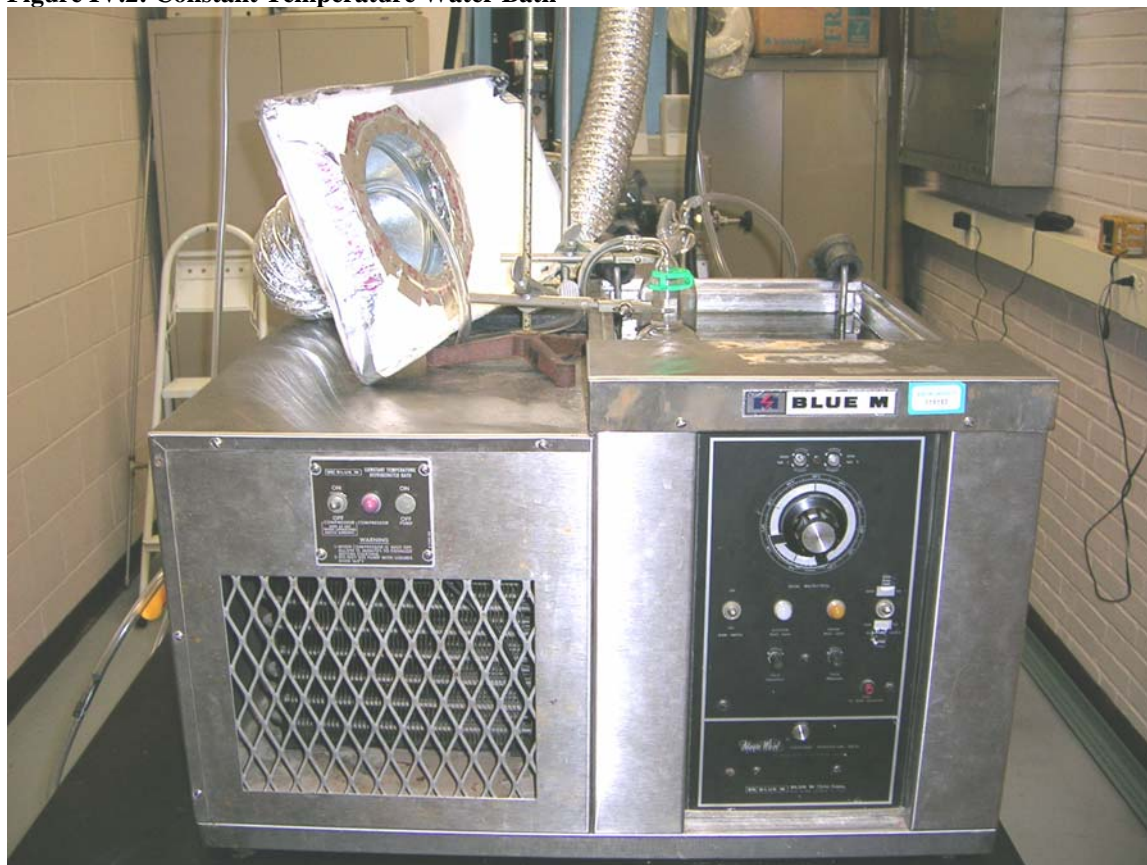
Figure IV.2: Constant Temperature Water Bath
