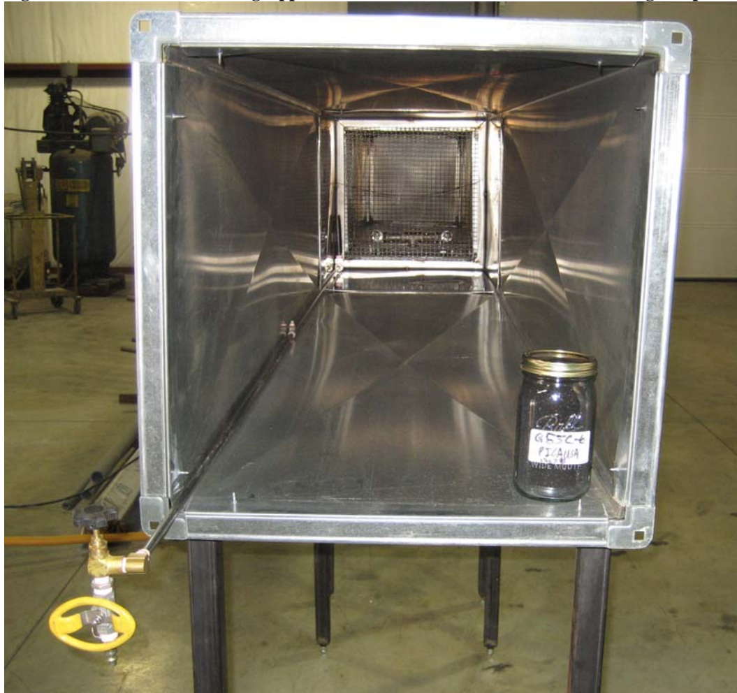
Figure V.3: Combustion Testing Apparatus with Sheet and Loose Particle Testing Peripherals
