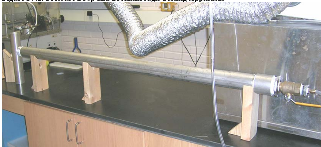
Figure IV.1: Pressure Drop and Breakthrough Testing Apparatus
