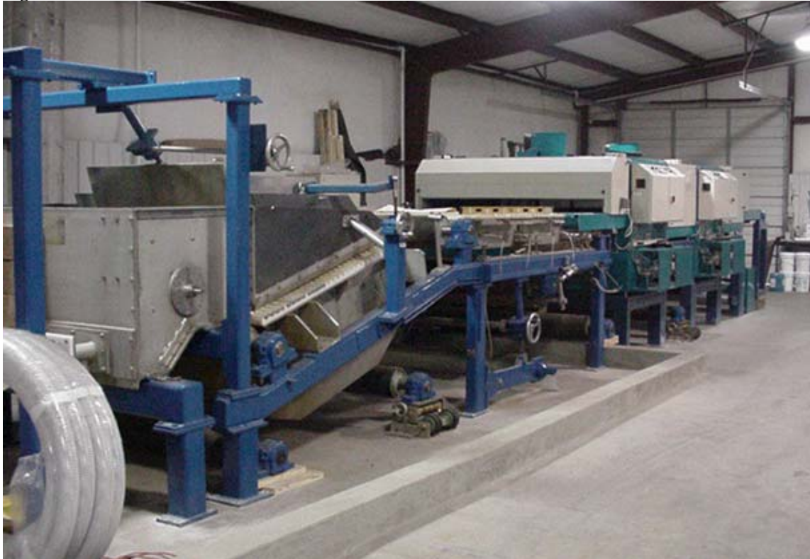
Figure III.7: 63 inch Inclined Wire Non-Woven Machine
