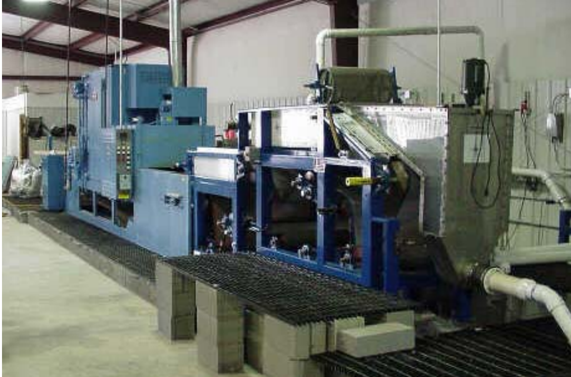
Figure III.6: 21 inch Inclined Wire Non-Woven Machine
