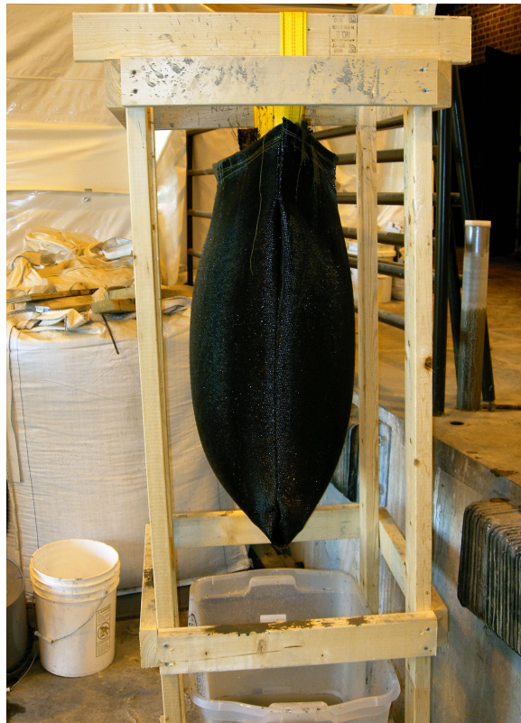
Figure 17: Hanging Bag Test Bag and Support Frame
