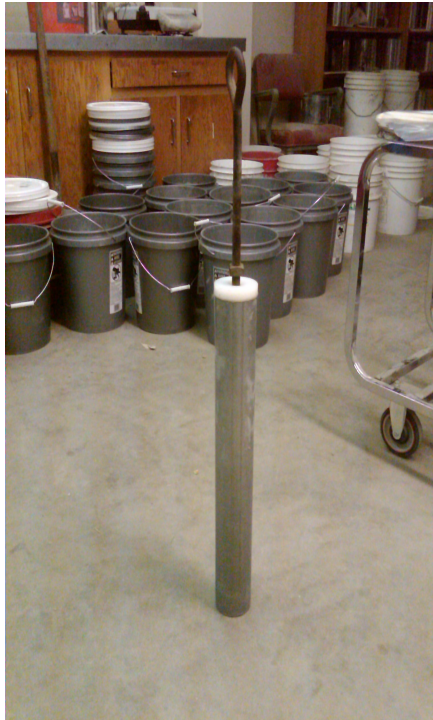
Figure 18: Modified Shelby tube for HBT sampling
