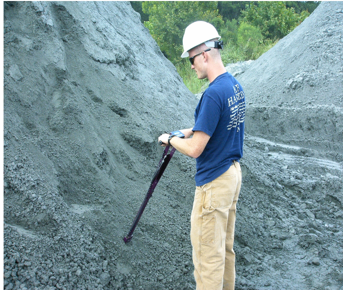
Figure 22: Fieldscout TDR 300 moisture probe in use in the field
