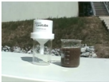
Figure 16: RDT Funnel (RDT Manual, 2009)
