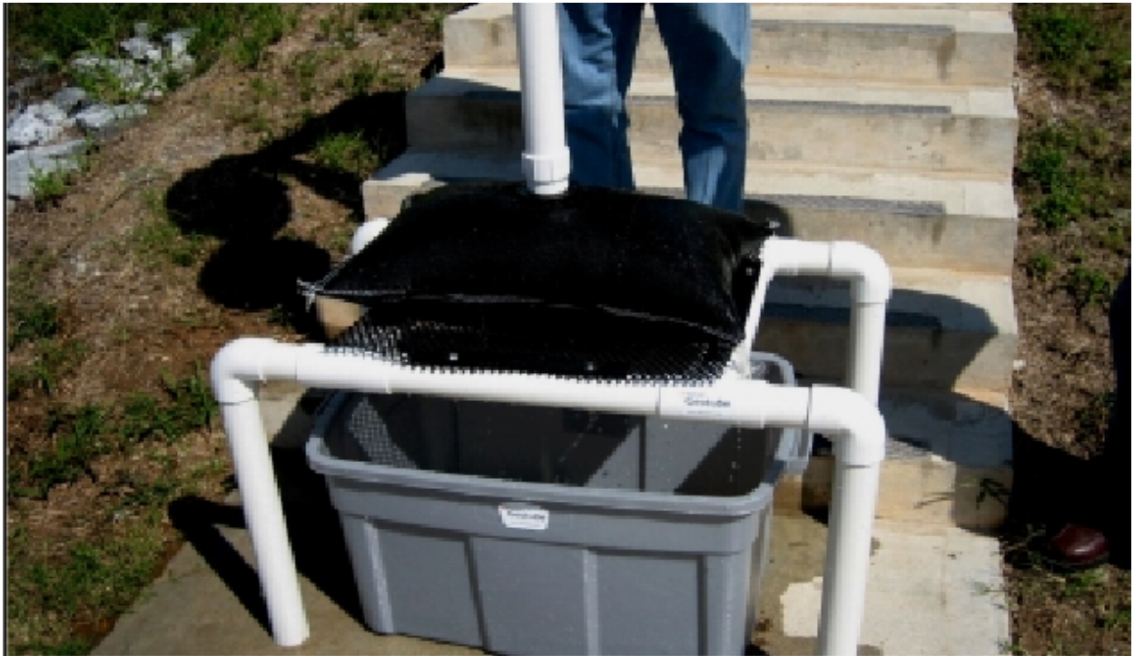
Figure 10: Geotube Dewatering Test (TenCate, 2009)
