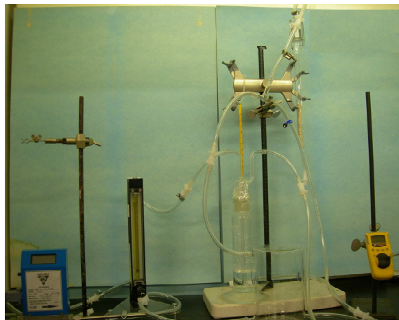
Figure 3.3 Schematic (top) and picture (bottom) of SO 2 adsorption test bench
