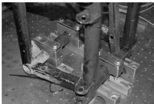
Figure 5.2: Physical constraints for the modal evaluation
