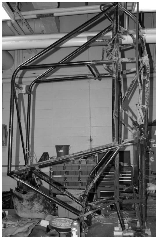
Figure 5.1: 2005 Baja SAE Frame under modal evaluation
