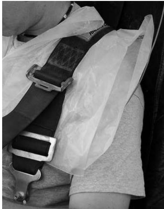
Figure 6.11: Detail of wax paper to provide low friction surface
