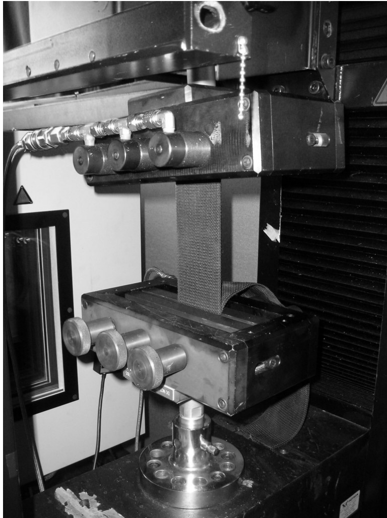
Figure 5.17: Detail of Belt Mounting
