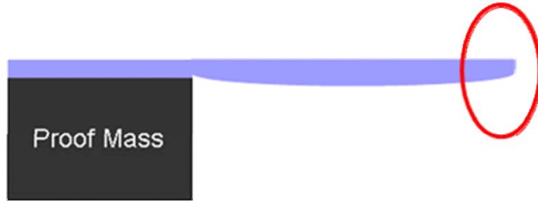
Figure 5.7 Concave etching profile after silicon etching
