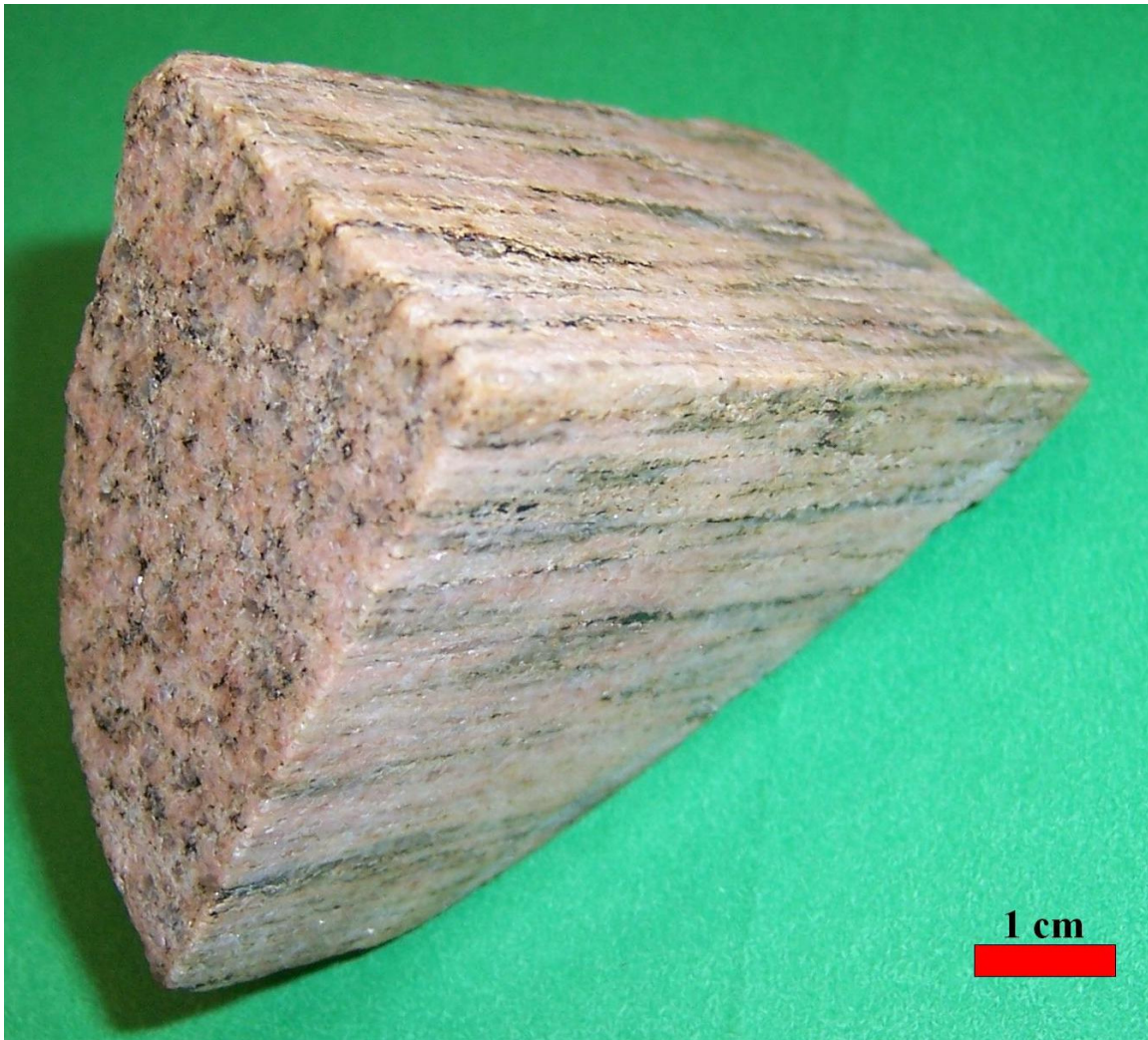
Figure 7. Orthogonally slabbed and polished L-tectonite from the core of the Sør fjord shear zone (Fig. 2). The two right-hand faces are cut parallel to the pencil lineation, and the view on the perpendicular face shows the complete lack of a planar fabric within the rock.
