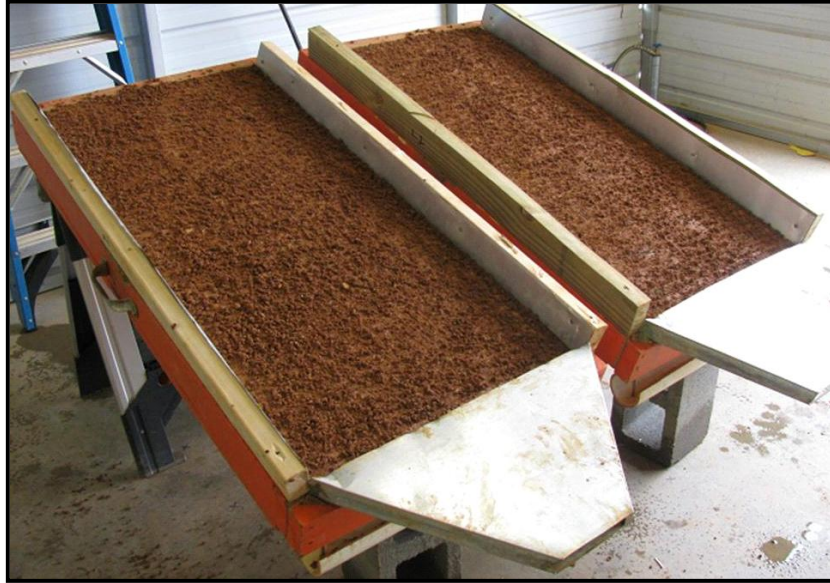
Figure 3.5 Sideboards Installed on Test Plots.
