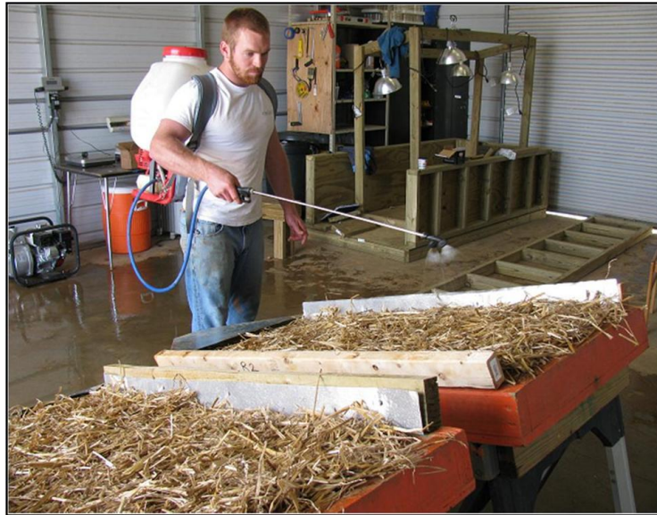
(b) Applying Tackifier to Prepared Test Plots
