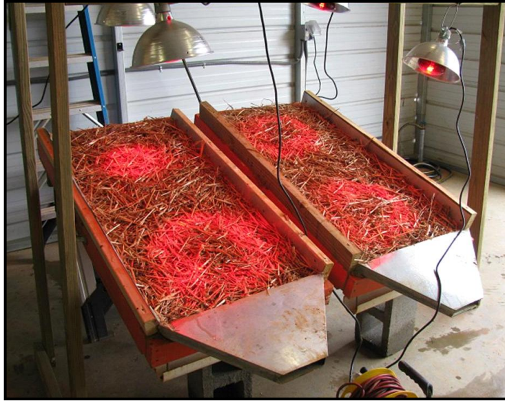
Figure 3.23 Conventional Straw with Tackifier for 48 hr Drying Period.
