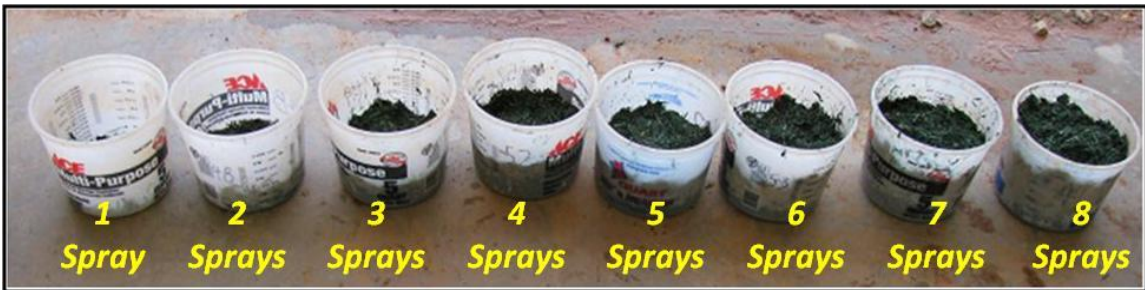
Figure 3.29 Hydromulch Scraped off of Test Boards into Corresponding Buckets.
