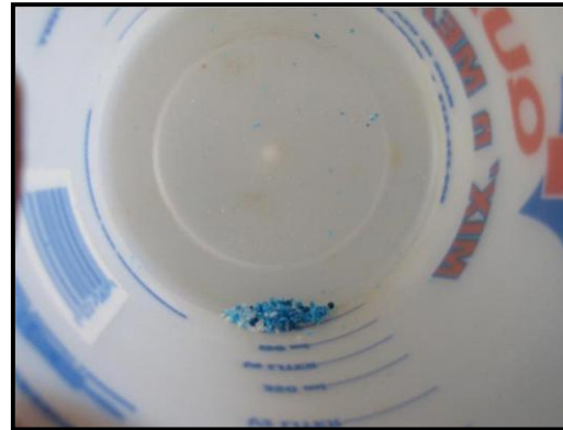
(b) 0.5 grams of Hytac (applicatin rate for both test plots)
