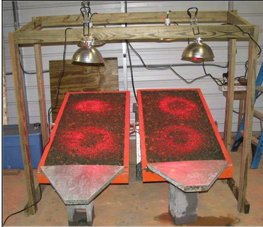
Figure 3.33 Wooden Structure to Suspend Heat Lamps.
