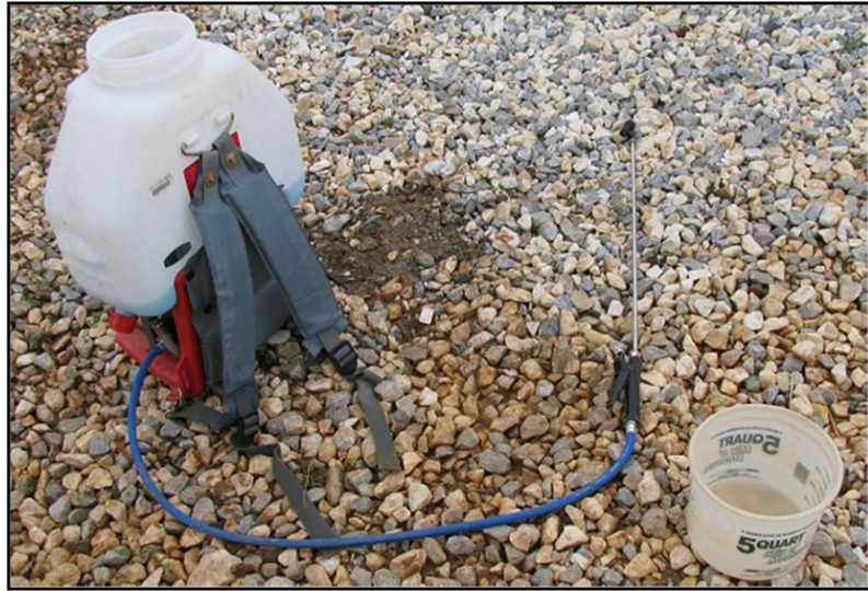
(a) Maruyama MS074 Backpack Sprayer with Tackifier Mixed
