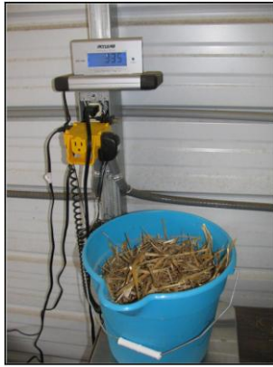
(a) Weighing Straw Prior to App. (4,000 lbs/acre \approx 333 grams/plot)
