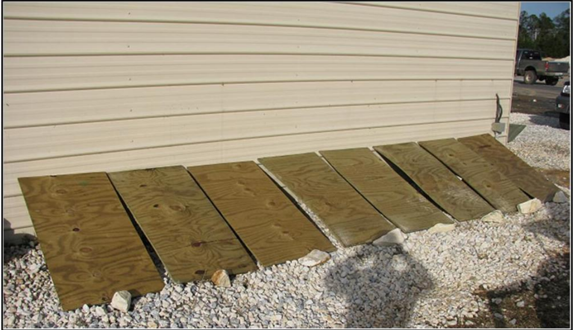
Figure 3.24 3H:1V Test Boards Pre-Application of Hydromulch.
