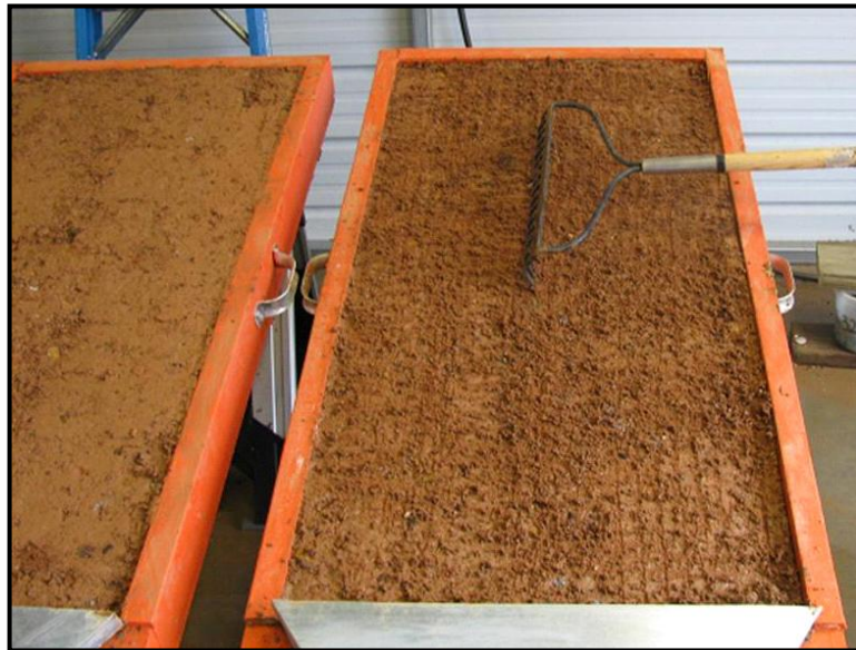
Figure 3.15 Uniform Tilling of Surface Approximately ¼ inch in Depth.
