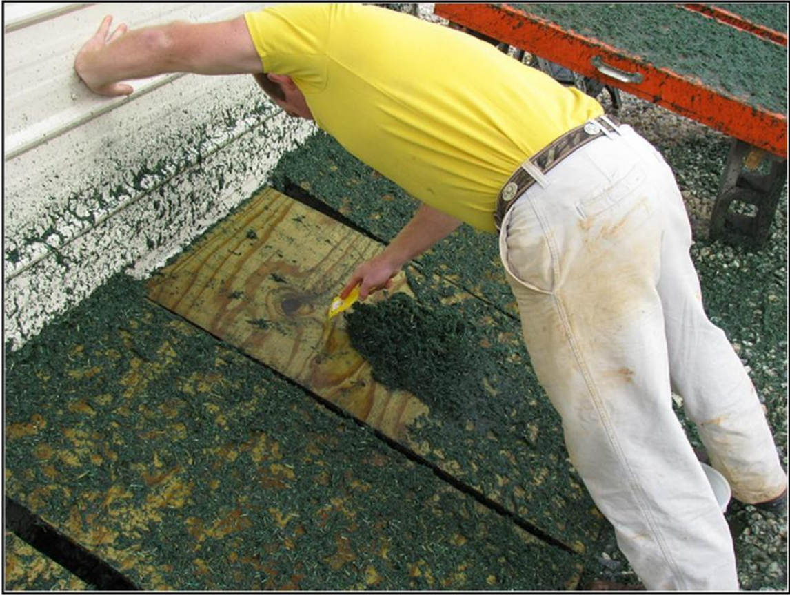
Figure 3.31 Scraping First Two Test Boards.
