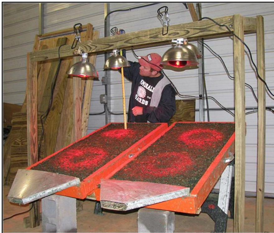
Figure 3.34 Heat Lamps Measured for Accurate Spacing.
