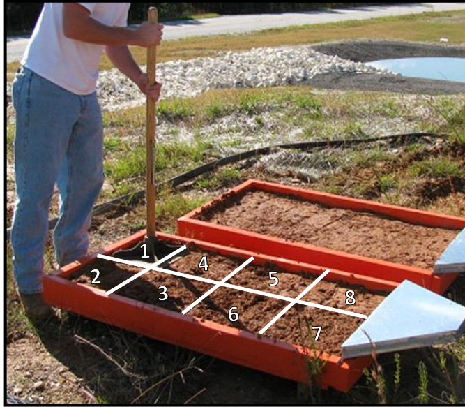
Figure 3.14 8 Sections to Compact Approximately 80 Times.
