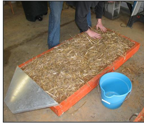
(b) Application of Straw on Test Plots (Minimum 70% cover)
