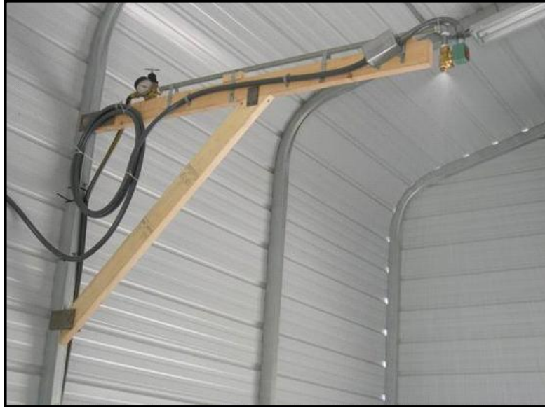
Figure 3.7 Illustration of Rainfall Simulator.
