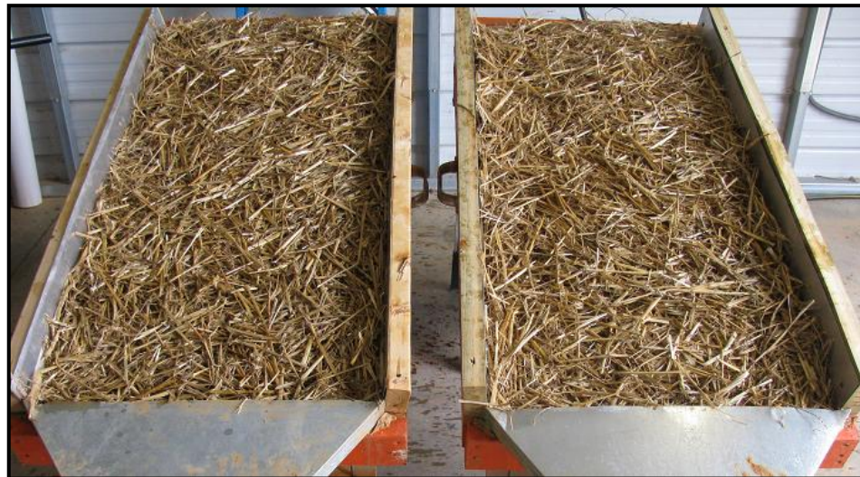
Conventional Straw w/Tackifier, Post-Experimentation.
