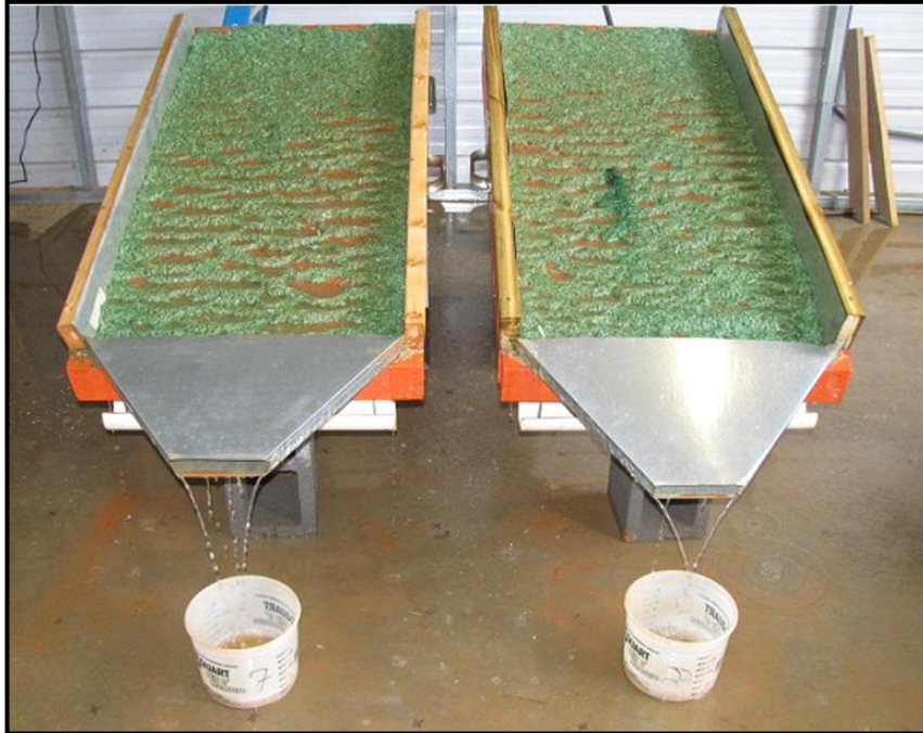
Figure 3.35 Collection of Runoff.
