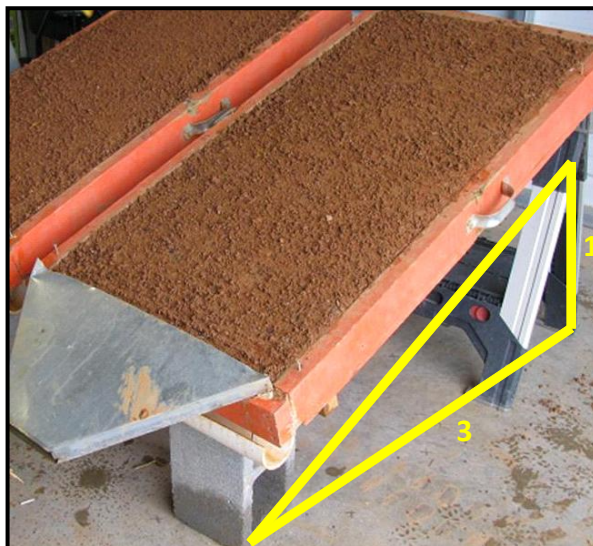
Figure 3.6 3H:1V Slope using Cinderblocks and Saw Horses.
