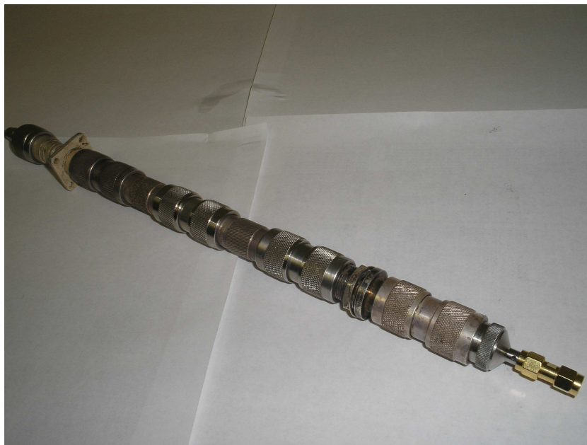
Figure A.4 Short Standard connected at end of coaxial connector plumbing
