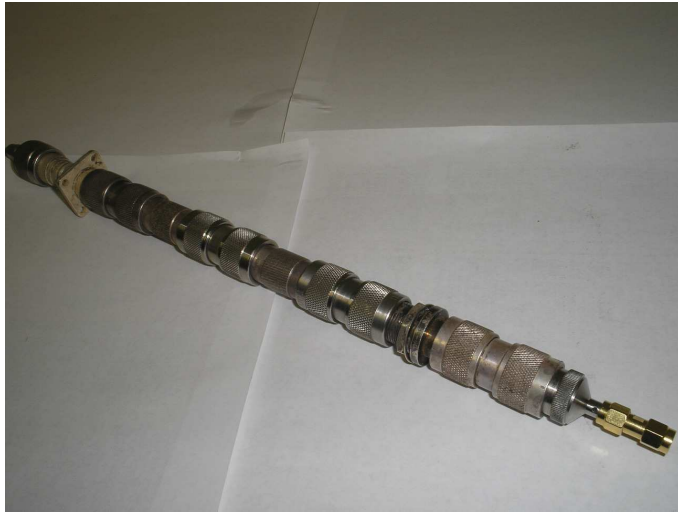
Figure A.8 Load Standard connected at end of coaxial connector plumbing
