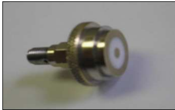
Figure 1.5 Coaxial Probe made from RF connector
