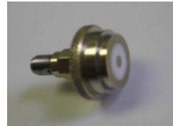
Figure 4.2 RF coaxial test probe made from N_{\text{Male}} to SMA_{\text{Male}} RF coaxial adapter
