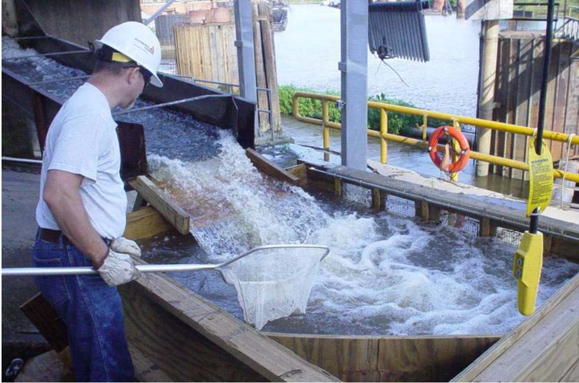
Figure 6. Outflow flume and collection basket at the cooling water intake structure for steam generation Units 1 through 3 during the Plant Barry Survival Study in 2007.
