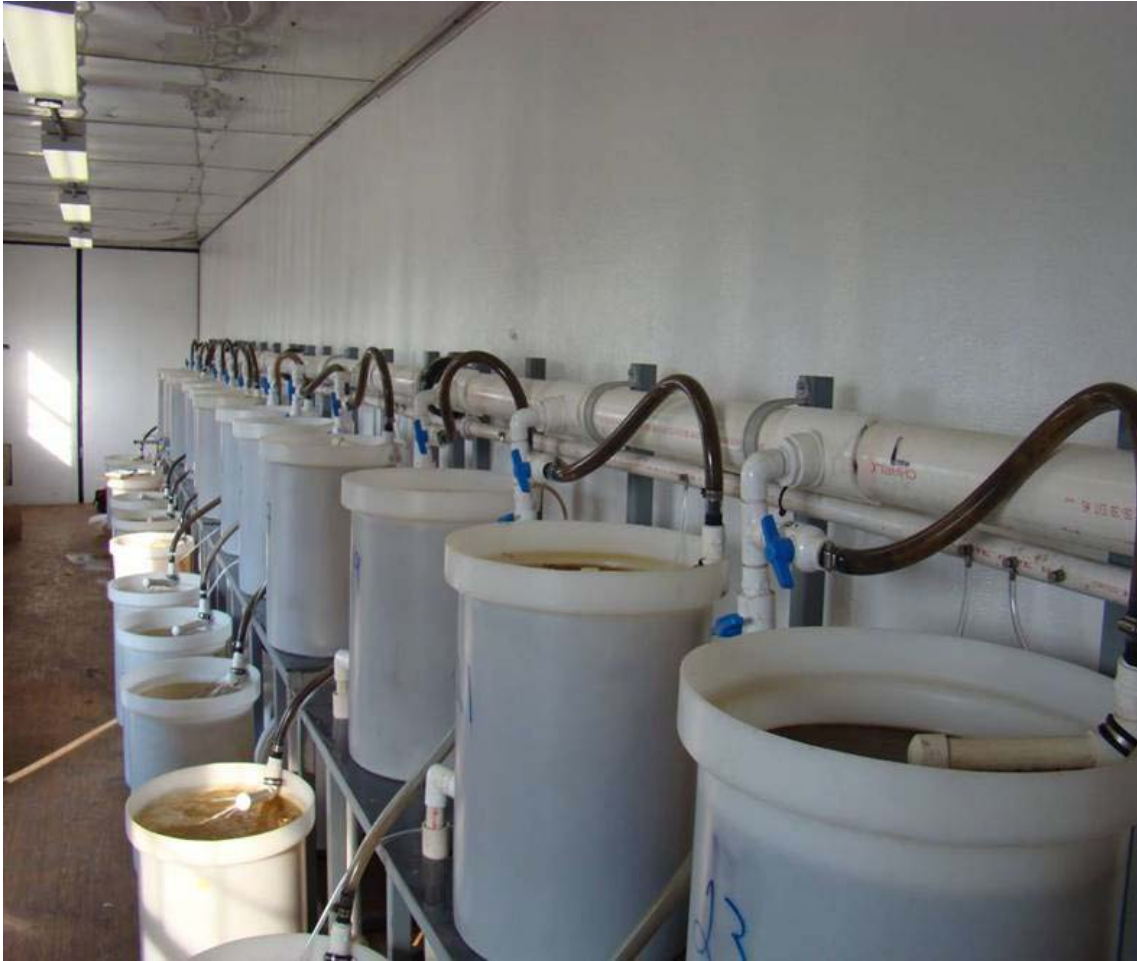
Figure 7. Aquaria system and temperature controlled trailer used in the Survival Study at Plant Barry, Alabama in 2007.
