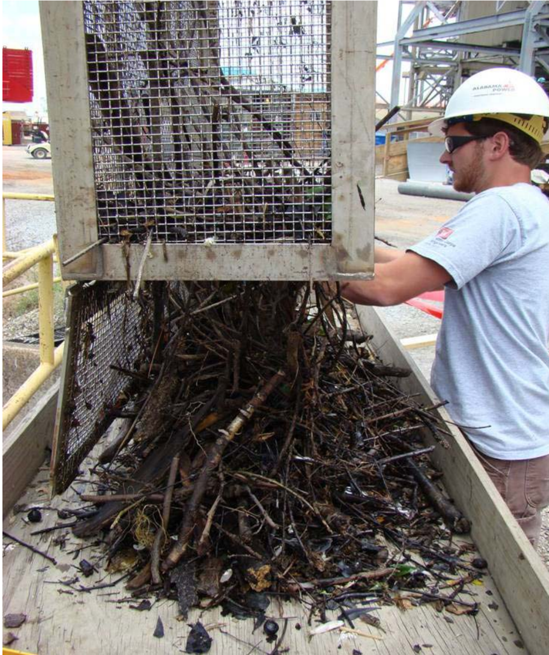
Figure 5. Sample collection from the outflow flume at the cooling water intake structure steam generation Units 4 and 5 during the Screen Rotation Study at Plant Barry, Alabama in 2007.
