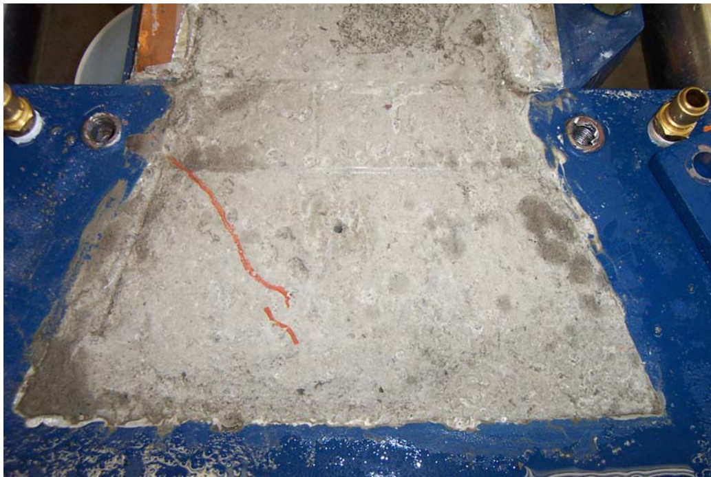
Figure 4-6: Cracking in the crosshead
