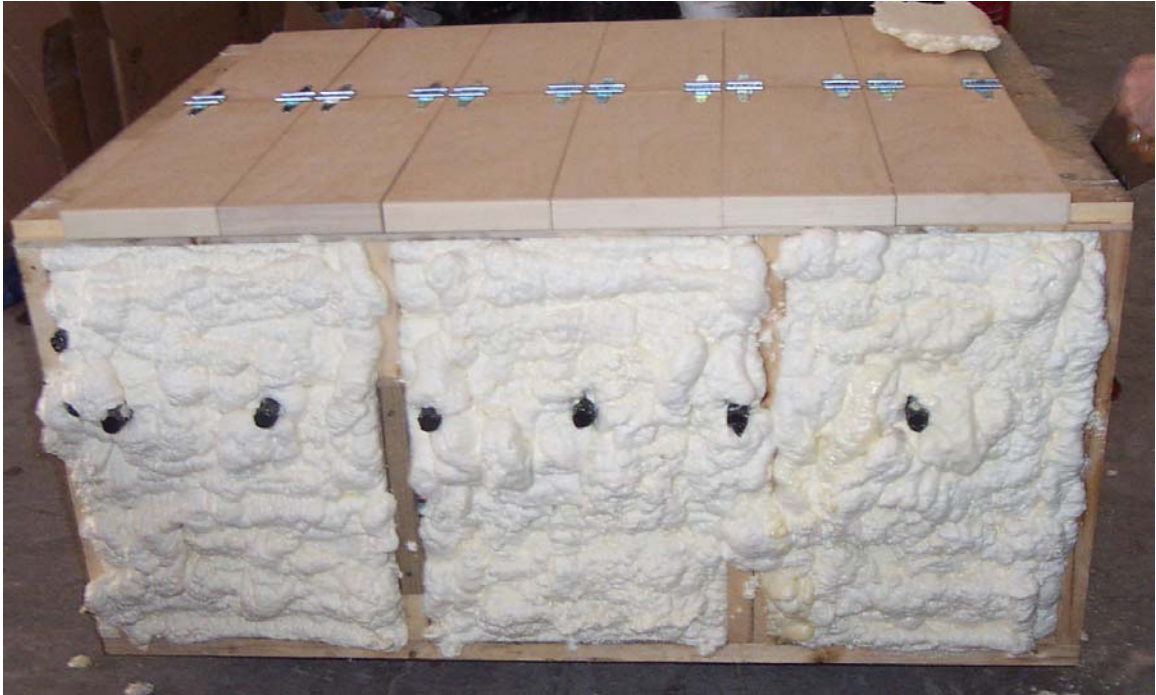
Figure D-7: Insulated match-curing box
