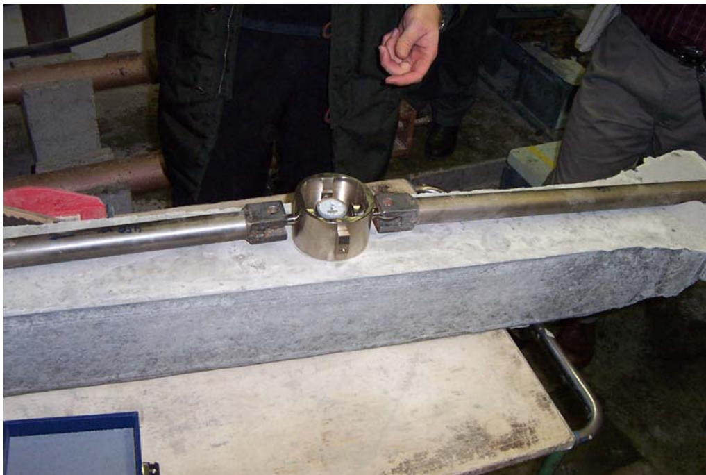
Figure A-9: Load cell and calibration linkage
