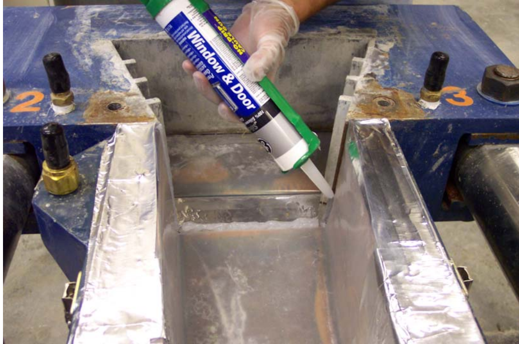
Figure C-11: Caulking joints with silicone sealant
