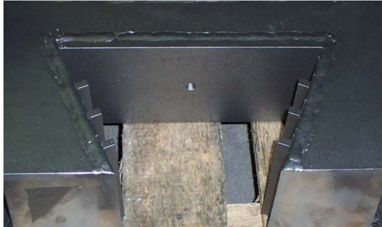
Figure 4-4: Cracking frame crosshead under construction
