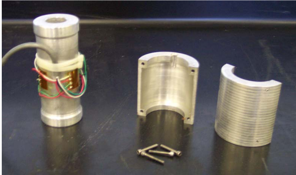
Figure C-2: Compression load cell
