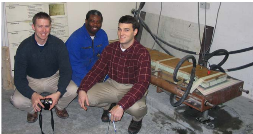
Figure 3-3: The rigid cracking frame during operation in Munich
