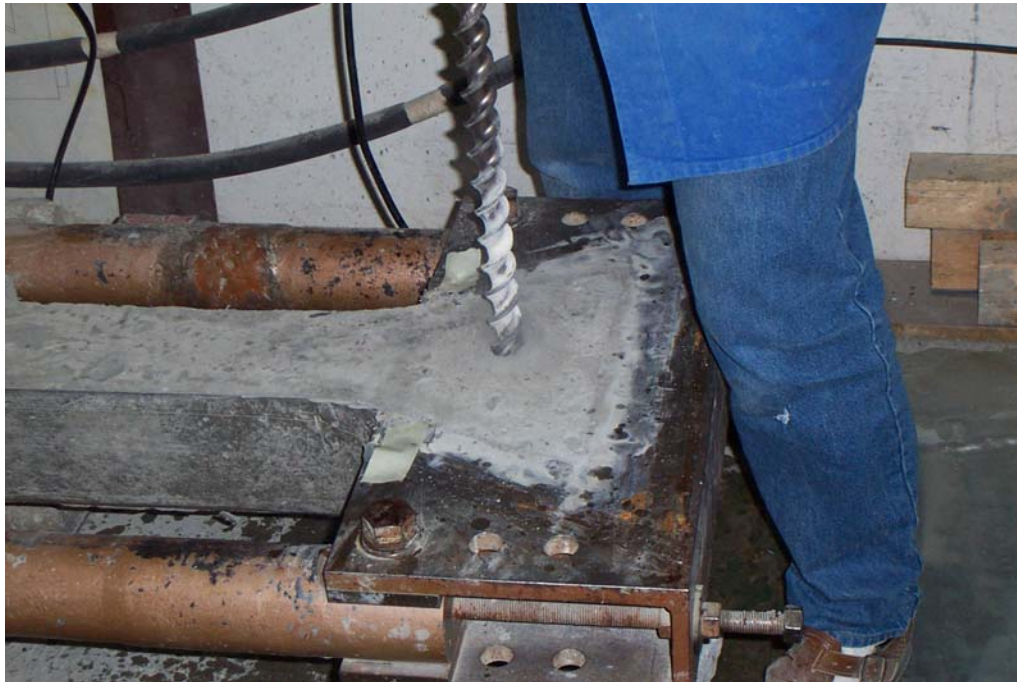
Figure A-11: Drilling a hole to remove the specimen from the crosshead
