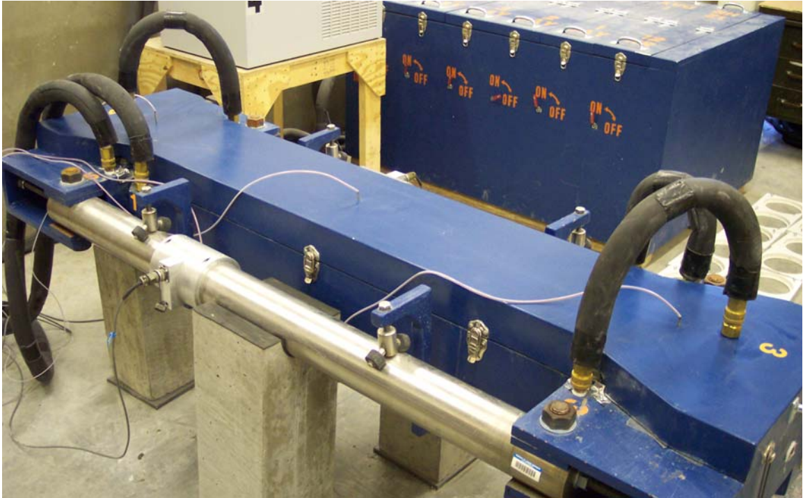
Figure B-29: Formwork installed in the rigid cracking frame
