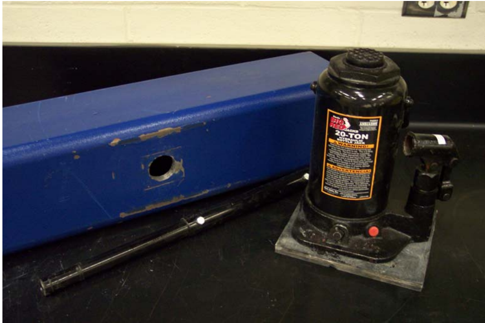
Figure C-26: 20-ton bottle jack and a steel rig
