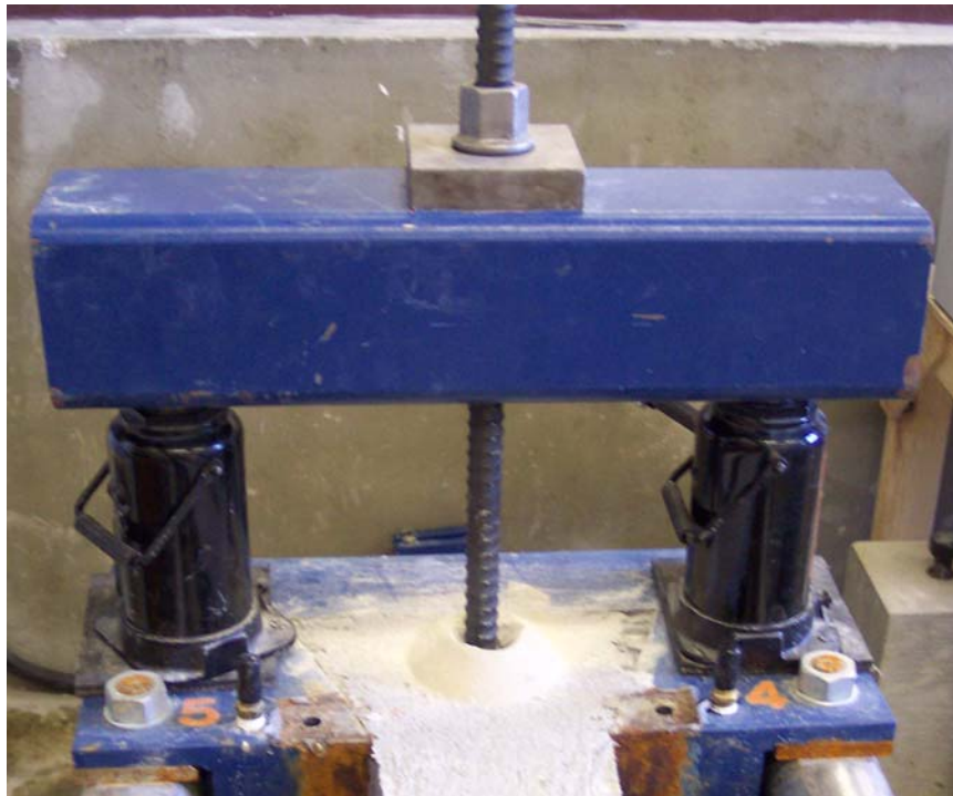
Figure 5-9: Specimen removal from the cracking frame
