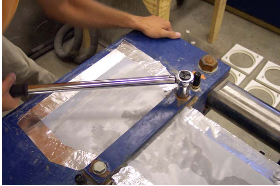
Figure C-17: Securing the crosshead braces with a torque wrench
