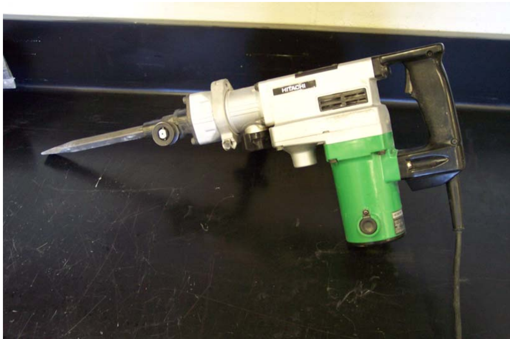
Figure C-29: Jackhammer and chisel
