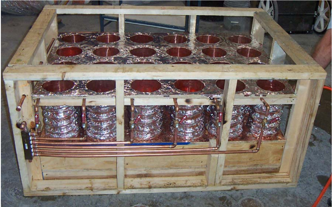
Figure D-5: Match-curing box ready for insulation
