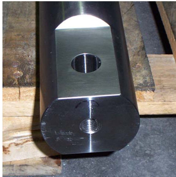
Figure 4-3: Invar side bar under construction
