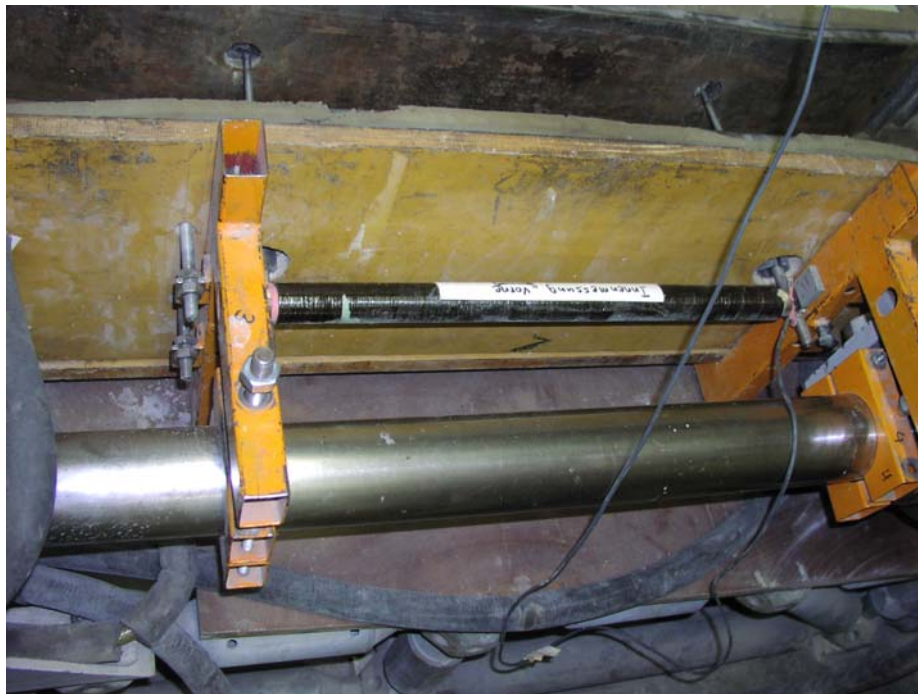
Figure 3-11: Side view of the length measurement device used at TUM
