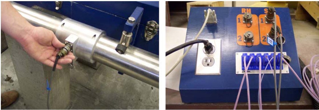
Figure C-20: Connecting strain gauges and instrumentation
