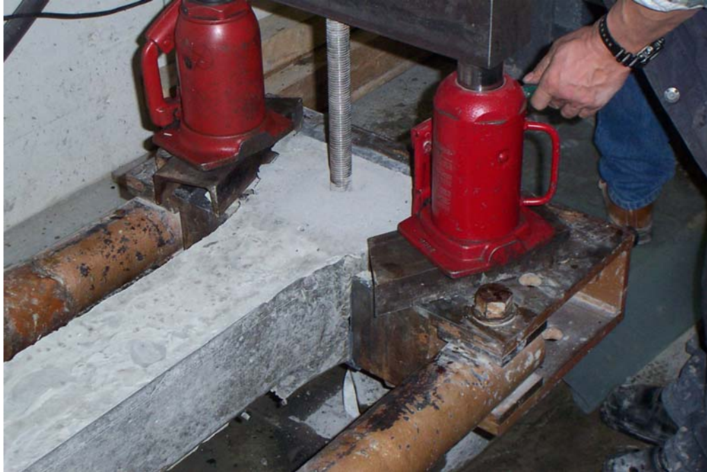
Figure A-12: Jacking the specimen out of the crosshead
