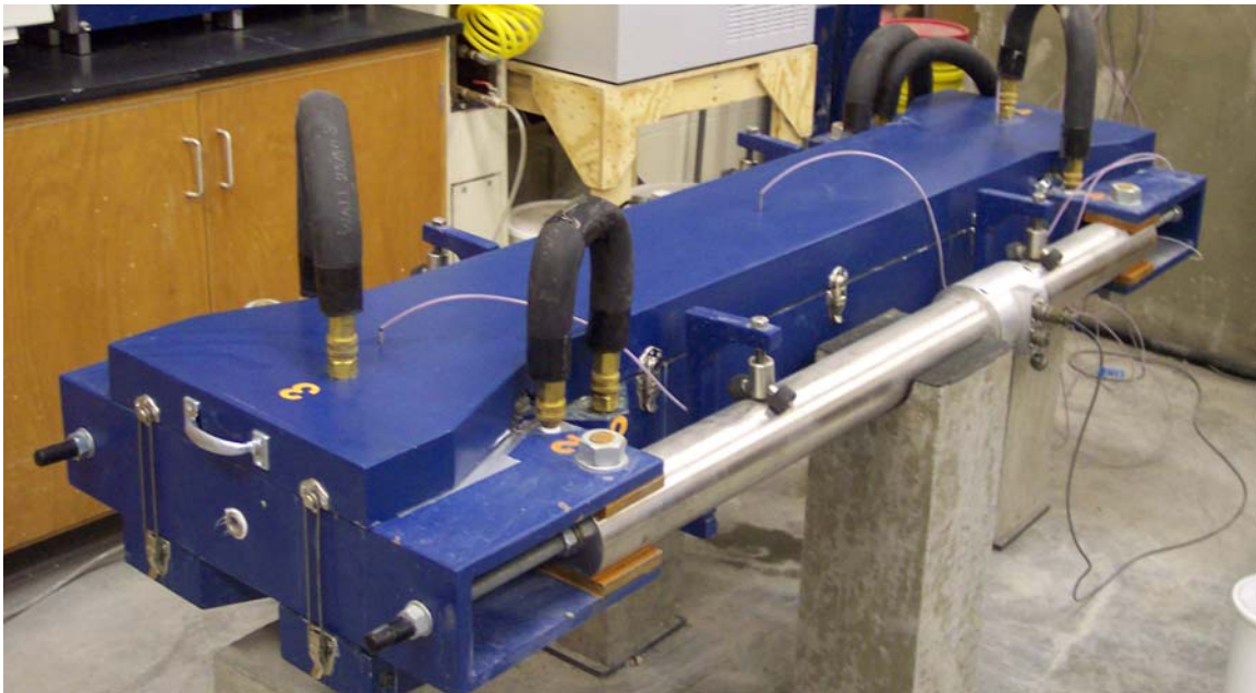
Figure C-5: Rigid cracking frame and thermally insulated formwork
