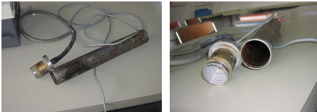
Figure 3-13: In-place stress meter developed at TUM
