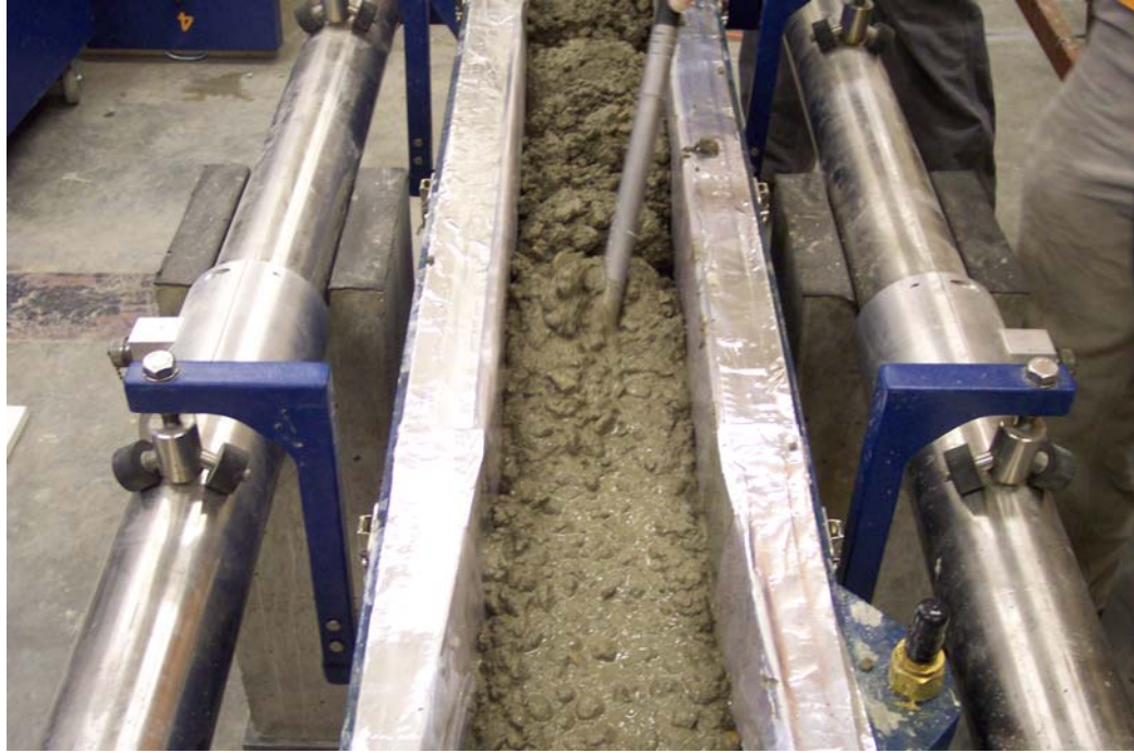
Figure C-13: Consolidating fresh concrete with a vibrator
