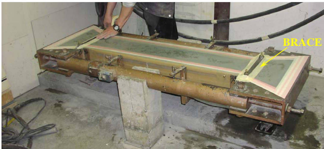
Figure 3-4: Sealing the concrete specimen in the frame
