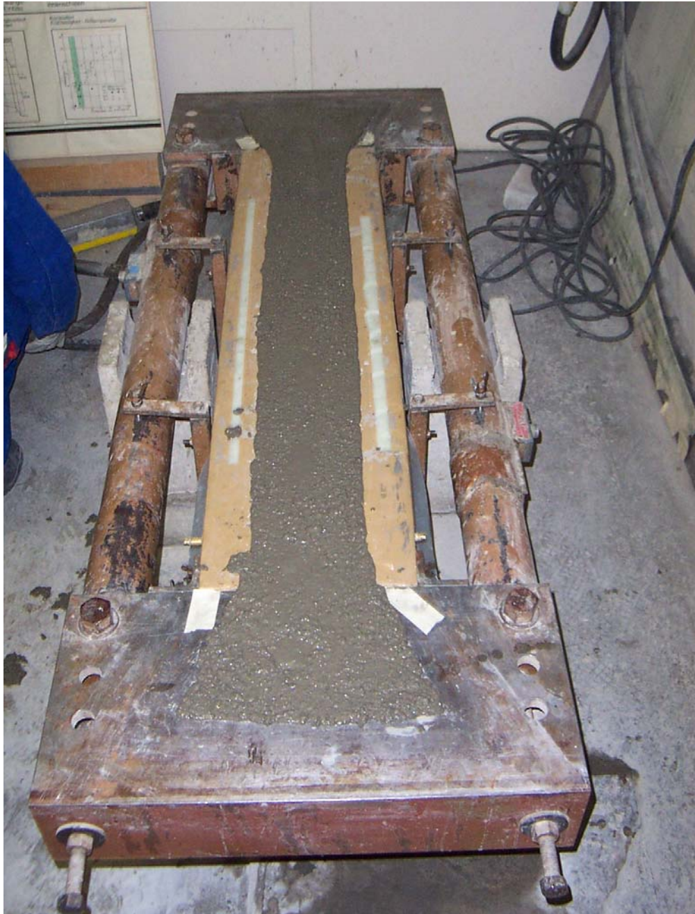
Figure A-7: Rigid cracking frame
