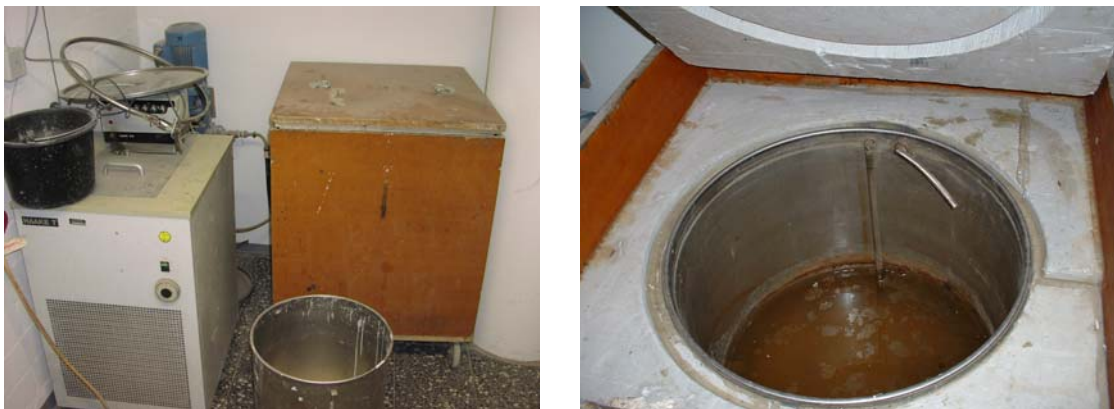
Figure 3-14: Adiabatic calorimeter used at TUM
