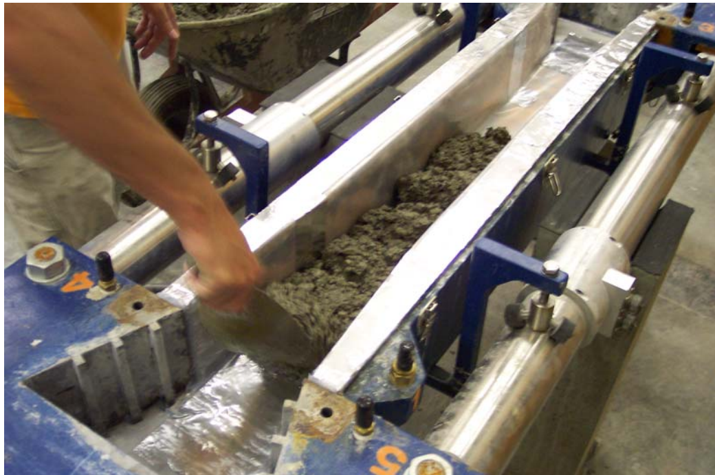
Figure C-12: Placing concrete in the formwork
