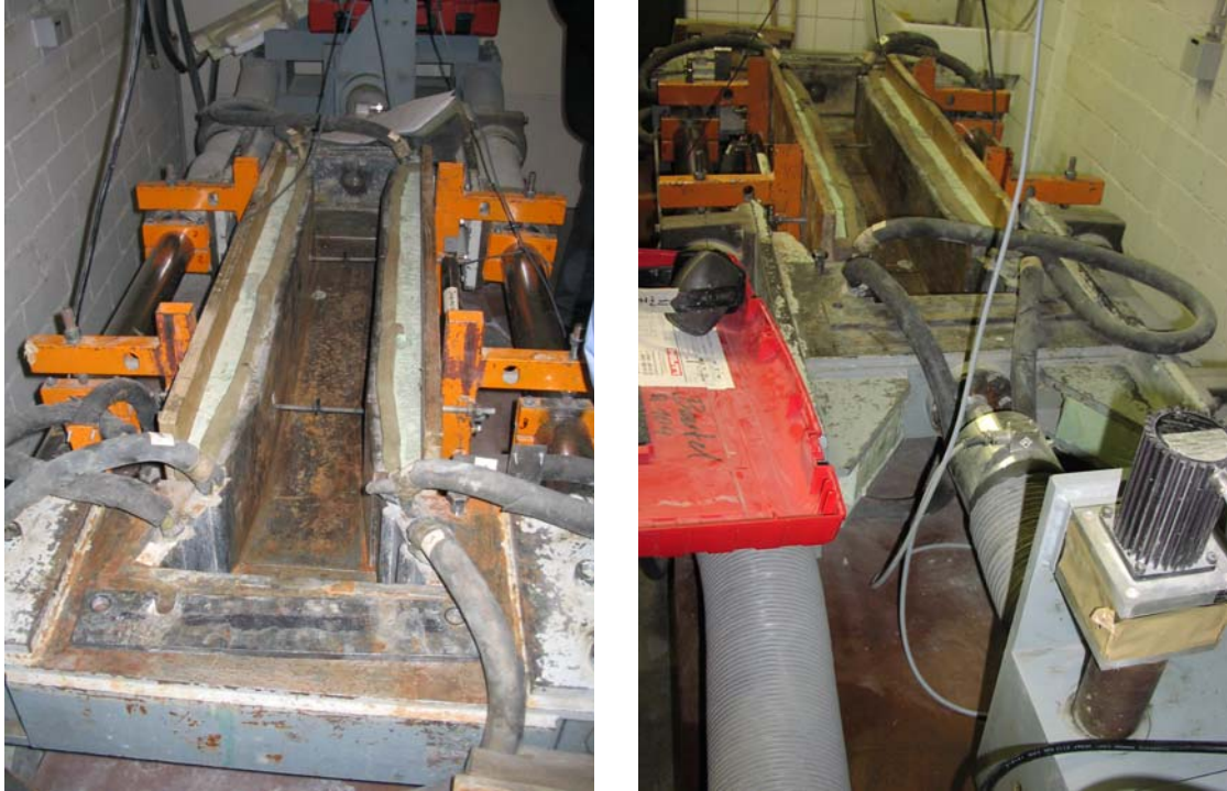
Figure 3-9: Temperature-stress testing machine at TUM
