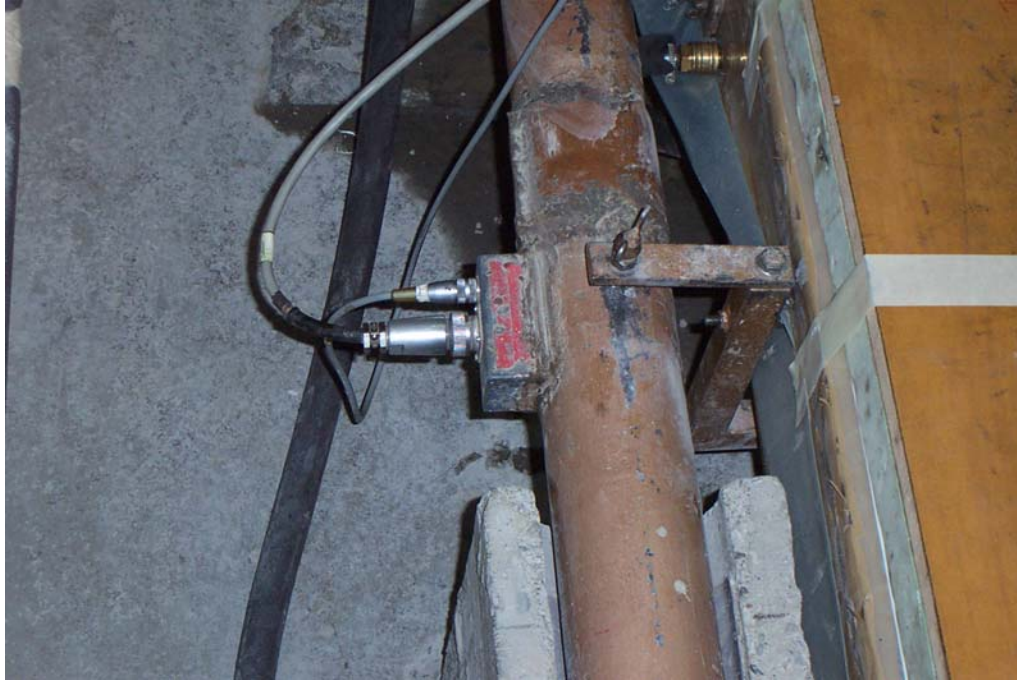
Figure A-8: Strain gauges mounted on the Invar side bars
