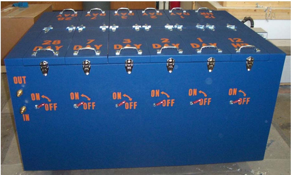
Figure D-8: Match-curing box ready for testing
