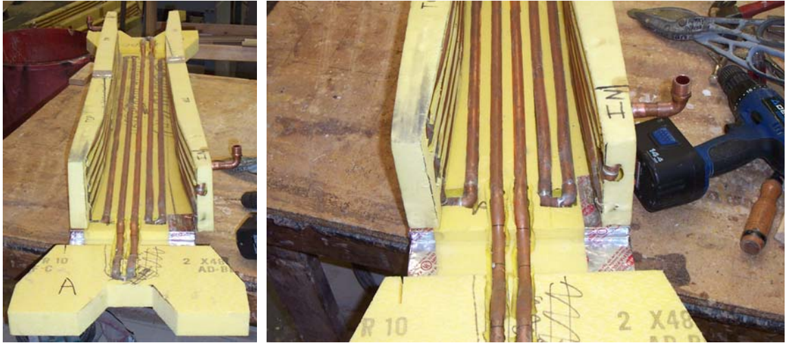
Figure B-25: Rigid insulation with copper tubing
