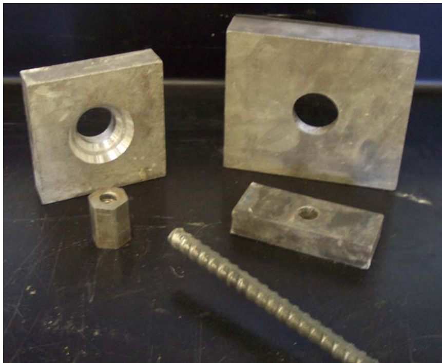
Figure C-3: 5/8-in. DYWIDAG bar with anchor plates and nuts
