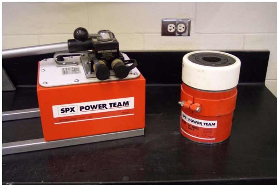
Figure C-1: Hydraulic jack and pump
