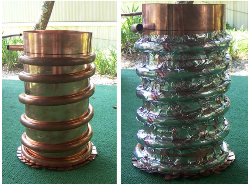
Figure D-3: Copper sleeves wrapped with copper tubing and foil tape
