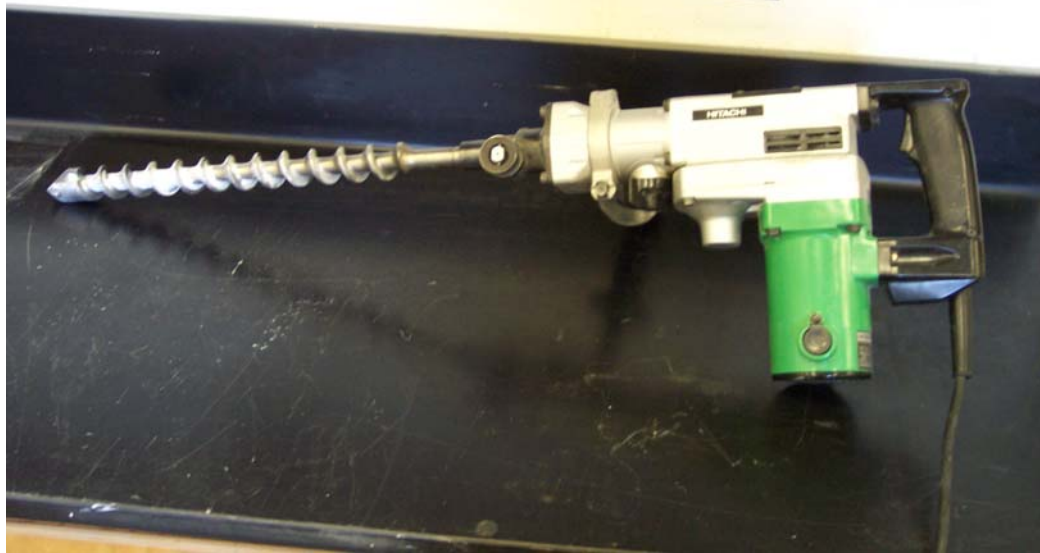
Figure C-28: Concrete drill with masonry bit
