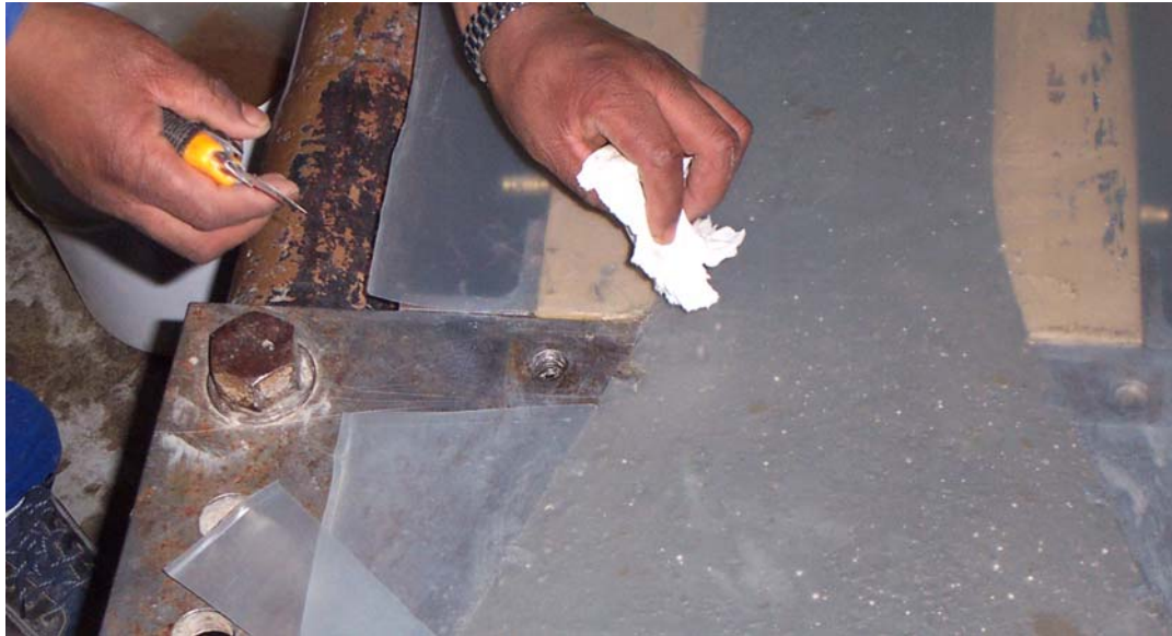
Figure A-4: Sealing the concrete specimen with plastic
