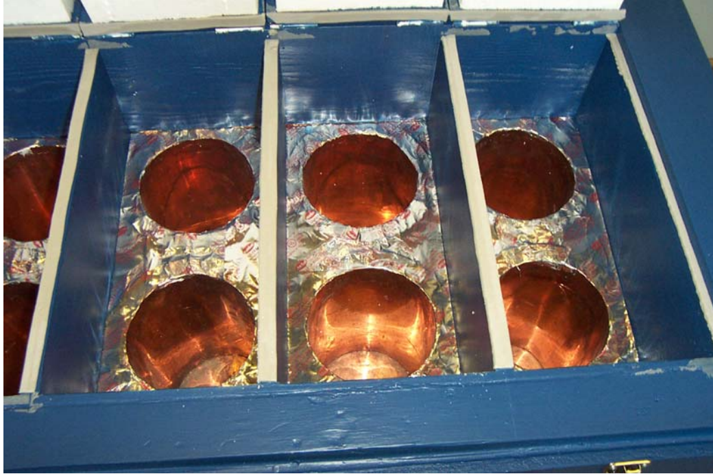
Figure D-9: Interior of match-curing box without cylinders
