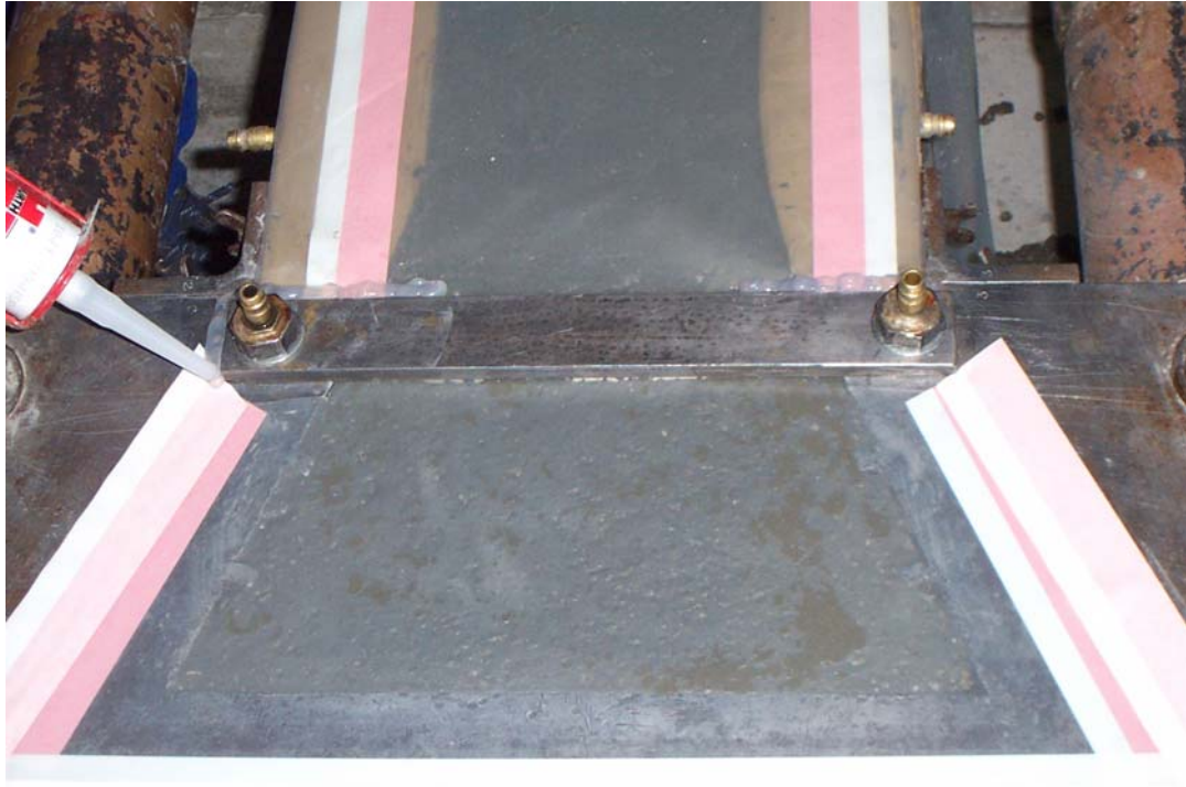
Figure A-6: Sealing the crosshead braces with silicone
