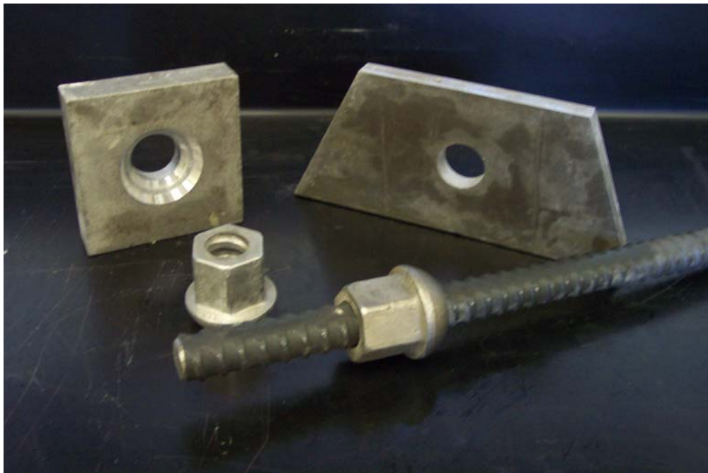
Figure C-27: 1-in. DYWIDAG bar with anchor plates and nuts
