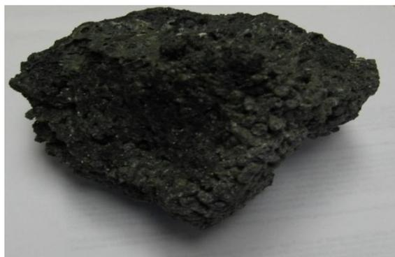
Figure 3.8 Ash agglomeration in the grate of gasifier after the gasification of poultry litter
