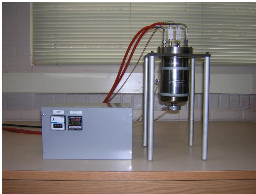
Figure 3.2. Photo of the oil degradation vessel.
