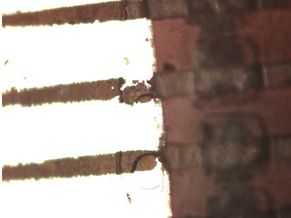
Figure 4.7: Interconnect Breakage Due to Delamination Event
