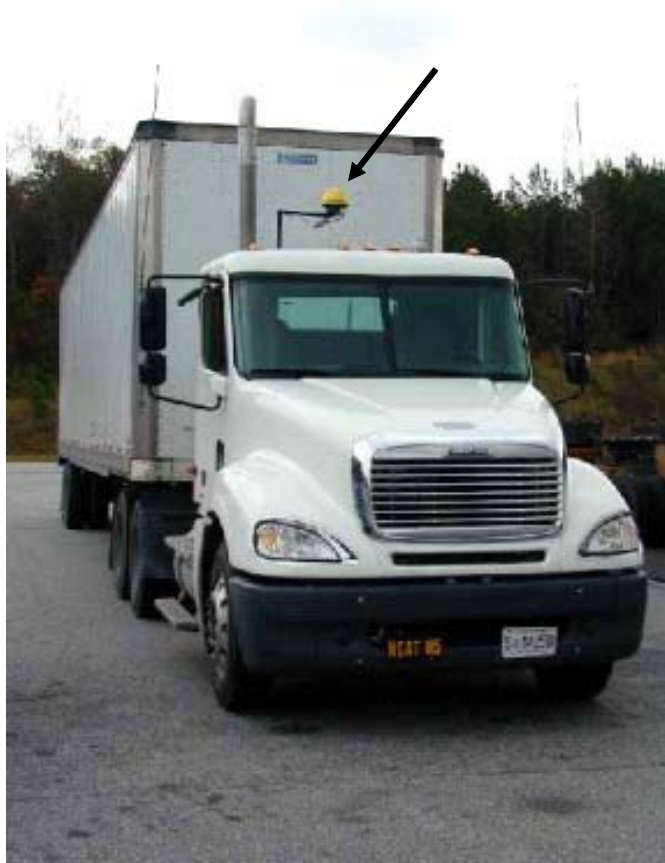
Figure B.3. NCAT Test Truck with Starfire GPS Unit Indicated
