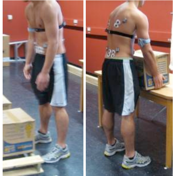
Figure 23: Subject wearing Noraxon TeleMyo™ 2400T Direct Transmission System (electrodes for the left and right bicep femoris muscles not shown)
