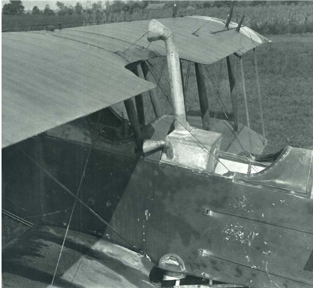
View of air suction hopper installed in Lieutenant McNeil's Hispano-powered Curtiss JN-6H. August 31, 1922. Photograph courtesy Louisiana Department of Agriculture and Forestry.
