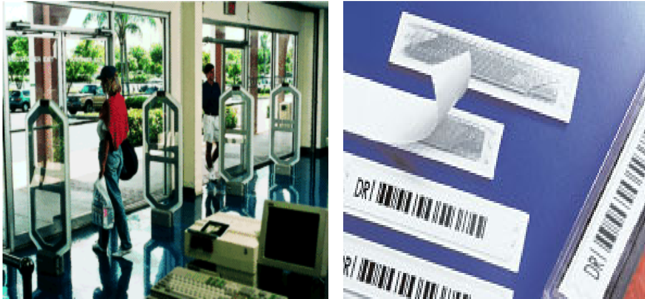
Figure 2.7 Magnetostriuctive strips used on valued goods for theft protection
