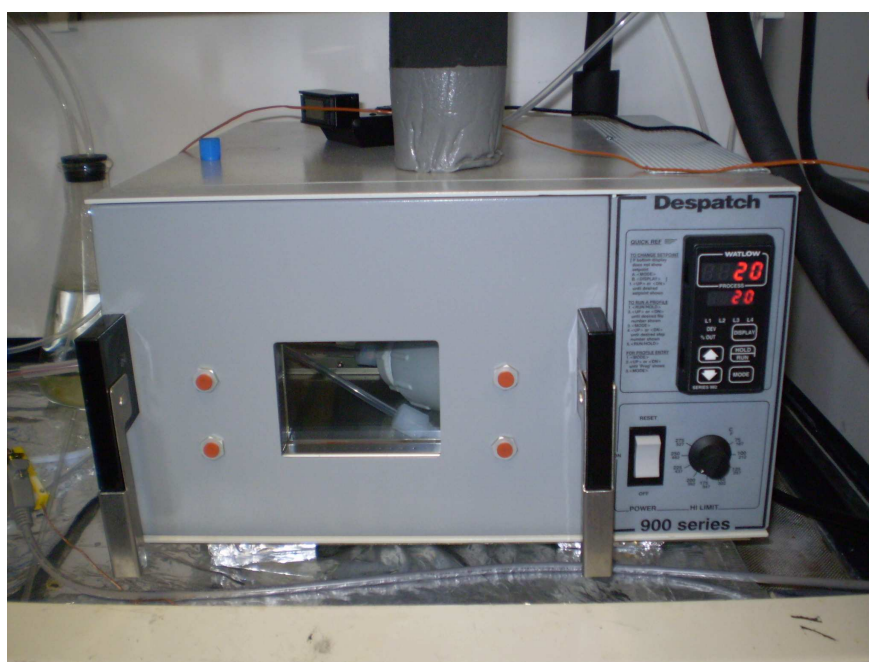
(b) Despatch 900 temperature chamber
