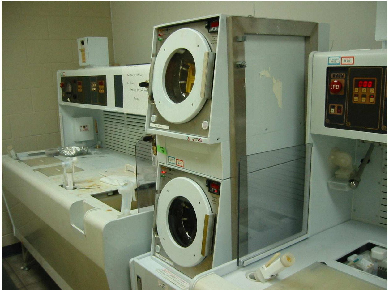
Figure 4.3: The spin dry washers at AMSTC rinses wafers with clean deionized water until the wash water has a resistance greater than a threshold value. It then automatically purges the wash chamber with nitrogen gas and spins the wafers until they are dry.
