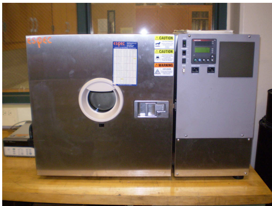
(a) Espec ECT temperature chamber
