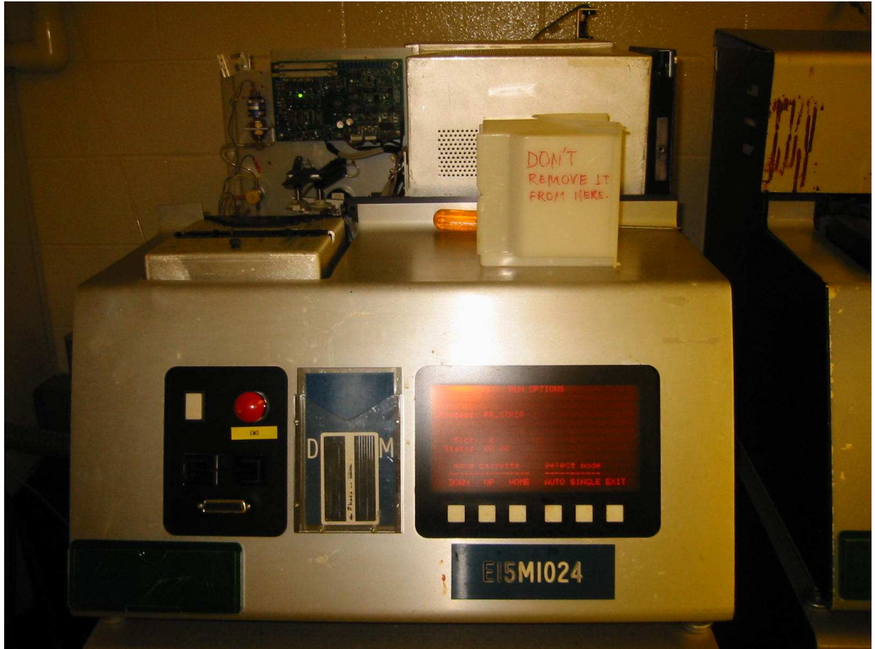
Figure 4.6: The matrix plasma asher at AMSTC is a dry etch device used for stripping of residual photoresist to improve electrode deposition.
