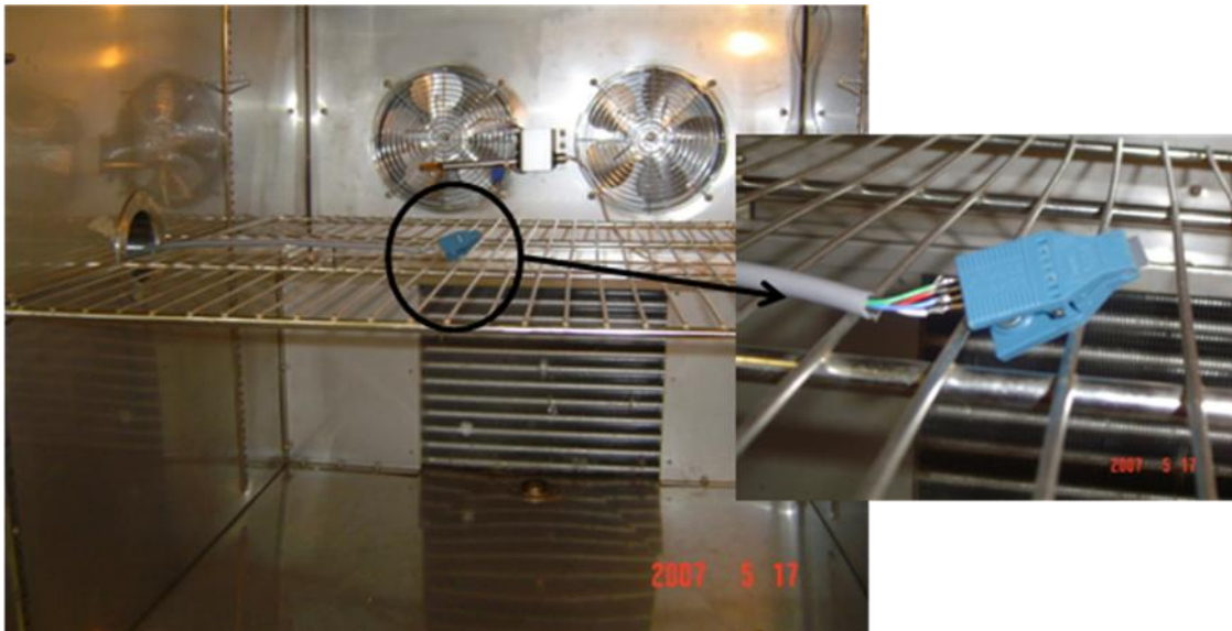
Figure 6-5 Photograph of the interior of the environmental chamber and Pomona clip for resistivity testing.
