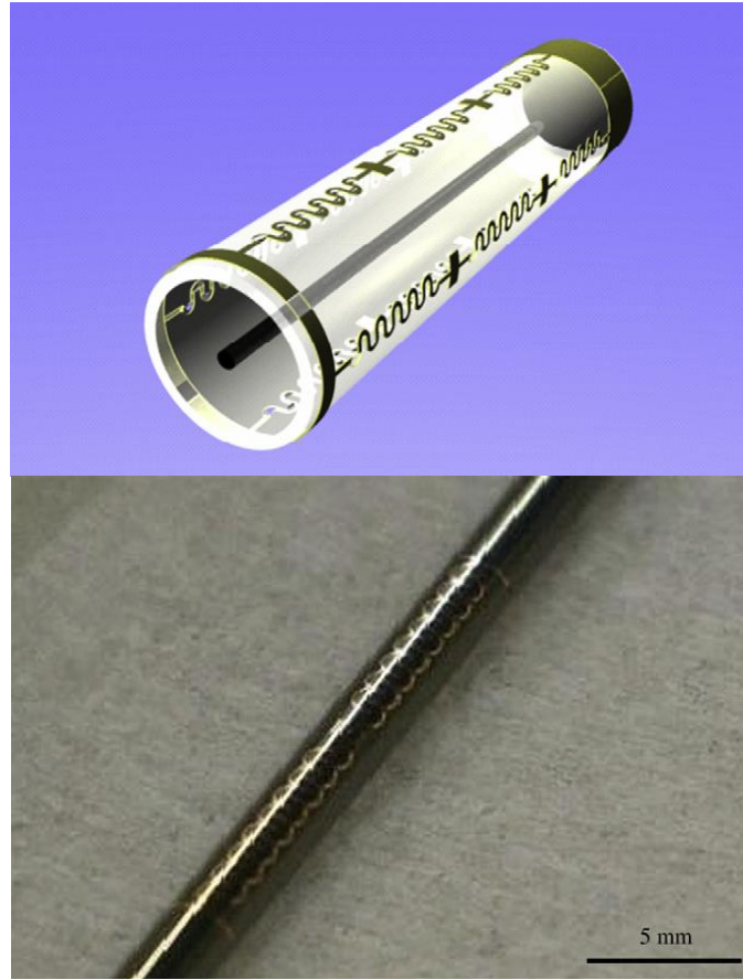
Figure 3-5 Schematic and photograph of zigzag shaped spring [9]
