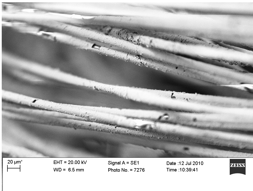
Figure 4-11. SEM image of Kevlar fibers first coated in the Ni electroless bath, then exposed to ultrasound in H 2 O and electroplated with Au via the thiosulfate procedure.
