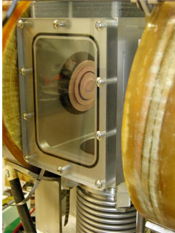
Figure 3-4: A photograph of the custom six-way vacuum box mounted on ALEXIS. Note the two magnets on either side of the box, the bellow that leads to the diffusion pump (near the bottom), and one of the “4-ring” electrode assemblies used to modify the electric field in the ALEXIS plasma.
