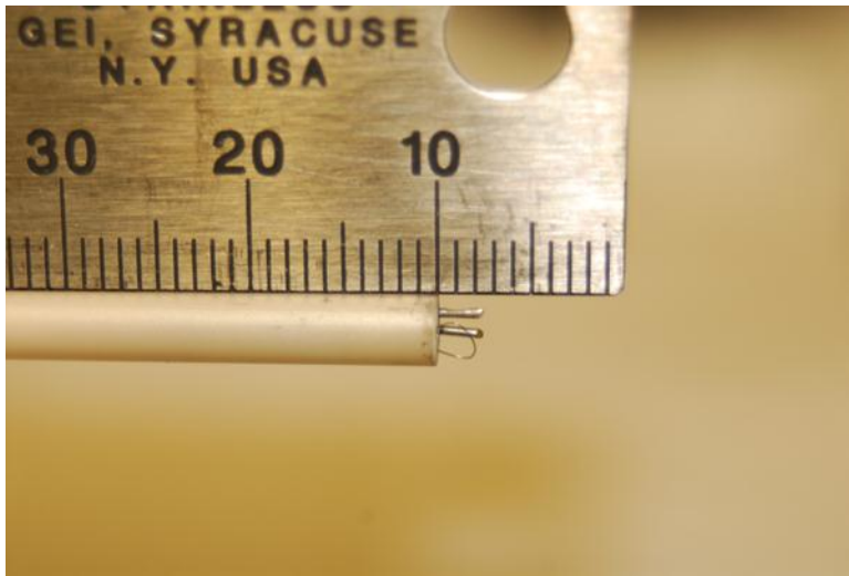
Figure 3-7: Combination emissive probe (thin wire loop) and double Langmuir probe (straight wires). The ruler gives the scale in millimeters.
