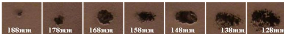
Figure 2.5: Photographic images of the ablation pits formed as a function of the distance between the RDX spot and the focusing lens, as indicated on the pictures. The area of each picture is 1.85mm by 1.60mm.
