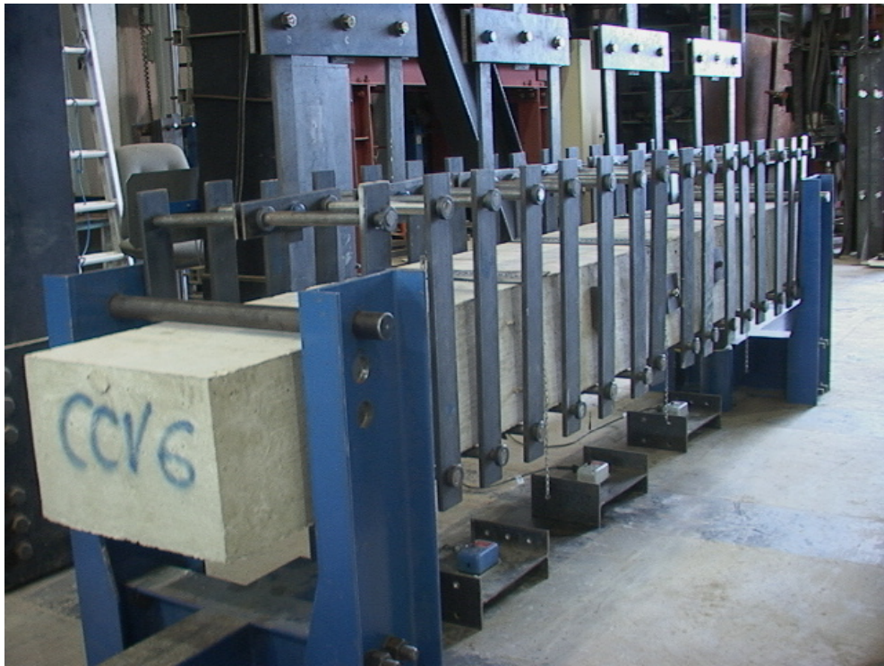
Fig. 3.2. University of Missouri loading-tree apparatus setup and reinforced concrete beam validation sample
