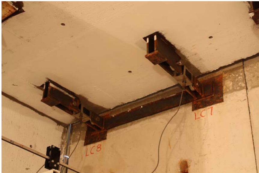
Figure 4.6. Load cells recording reaction force for single span specimens
