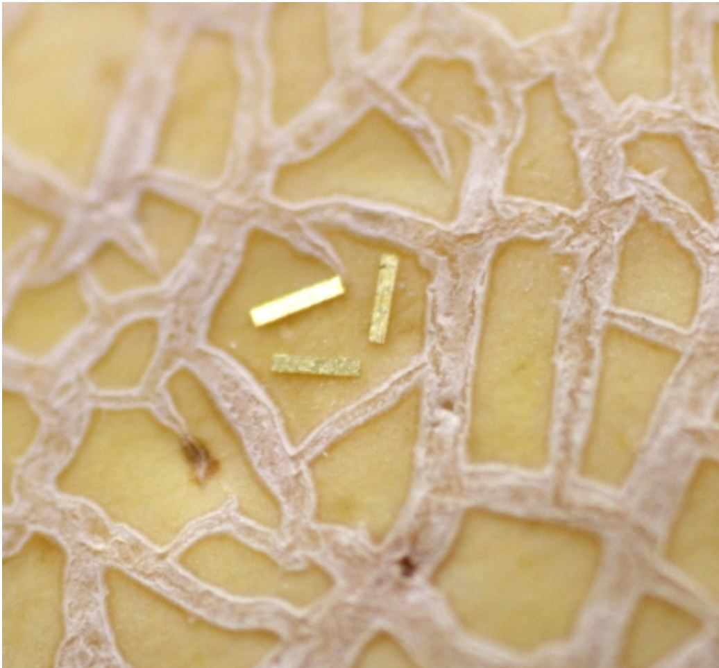
Figure 9.1: Three magnetoelastic sensors for simultaneously detecting S. typhimurium directly on the cantaloupe surface. Sensor Dimensions: 2000 \times 400 \times 15 \mu\text{m} .
