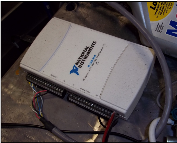
Figure 4-6: National Instruments USB-6210 data acquisition unit
