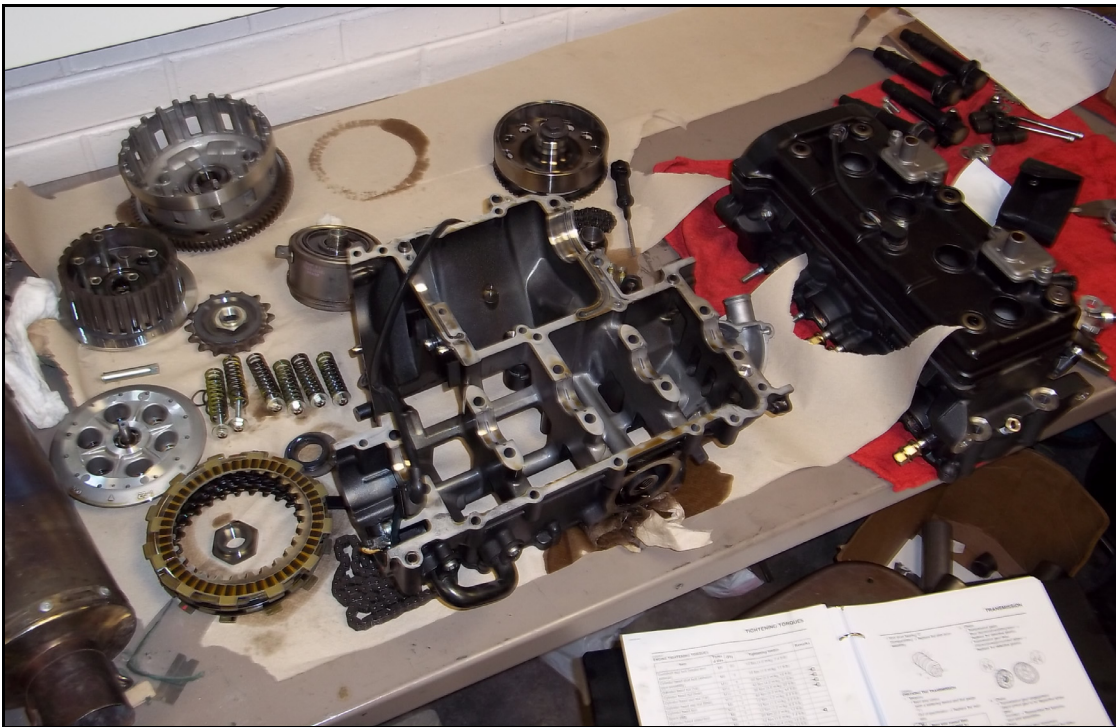
Figure 5-6: Disassembled lower crankcase, cylinder head, & clutch components
