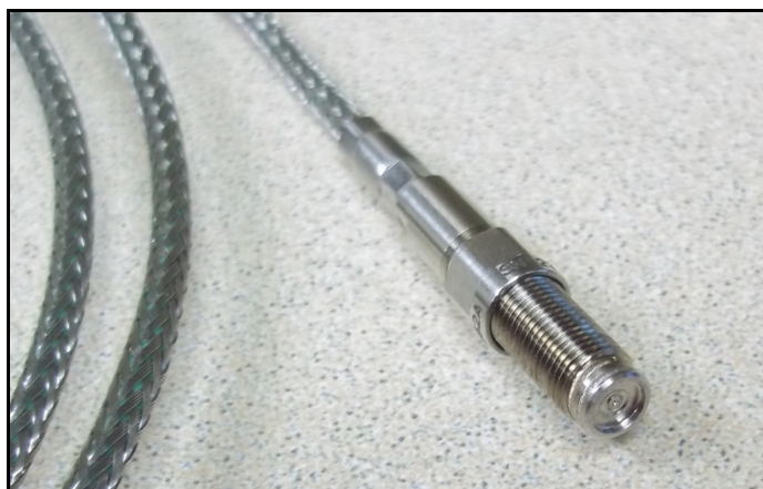
Figure 4-1: Kistler 5001 charge amplifier and 6052A high temperature pressure sensor
