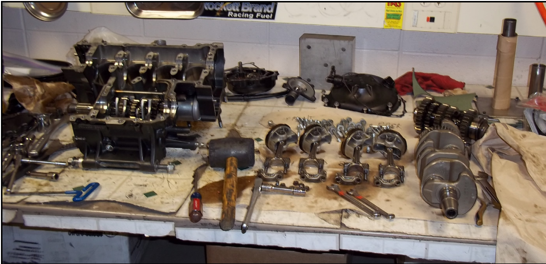
Figure 5-5: Disassembled upper crankcase, transmission, & power cylinder components
