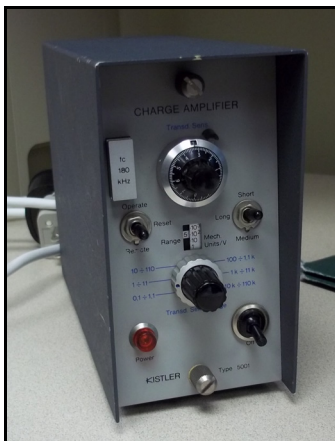
Figure 4-1: Kistler 5001 charge amplifier and 6052A high temperature pressure sensor
