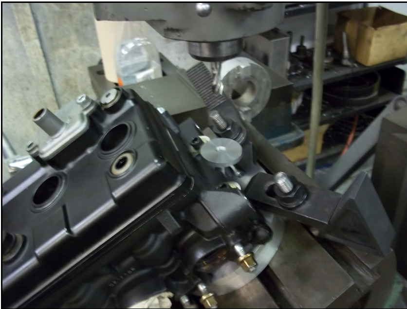
Figure 5-1: Tilt table and cylinder head jig adjustment on mill
