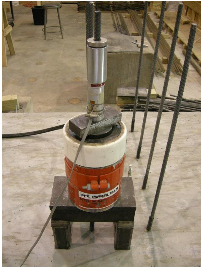
Figure 3.14: Chuck, load cell, hydraulic jack, and 8-inch-tall reaction chair
