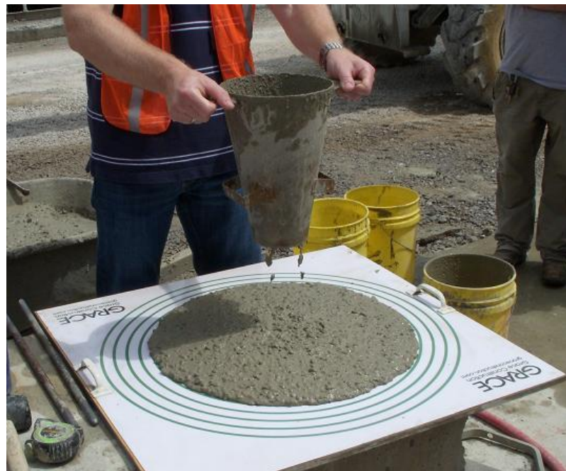
Figure 3.20: Performance of slump flow test
