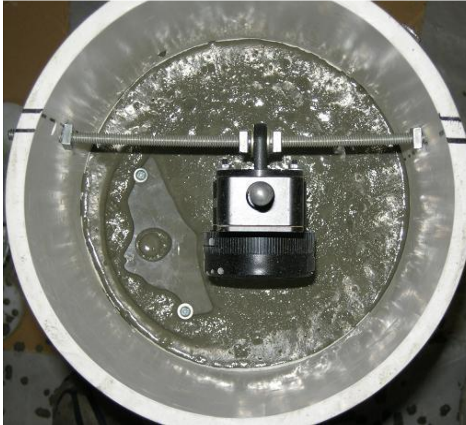
Figure 4.1: Acrylic settlement plate sinking unevenly during the surface settlement testing of SCC-1A
