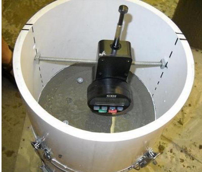
Figure 1.4: Settlement of a clear acrylic plate into SCC during the surface settlement test
