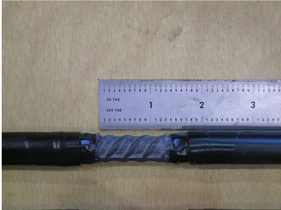
Figure 3.12: 1.25 in. bonded region of a No. 4 rebar ready for casting into concrete
