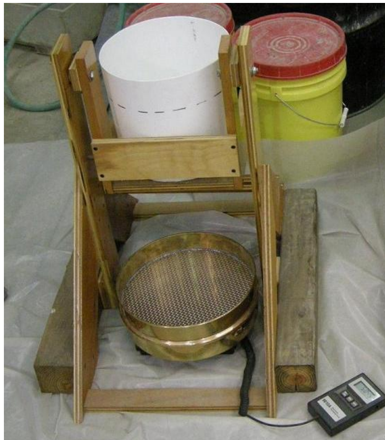
Figure 3.22: Sieve stability test with pouring apparatus, sieve, and scale
