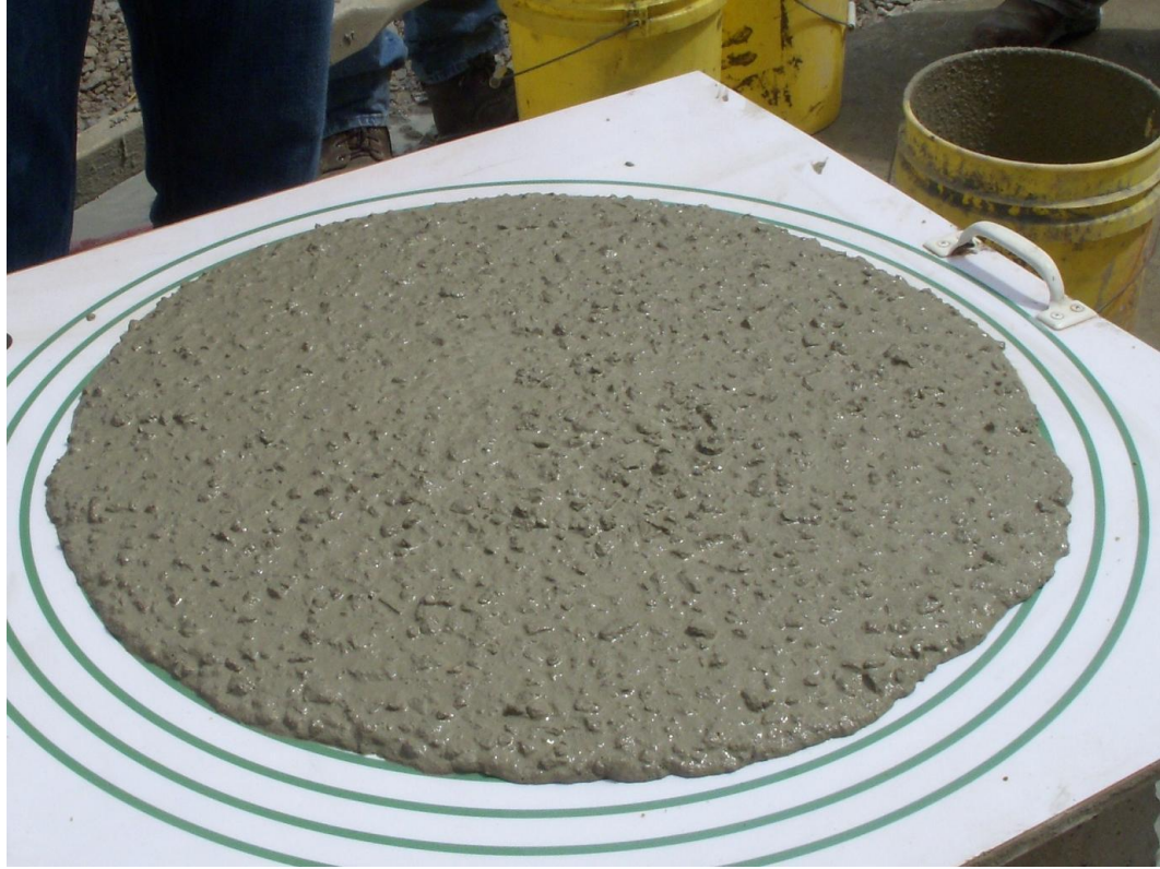
Figure 1.3: Patty of fresh SCC as it is visually assessed during the VSI test
