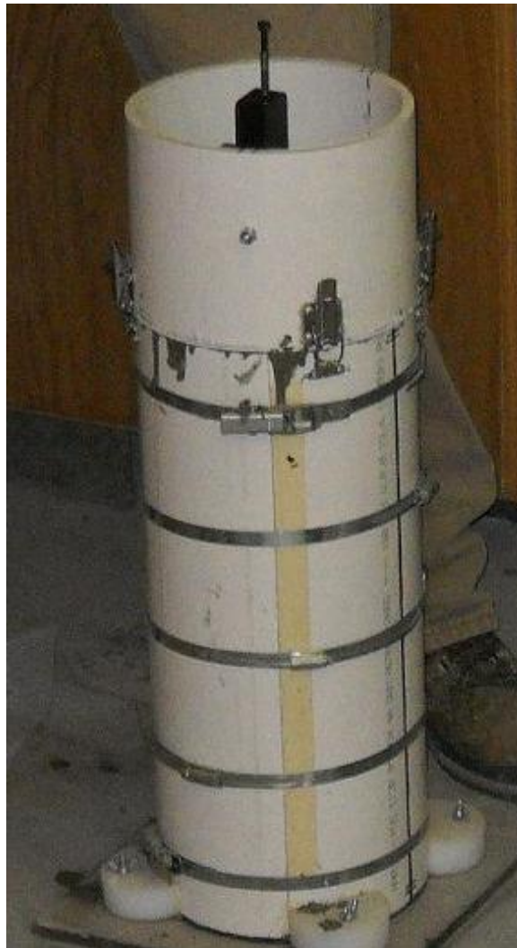
Figure 3.23: A) Digital dial indicator used to measure settlement of an acrylic plate, and B) four-piece constructed surface settlement test apparatus
