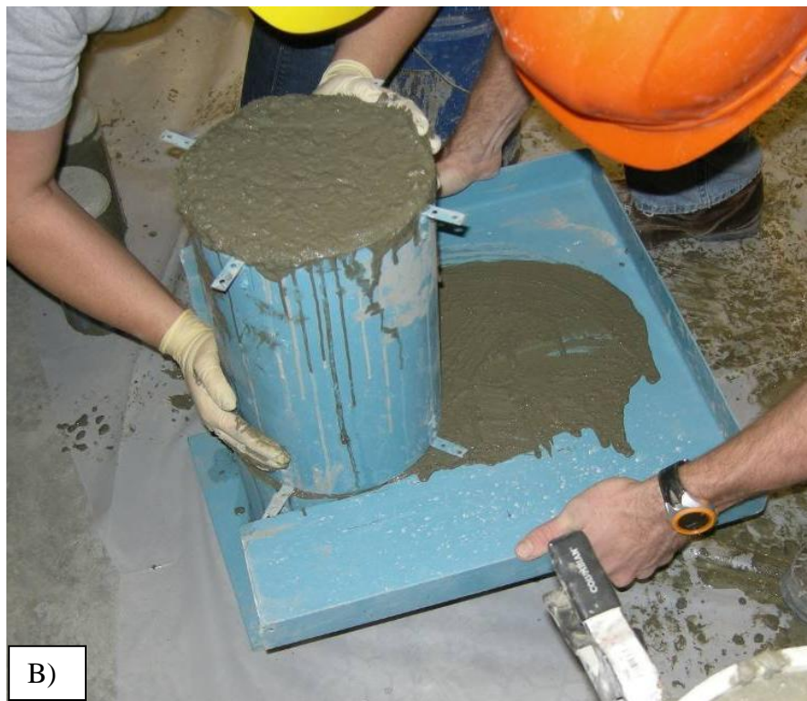
Figure 3.21: A) Two column segregation molds used during simultaneous testing and B) metal plate used to separate column segregation test apparatus segments
