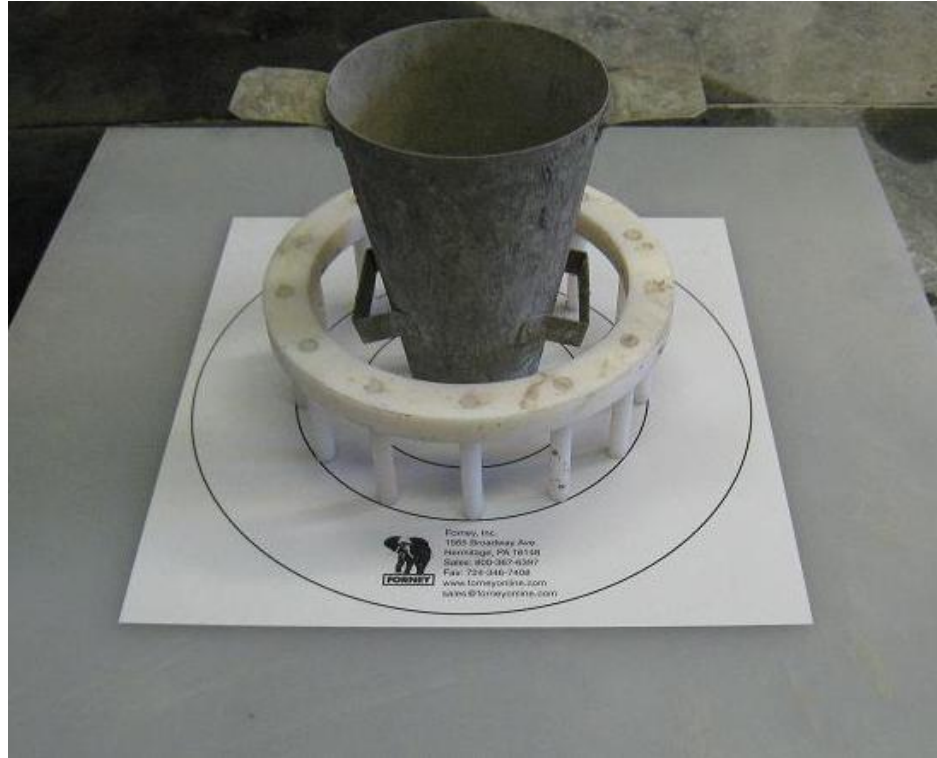
Figure 2.4: J-ring apparatus with slump cone (ACI 237 2007)
