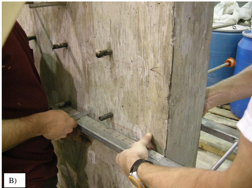
Figure 3.8: A) Measurement of wall thickness using a large caliper and ruler, and B) measurement taken using a 1/100 th in. gradation ruler
