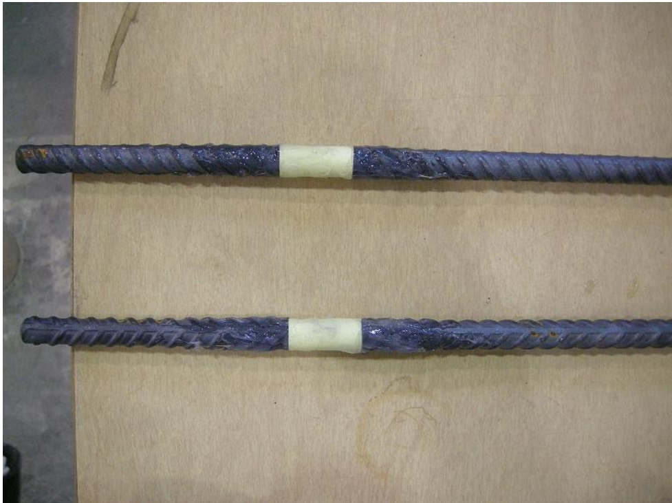
Figure 3.11: Application of Type I silicone to pullout bars
