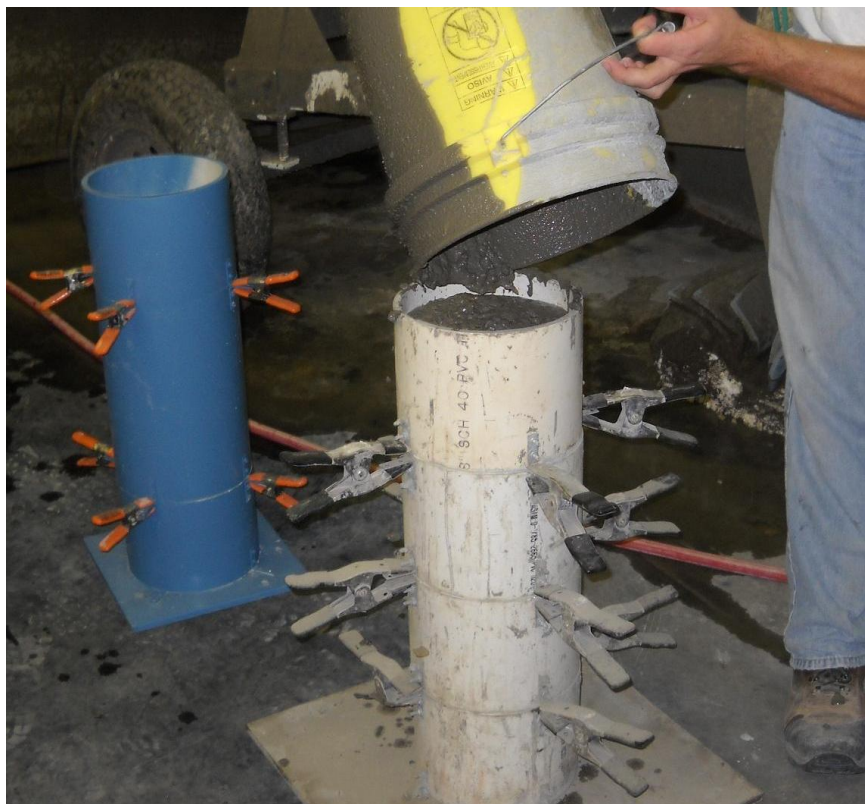
Figure 1.5: Filling of a column mold during the column segregation test
