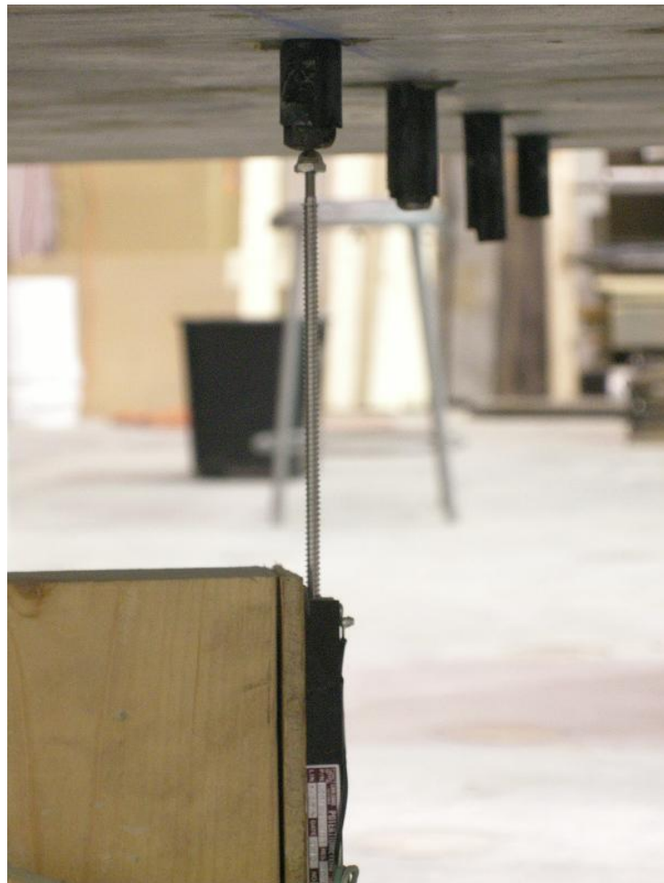
Figure 3.15: Spring-loaded linear potentiometer used to measure free-end slip
