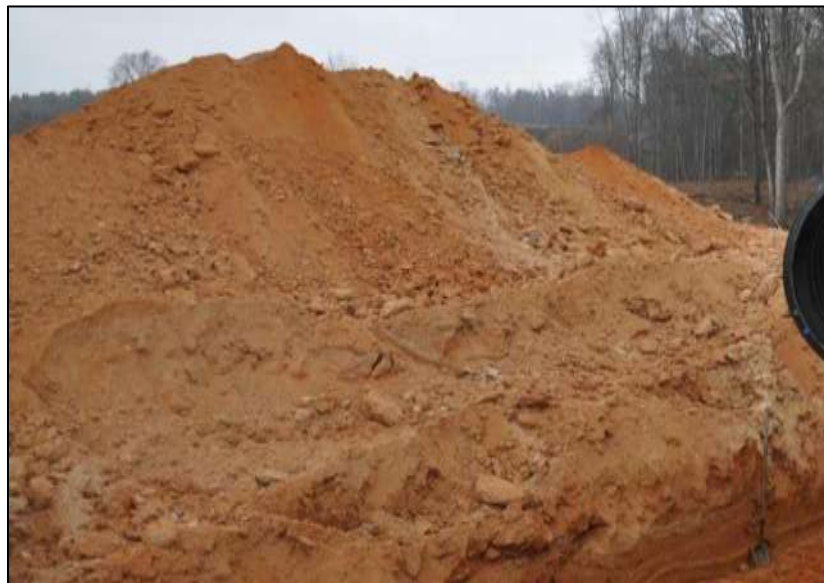
Figure 4-15: ASTM Class III Native Clay Backfill
