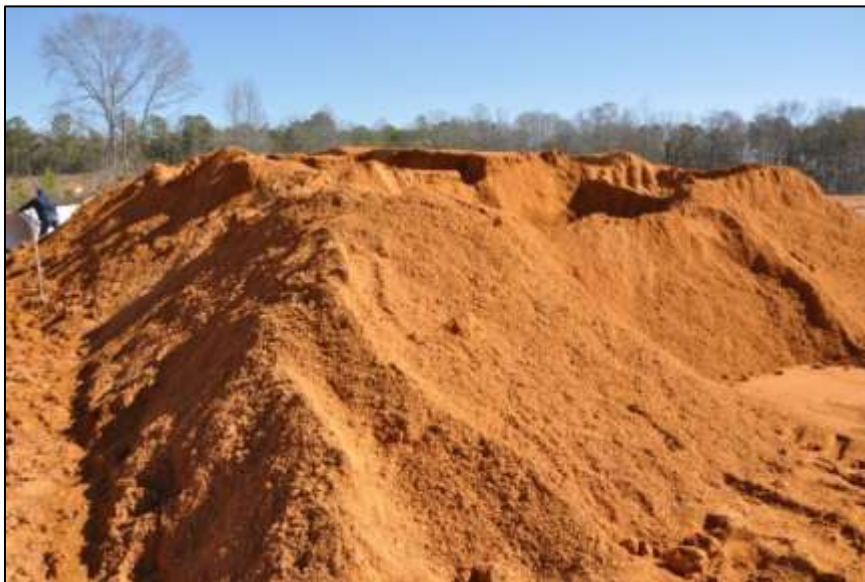
Figure 4-14: ASTM Class II Sandy Clay Backfill
