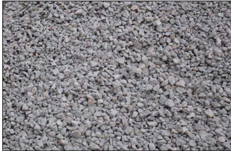
Figure 4-4: ASTM Class I Backfill (#57 Stone)
