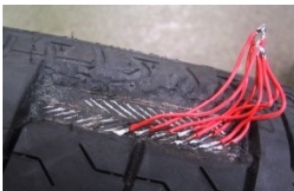
Figure 1.10: Capacitance change based wireless strain monitoring[66].
