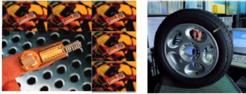
Figure 1.14: Seimens's[56] SAW sensor with energy generating piezoelectric crystals.
