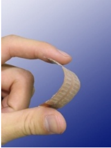
Figure 1.11: Flexible capacitance change based wireless strain monitoring[67].
