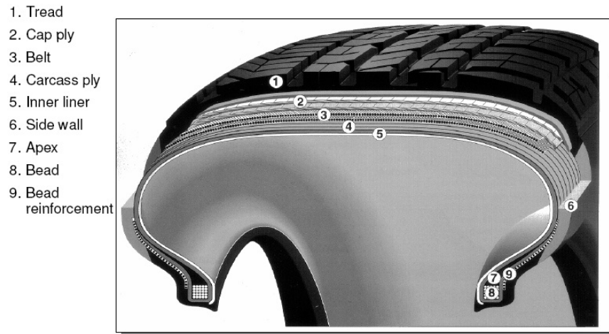
Figure 2.1: Typical components of a passenger car radial tire.
