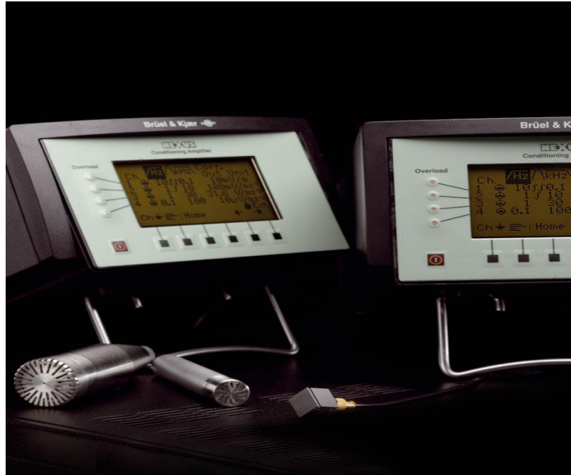
Figure A.2: Brüel & Kjaer 2693 NEXUS signal conditioning amplifier (an accelerometer is shown to the right of the microphones, microphones were not used in this study)
