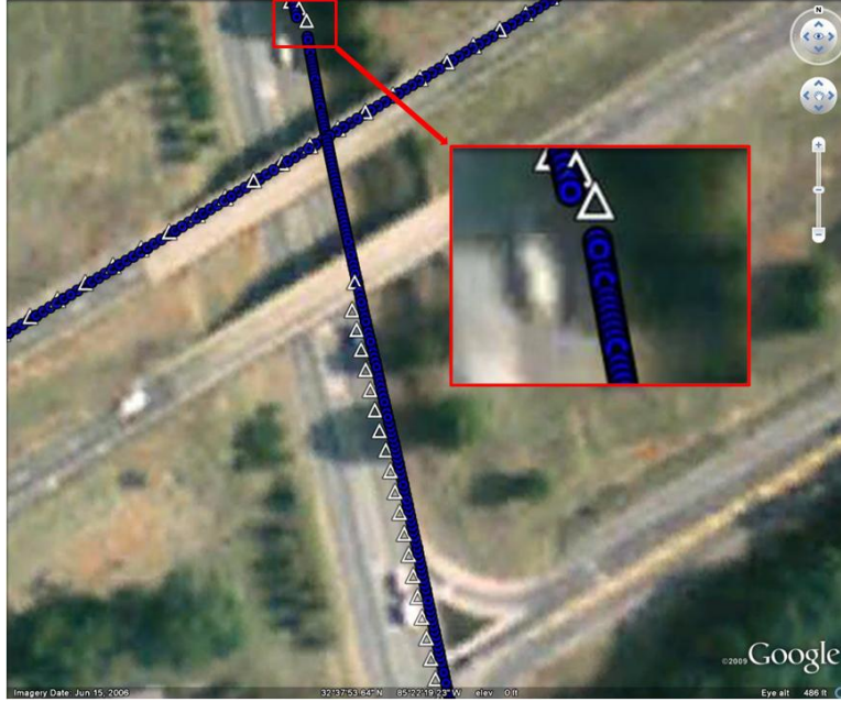
Figure 3.2: IMU dead reckoning under an overpass during GPS outage
