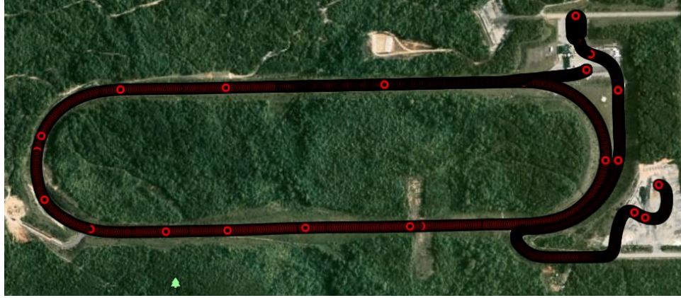
Figure 3.7: NCAT test facility with data collection locations. Background map by GPS Visualizer
