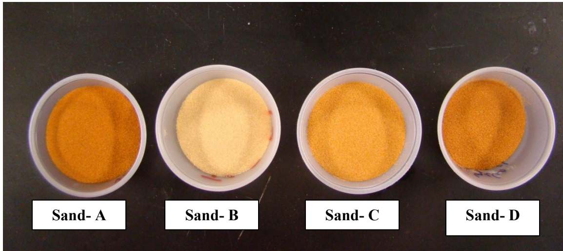
Figure 3-1 : Samples of the four synthetic goethite-coated sands
