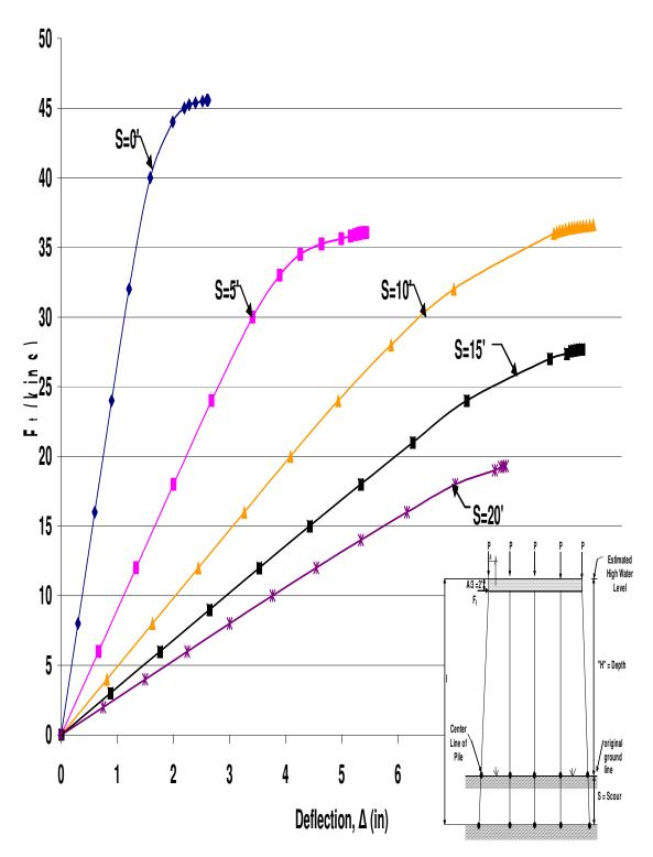
Figure A.49 HP10x42 Unbraced 5-Pile Bent with H=10', P=100kips and A=6'
