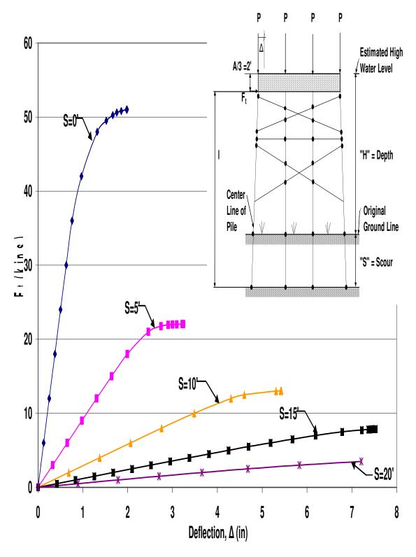
Figure A.42 HP10x42 Two-Story X-Braced 4-Pile Bent with H=21', P=120kips, and A=6'
