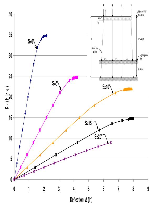
Figure A.26 HP10x42 Unbraced 4-Pile Bent with H=10', P=120kips, and A=6'
