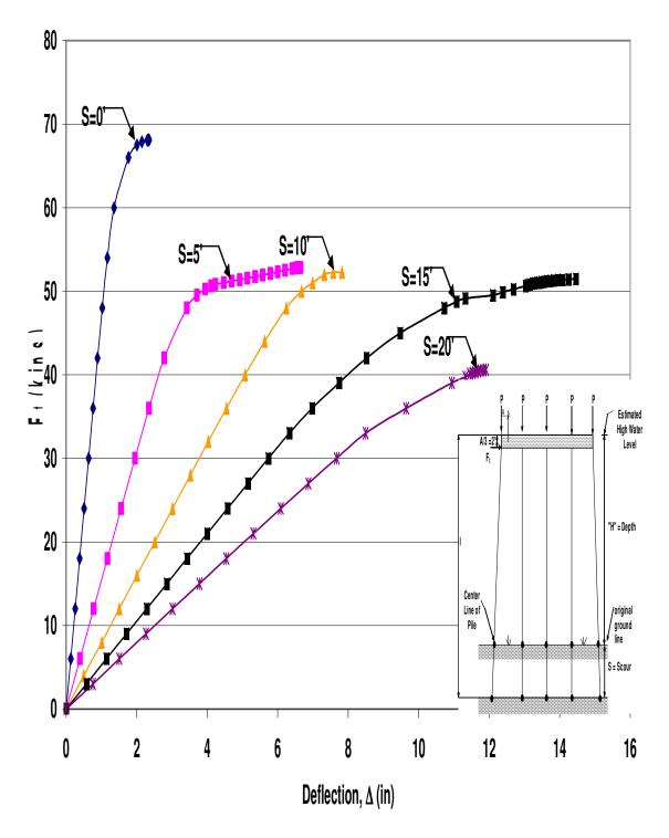
Figure B.49 HP12x53 Unbraced 5-Pile Bent with H=10',P=100kips and A=6'
