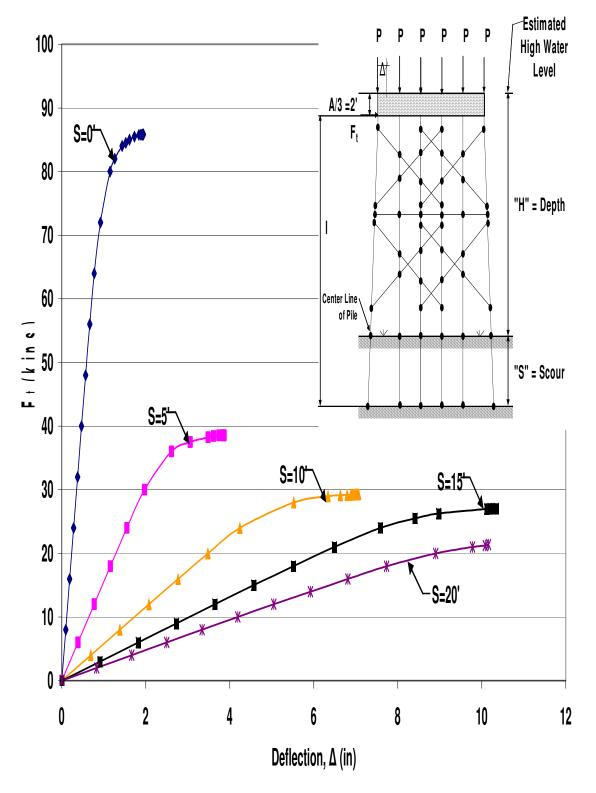
Figure A.105 HP10x42 Two-Story Double X-Braced 6-Pile Bent with H=21', P=100kips and A=6' Pushover Analysis Results
