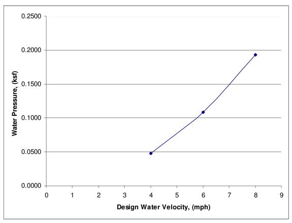
Figure 2.3 Relationship Between Water Pressure and Design Water Velocity for  $C_D = 1.4$
