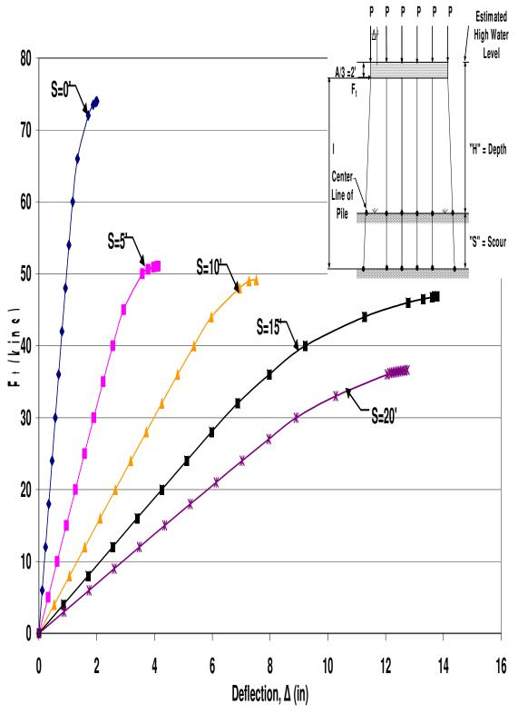
Figure B.74 HP12x53 Unbraced 6-Pile Bent with H=10', P=120kips and A=6'
