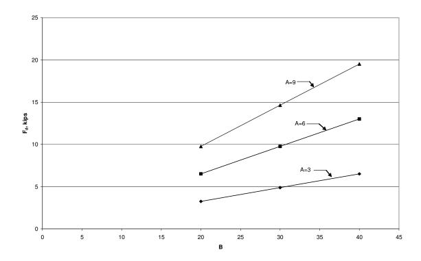
Figure 2.5 Debris Raft Force,  $F_T$ , for Various Debris Raft Dimensions (B) and (A) with  $V_{design} = 6mph$
