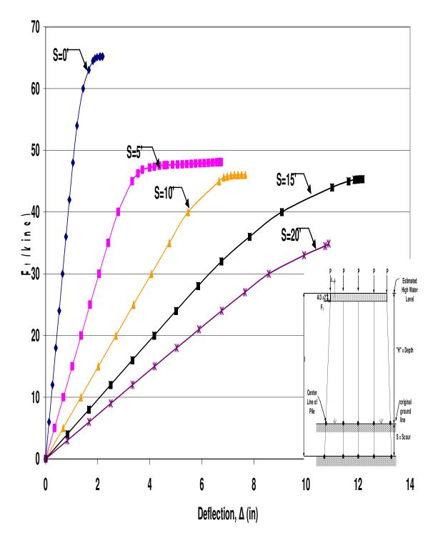
Figure B.50 HP12x53 Unbraced 5-Pile Bent with H=10', P=120kips and A=6'
