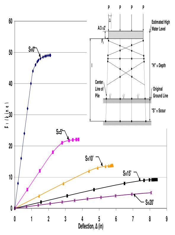
Figure A.45 HP10x42 Two-Story X-Braced 4-Pile Bent with H=25', P=100kips, and A=6'
