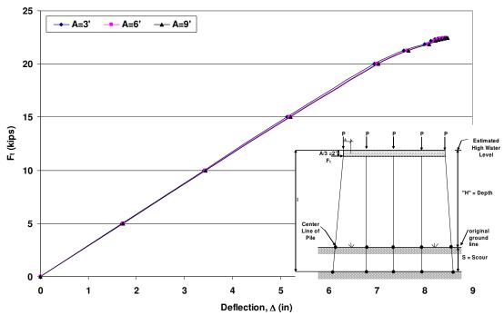
Figure 3.4 HP10x42 Unbraced 5-Pile Bent with H=13', S=15', and P=100kips Pushover Analysis Results
