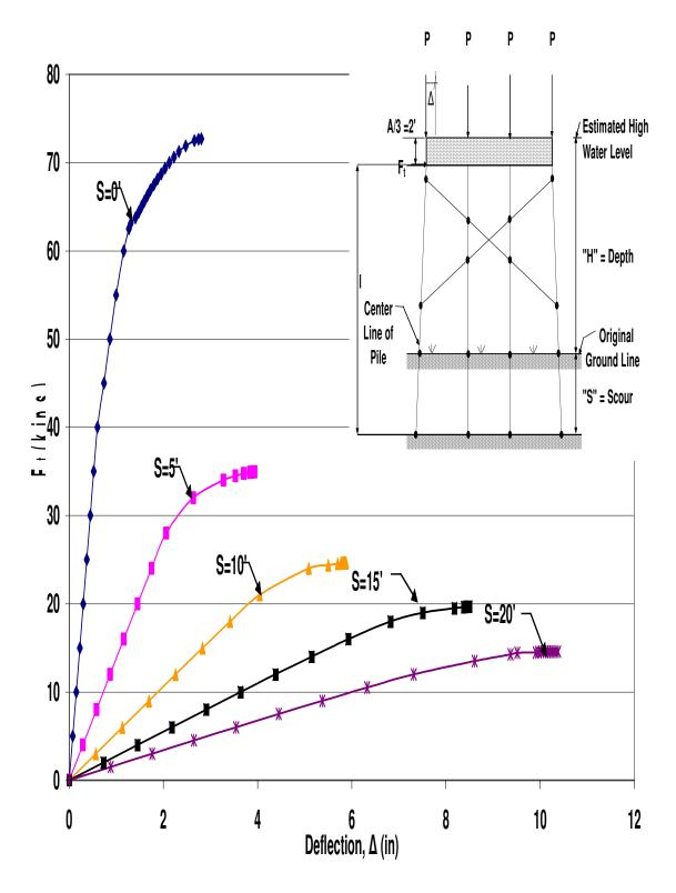
Figure B.39 HP12x53 X-Braced 4-Pile Bent with H=17', P=140kips and A=6'
