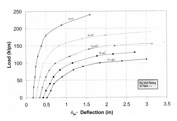
Figure 2.15 P- $\Delta_{top}$  Curves in Transverse Direction for HP10x42 Pile Bent in Figure 2.14 (Brown and Ramey 2003)
