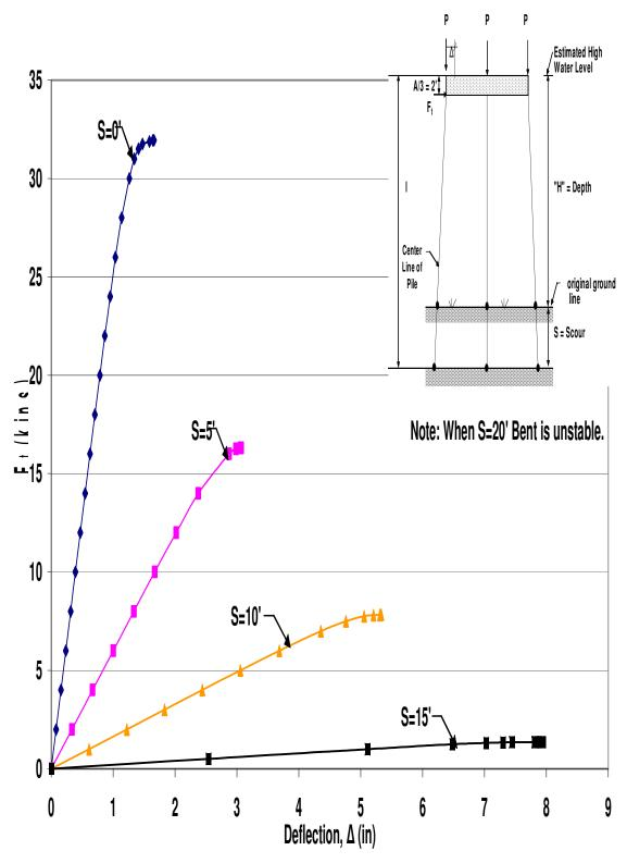
Figure B.4 HP12x53 Unbraced 3-Pile Bent with H=10', P=160kips and A=6'
