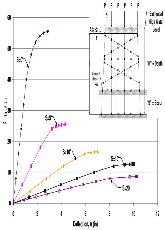
Figure A.102 HP10x42 Two-Story Single X-Braced 6-Pile Bent with H=25', P=120kips and A=6' Pushover Analysis Results
