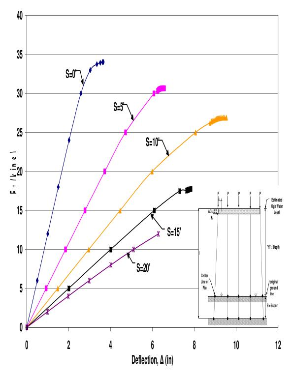
Figure A.54 HP10x42 Unbraced 5-Pile Bent with H=13', P=120kips and A=6'
