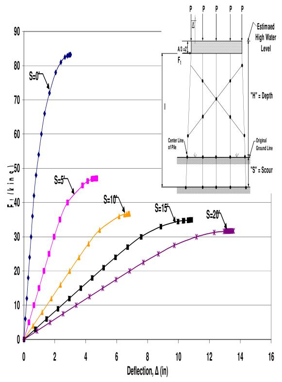
Figure B.62 HP12x53 X-Braced 5-Pile Bent with H=17', P=120kips and A=6'
