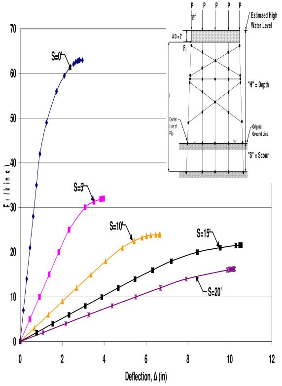
Figure A.65 HP10x42 Two-Story X-Braced 5-Pile Bent with H=21', P=100kips and A=6'
