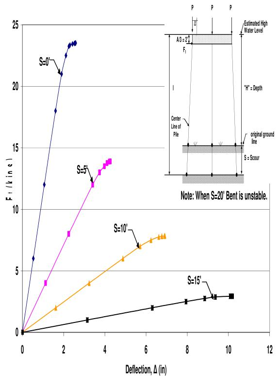
Figure B.6 HP12x53 Unbraced 3-Pile Bent with H=13', P=120kips and A=6'
