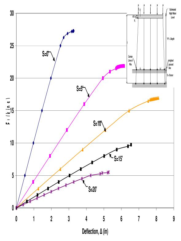
Figure A.56 HP10x42 Unbraced 5-Pile Bent with H=13', P=160kips and A=6'
