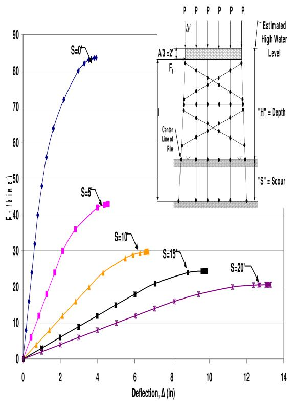
Figure B.103 HP12x53 Two-Story Single X-Braced 6-Pile Bent with H=25', P=140kips and A=6' Pushover Analysis Results
