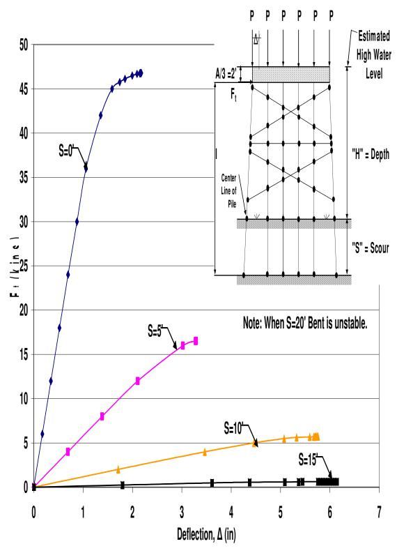
Figure A.104 HP10x42 Two-Story Single X-Braced 6-Pile Bent with H=25', P=160kips and A=6' Pushover Analysis Results
