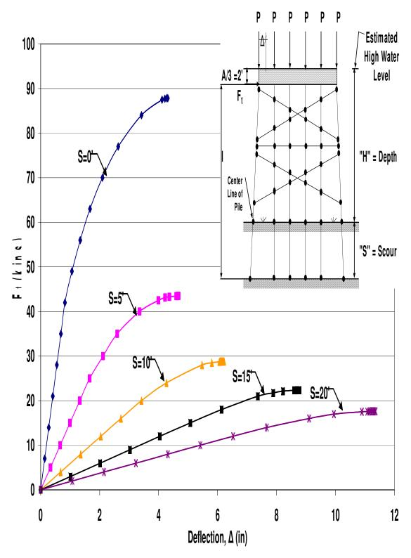
Figure B.100 HP12x53 Two-Story Single X-Braced 6-Pile Bent with H=21', P=160kips and A=6' Pushover Analysis Results
