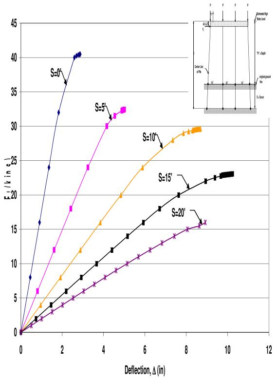
Figure B.31 HP12x53 Unbraced 4-Pile Bent with H=13', P=140kips, and A=6'
