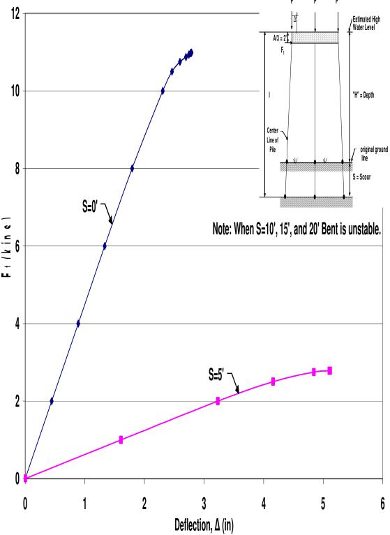
Figure A.7 HP10x42 Unbraced 3-Pile Bent with H=13', P=140kips and A=6' Pushover Analysis Results
