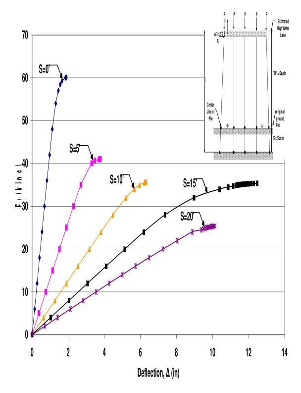
Figure B.52 HP12x53 Unbraced 5-Pile Bent with H=10', P=160kips and A=6'
