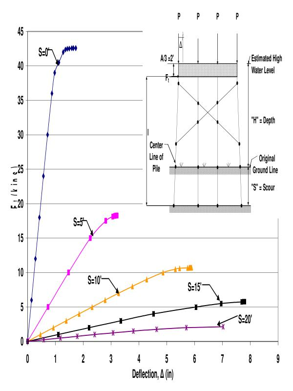
Figure A.39 HP10x42 X-Braced 4-Pile Bent with H=17', P=140kips and A=6'
