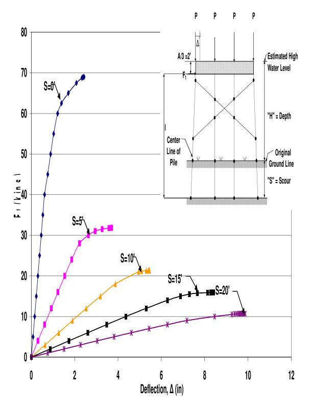
Figure B.40 HP12x53 X-Braced 4-Pile Bent with H=17', P=160kips and A=6'
