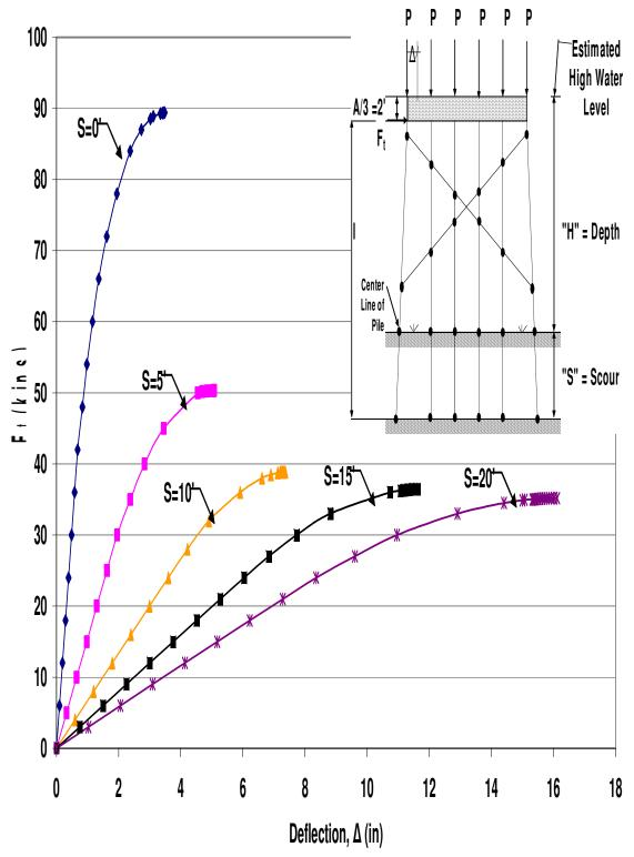
Figure B.86 HP12x53 Single X-Braced 6-Pile Bent with H=17', P=120kips and A=6'
