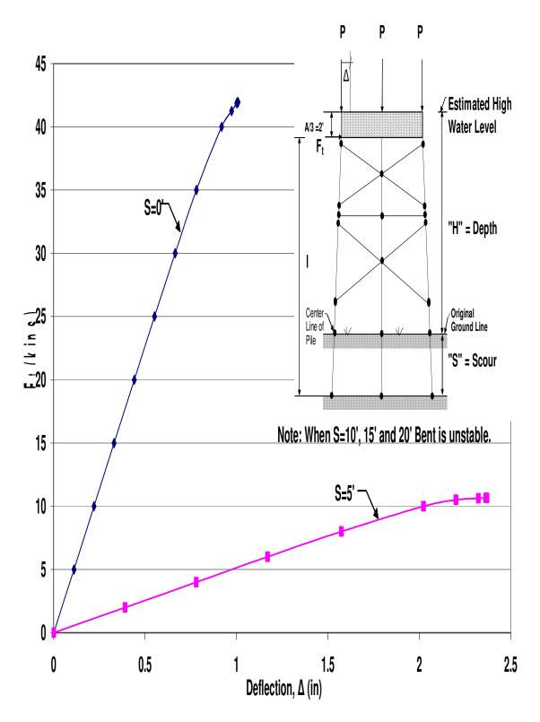
Figure A.23 HP10x42 Two-Story X-Braced 3-Pile Bent with H=25', P=140kips and A=6'
