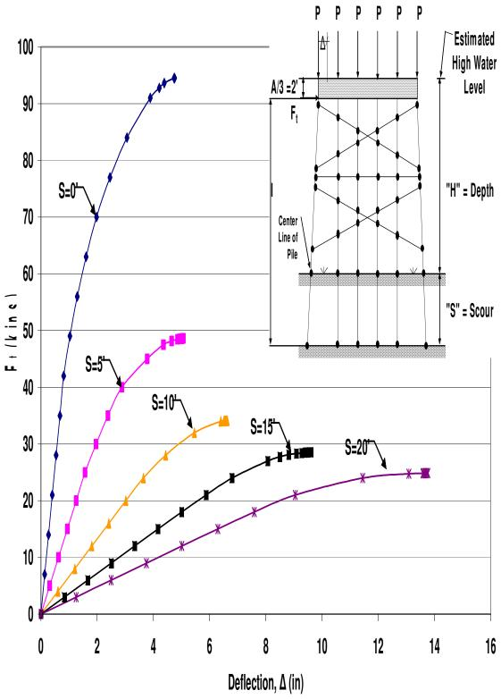
Figure B.99 HP12x53 Two-Story Single X-Braced 6-Pile Bent with H=21', P=140kips and A=6' Pushover Analysis Results
