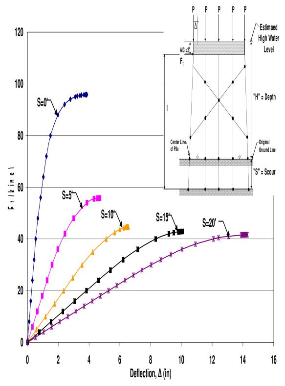
Figure B.57 HP12x53 X-Braced 5-Pile Bent with H=13', P=100kips and A=6'
