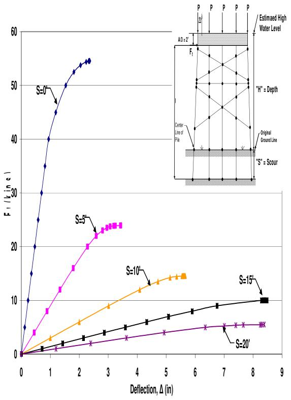
Figure A.67 HP10x42 Two-Story X-Braced 5-Pile Bent with H=21', P=140kips and A=6'
