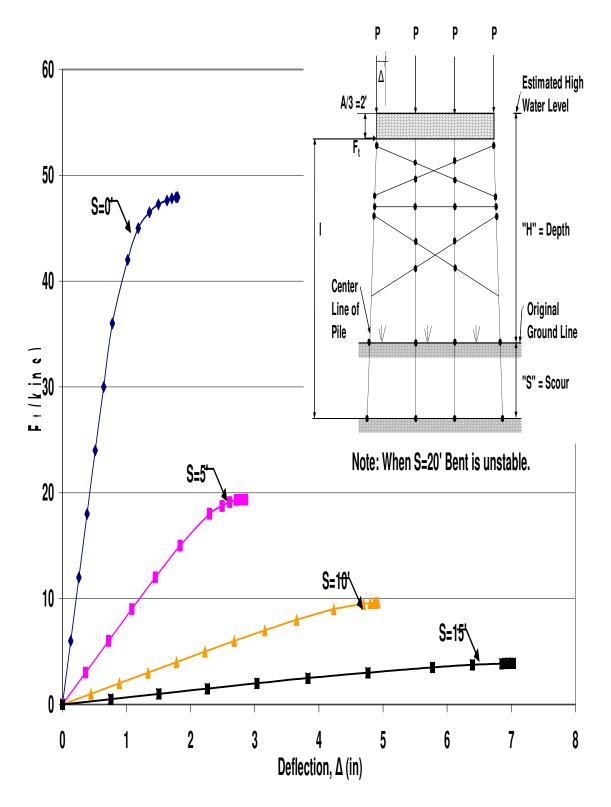
Figure A.43 HP10x42 Two-Story X-Braced 4-Pile Bent with H=21', P=140kips,and A=6'
