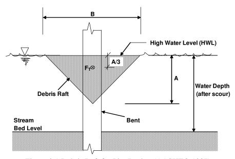
Figure 3.1 Debris Raft for Pier Design (AASHTO 1997)
