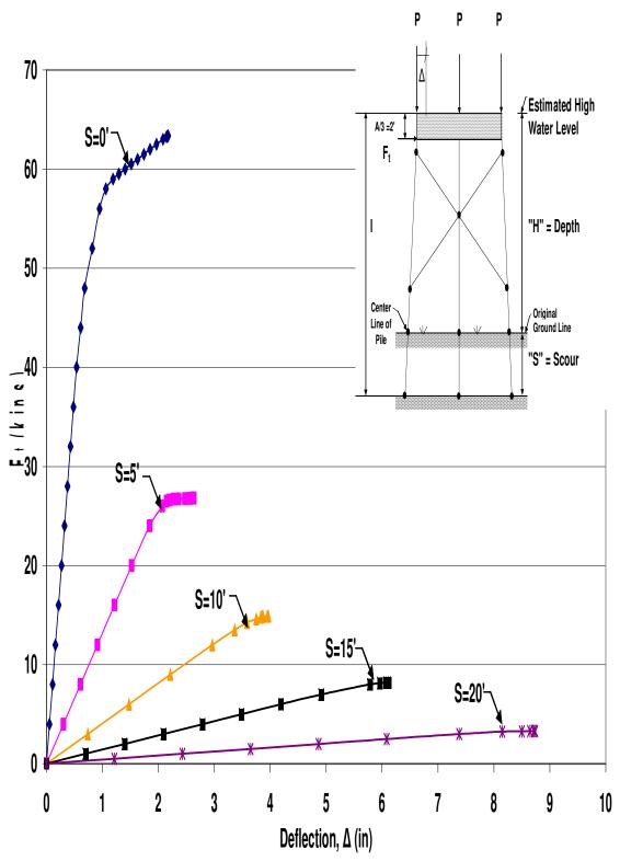
Figure B.13 HP12x53 X-Braced 3-Pile Bent with H=17', P=100 kips and A=6'
