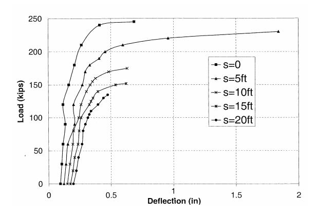
Figure 2.18 P- $\Delta_{top}$  Curves in Transverse Direction for Pile Bent in Figure 2.14 for Batter = 0.167 (Brown and Ramey 2003)
