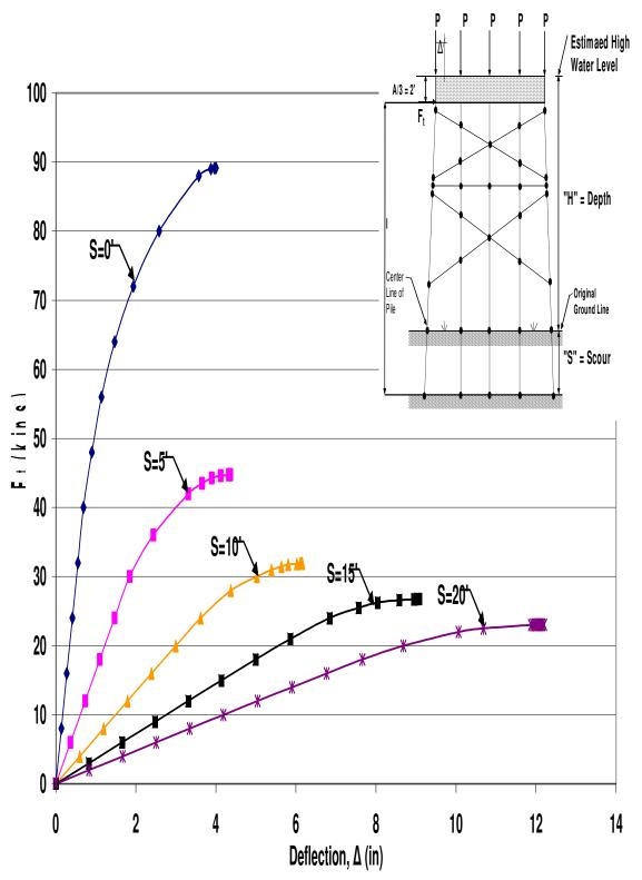
Figure B.67 HP12x53 Two-Story X-Braced 5-Pile Bent with H=21', P=140kips and A=6'
