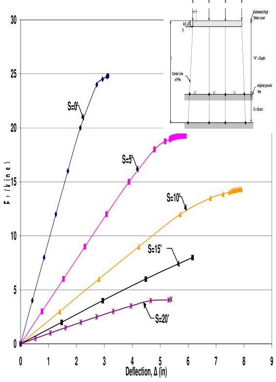
Figure A.31 HP10x42 Unbraced 4-Pile Bent with H=13', P=140kips and A=6'
