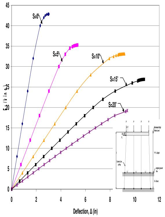
Figure B.30 HP12x53 Unbraced 4-Pile Bent with H=13', P=120kips, and A=6'
