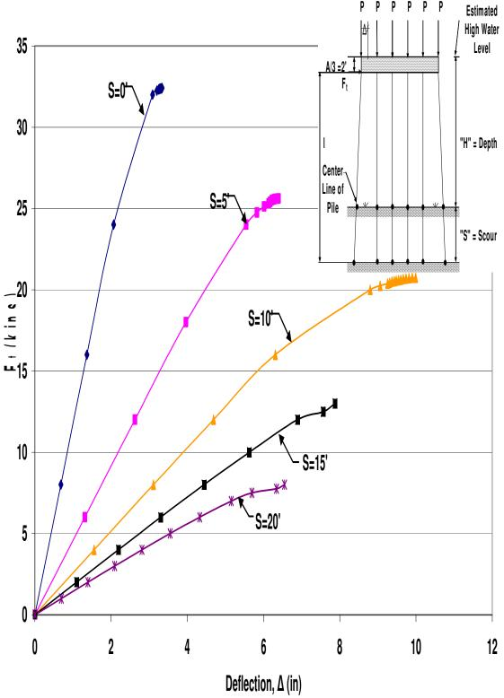
Figure A.79 HP10x42 Unbraced 6-Pile Bent with H=13', P=140kips and A=6'
