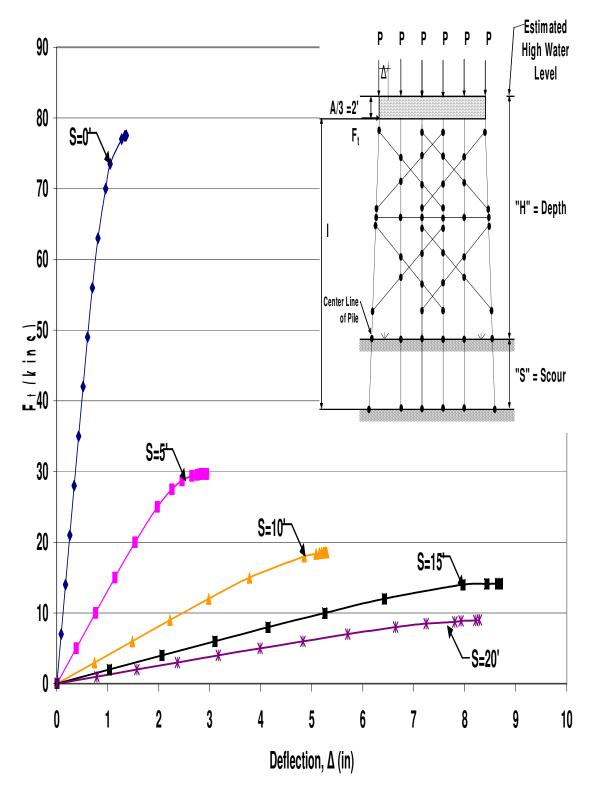
Figure A.107 HP10x42 Two-Story Double X-Braced 6-Pile Bent with H=21', P=140kips and A=6' Pushover Analysis Results
