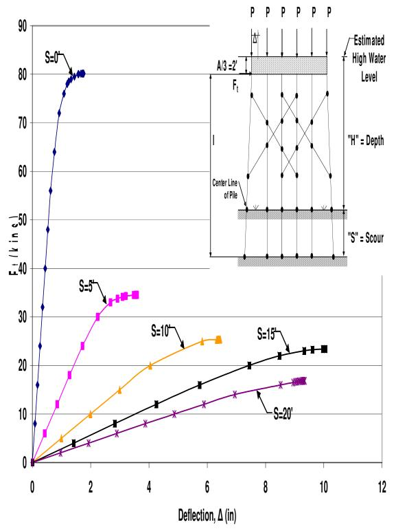
Figure A.90 HP10x42 Double X-Braced 6-Pile Bent with H=13', P=120kips and A=6'
