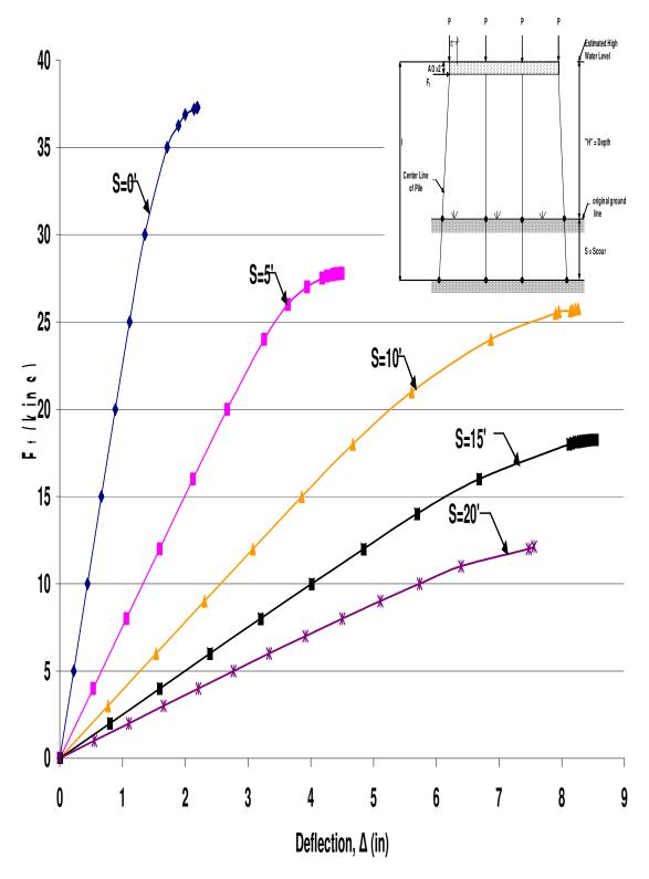
Figure A.25 HP10x42 Unbraced 4-Pile Bent with H=10', P=100kips, and A=6'
