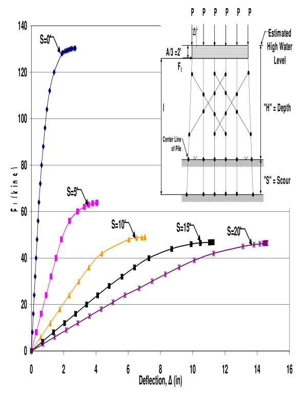
Figure B.89 HP12x53 Double X-Braced 6-Pile Bent with H=13', P=100kips and A=6'
