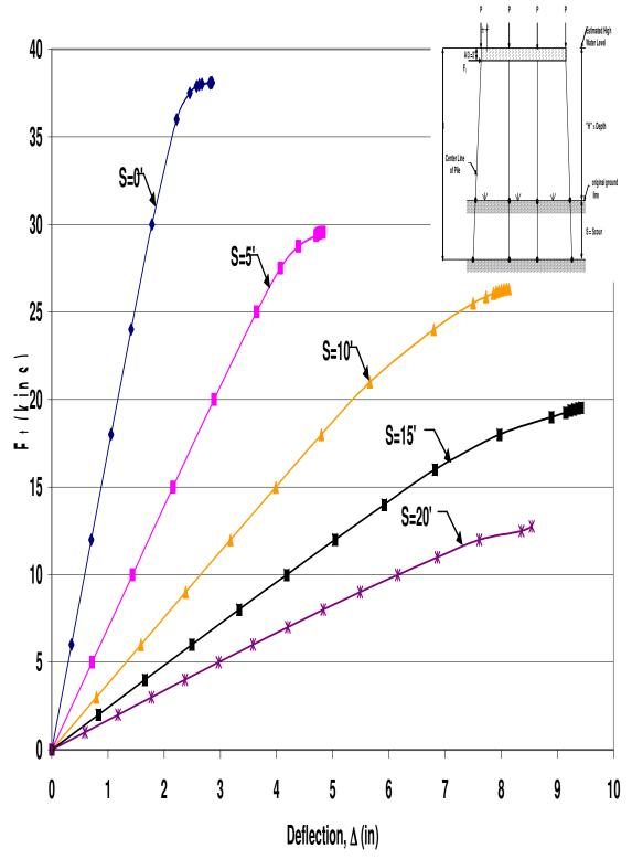
Figure B.32 HP12x53 Unbraced 4-Pile Bent with H=13', P=160kips, and A=6'
