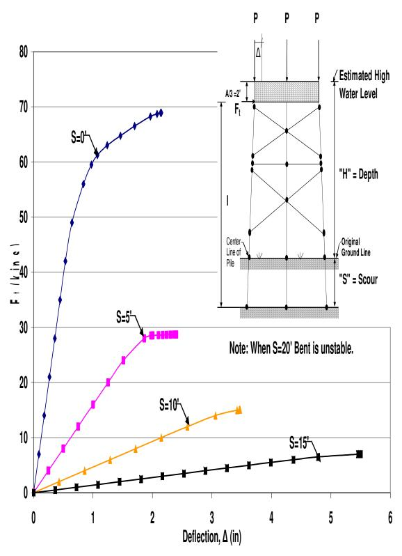
Figure B.18 HP12x53 Two-Story X-Braced 3-Pile Bent with H=21',P=120kips and A=6'
