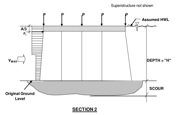
Figure 2.7 Sections Showing Longitudinal And Transverse Flood Water Loading on Bent (see Fig. 2.6)
