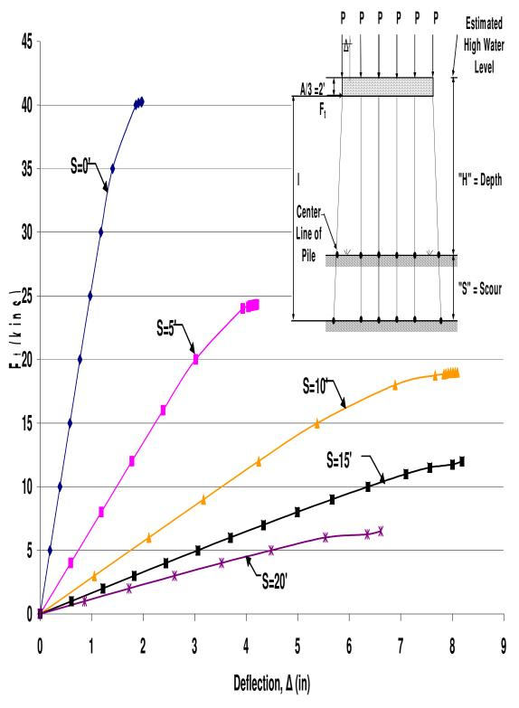
Figure A.76 HP10x42 Unbraced 6-Pile Bent with H=10', P=160kips and A=6'
