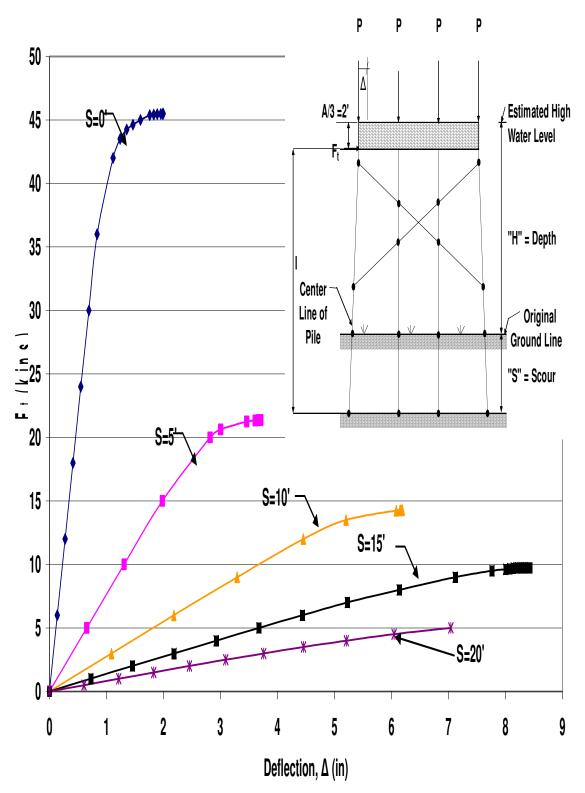
Figure A.38 HP10x42 X-Braced 4-Pile Bent with H=17',P=120kips, and A=6'
