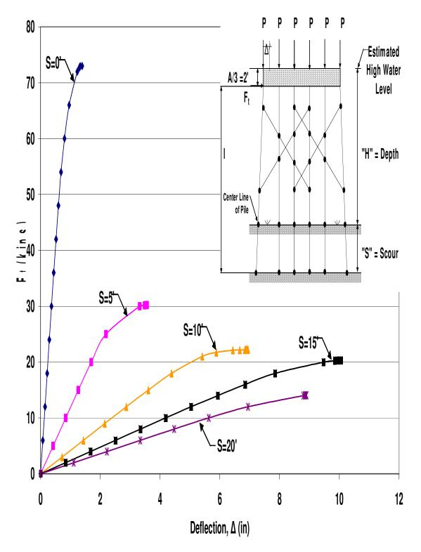
Figure A.94 HP10x42 Double X-Braced 6-Pile Bent with H=17', P=120kips and A=6'
