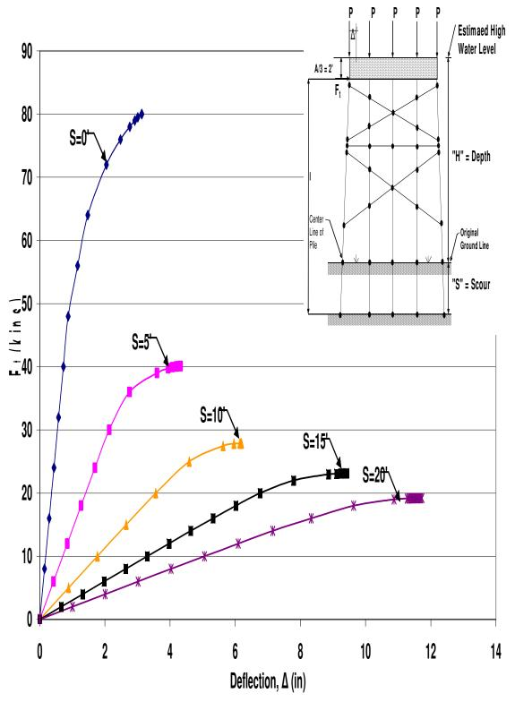
Figure B.71 HP12x53 Two-Story X-Braced 5-Pile Bent with H=25', P=140kips and A=6'
