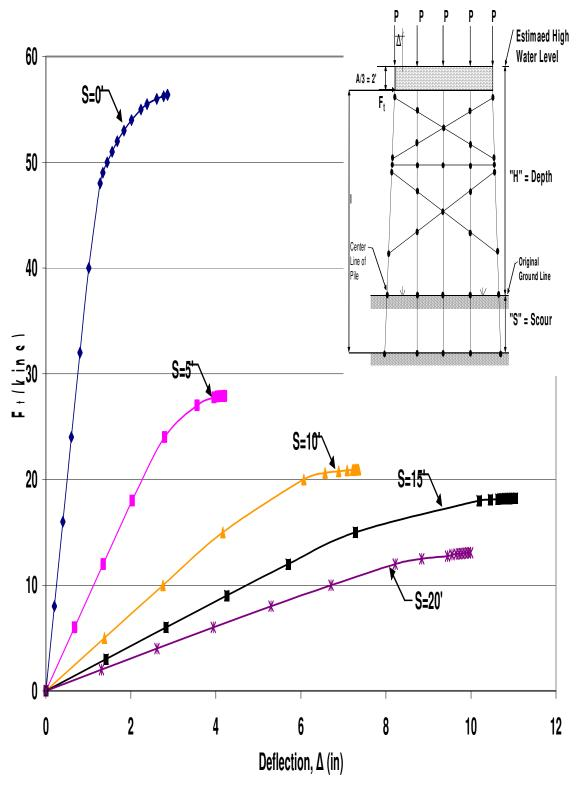
Figure A.69 HP10x42 Two-Story X-Braced 5-Pile Bent with H=25', P=100kips and A=6'
