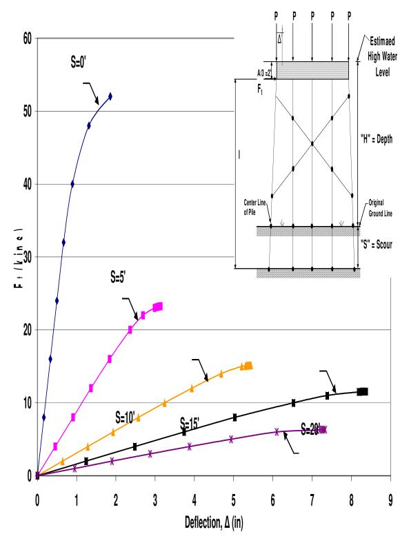
Figure A.60 HP10x42 X-Braced 5-Pile Bent with H=13',P=160kips and A=6'
