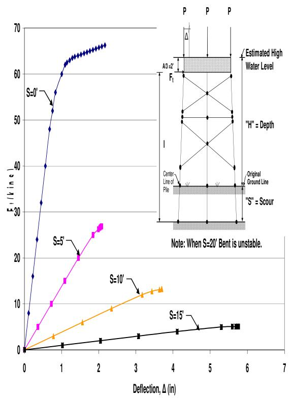
Figure B.22 HP12x53 Two-Story X-Braced 3-Pile Bent with H=25',P=120kips and A=6'
