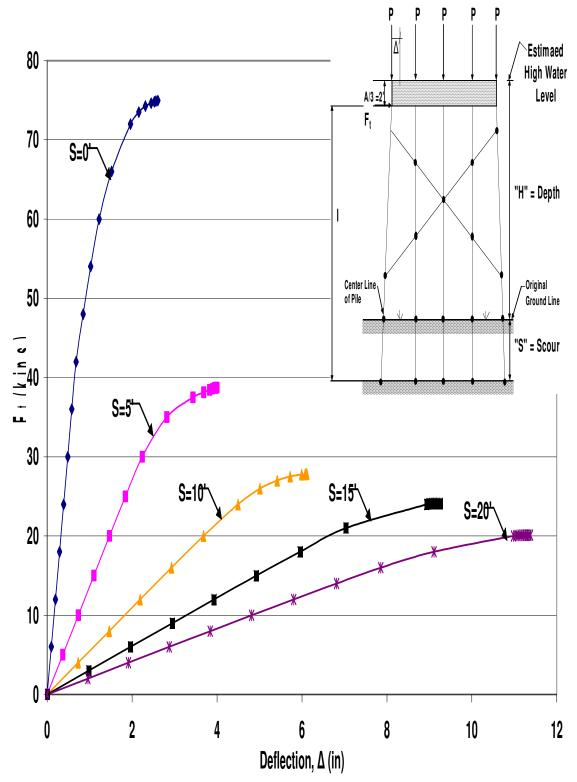
Figure B.64 HP12x53 X-Braced 5-Pile Bent with H=17', P=160kips and A=6'
