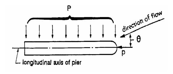
Figure 2.8 Plan View of Pier Showing Stream Flow Pressure (AASHTO 3.7.3.2-1)
