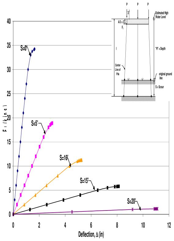
Figure B.2 HP12x53 Unbraced 3-Pile Bent with H=10', P=120kips and A=6',
