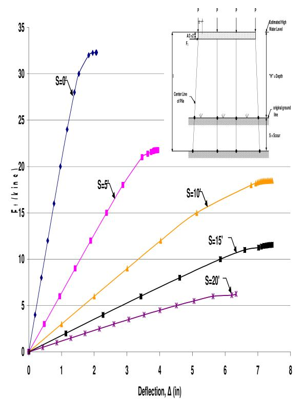
Figure A.27 HP10x42 Unbraced 4-Pile Bent with H=10', P=140kips, and A=6'
