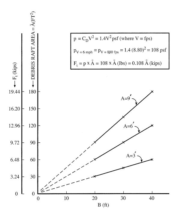
Figure 3.2 Bent  $F_t$  Force for Various Debris Raft Dimensions for  $V_{Design} = 6mph$
