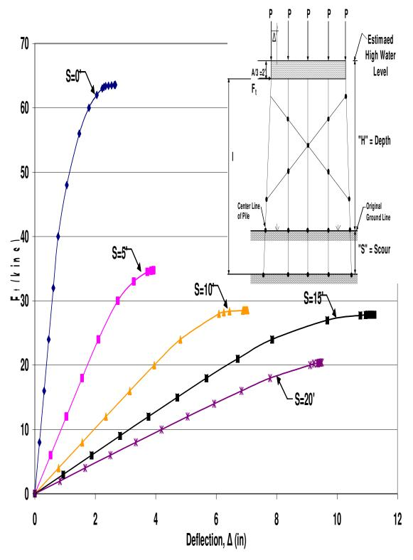
Figure A.57 HP10x42 X-Braced 5-Pile Bent with H=13', P=100kips and A=6'
