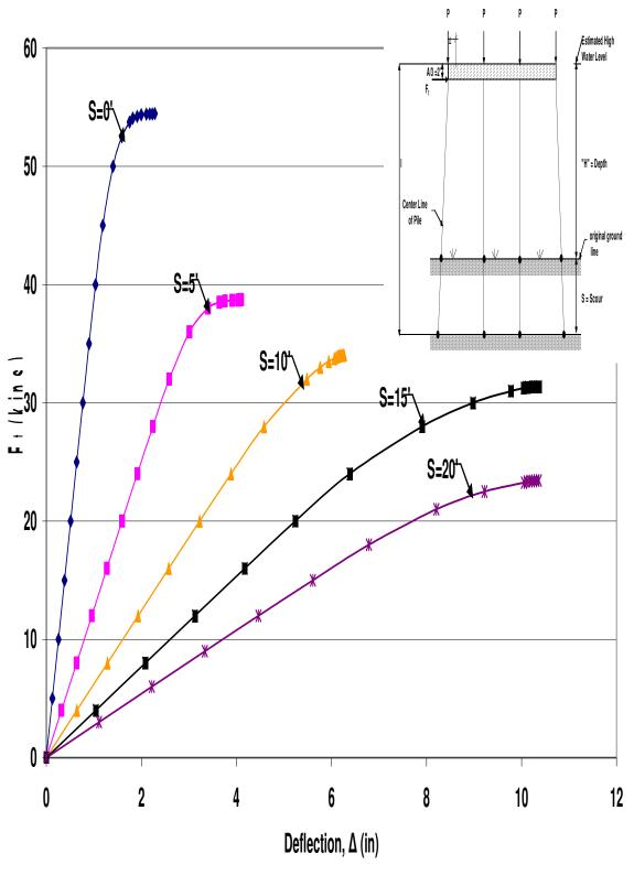
Figure B.26 HP12x53 Unbraced 4-Pile Bent with H=10', P=120kips and A=6'
