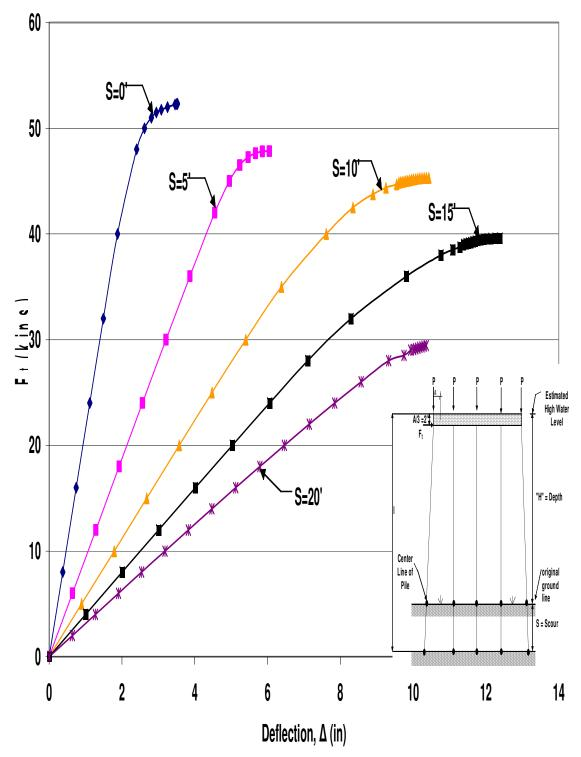
Figure B.54 HP12x53 Unbraced 5-Pile Bent with H=13', P=120kips and A=6'
