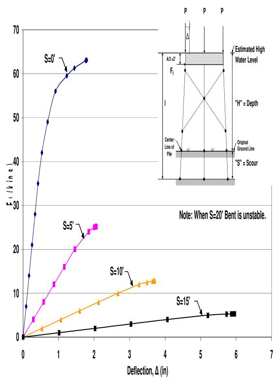
Figure B.11 HP12x53 X-Braced 3-Pile Bent with H=13', P=140kips and A=6'
