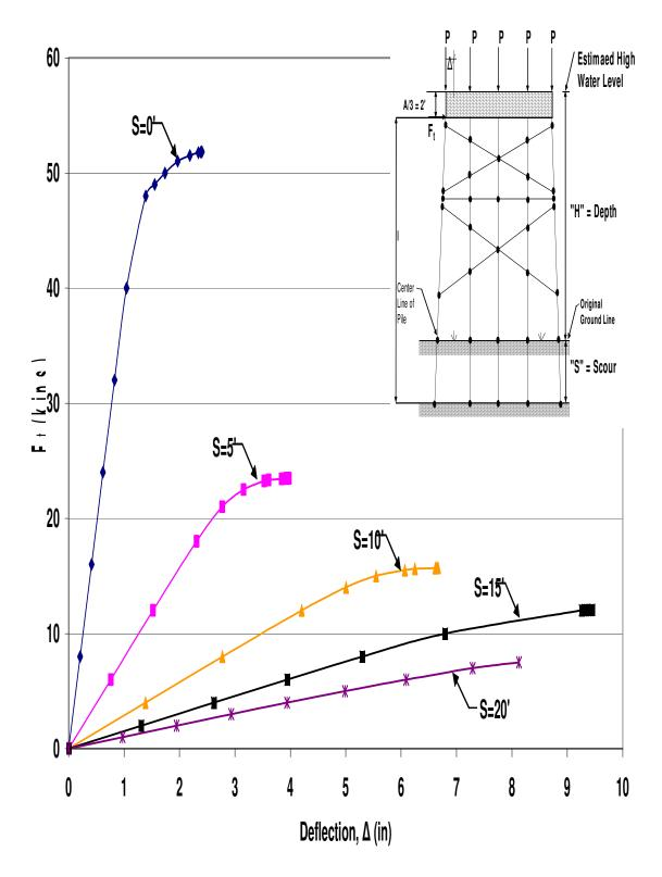
Figure A.70 HP10x42 Two-Story X-Braced 5-Pile Bent with H=25', P=120kips and A=6' Pushover Analysis Results
