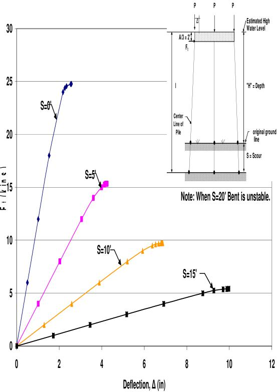
Figure B.5 HP12x53 Unbraced 3-Pile Bent with H=13', P=100kips and A=6'
