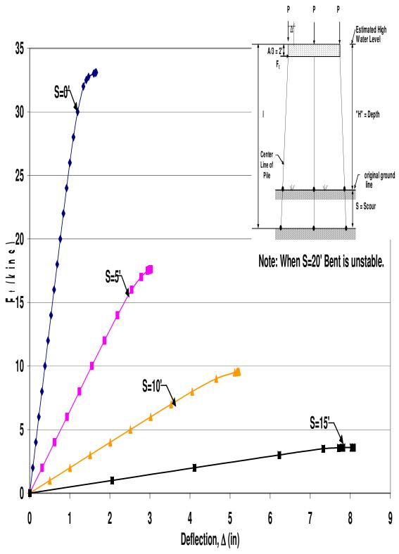
Figure B.3 HP12x53 Unbraced 3-Pile Bent with H=10', P=140kips and A=6'
