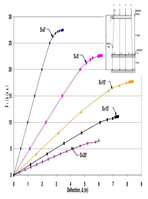
Figure A.30 HP10x42 Unbraced 4-Pile Bent with H=13', P=120kips and A=6'
