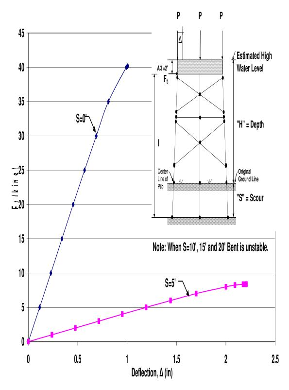
Figure A.24 HP10x42 Two-Story X-Braced 3-Pile Bent with H=25', P=160kips and A=6'
