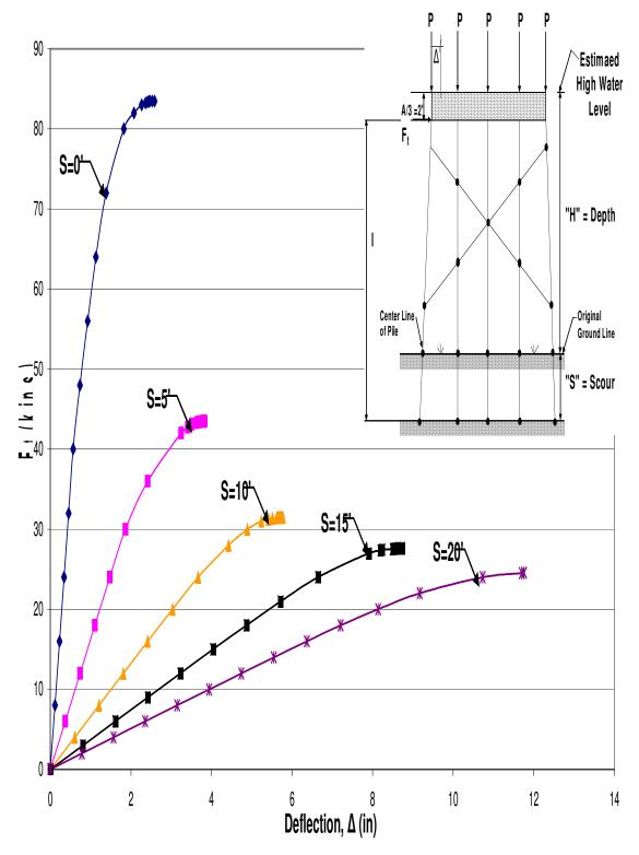
Figure B.60 HP12x53 X-Braced 5-Pile Bent with H=13', P=160kips and A=6'
