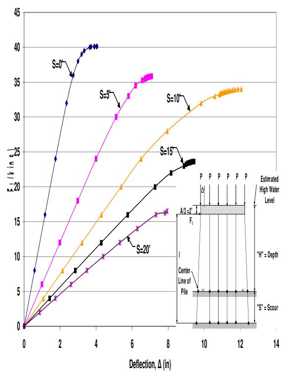
Figure A.77 HP10x42 Unbraced 6-Pile Bent with H=13',P=100kips and A=6'
