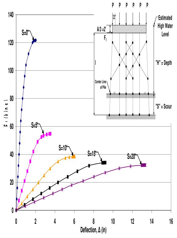
Figure B.91 HP12x53 Double X-Braced 6-Pile Bent with H=13', P=140kips and A=6'
