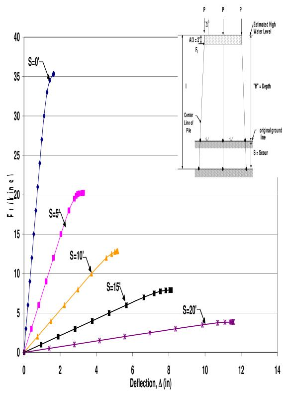
Figure B.1 HP12x53 Unbraced 3-PileBent with H=10', P=100kips and A=6'
