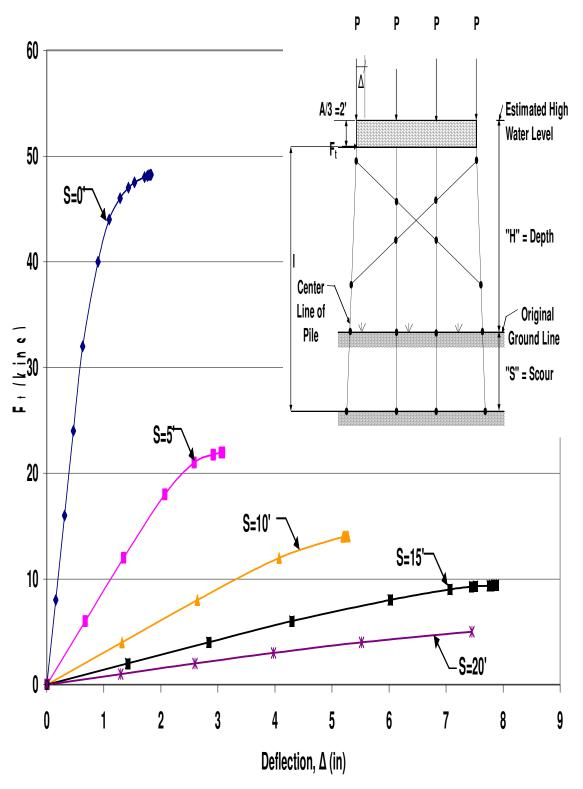
Figure A.35 HP10x42 X-Braced 4-Pile Bent with H=13', P=140kips, and A=6'
