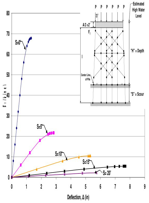
Figure A.112 HP10x42 Two-Story Double X-Braced 6-Pile Bent with H=25', P=160kips and A=6' Pushover Analysis Results
