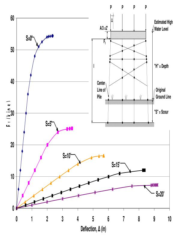
Figure A.41 HP10x42 Two-Story X-Braced 4-Pile Bent with H=21', P=100kips and A=6'
