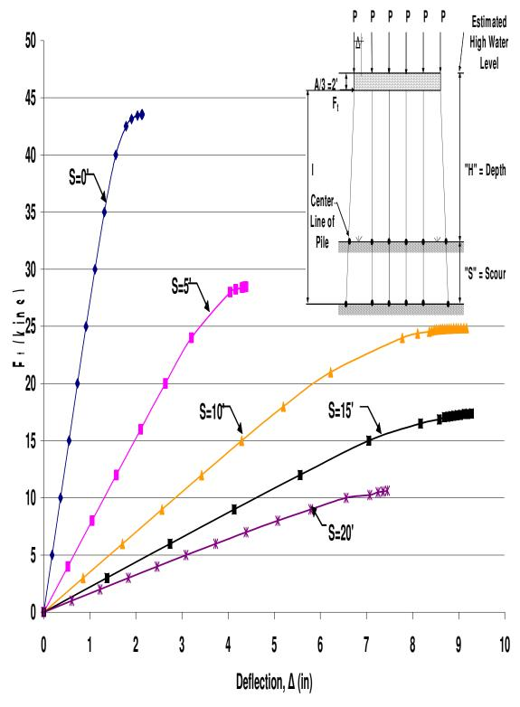
Figure A.75 HP10x42 Unbraced 6-Pile Bent with H=10', P=140kips and A=6'
