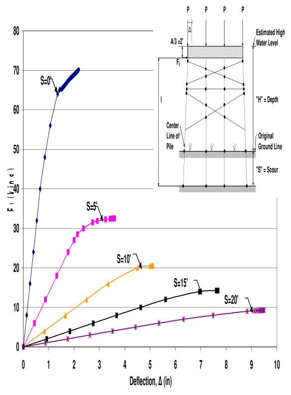
Figure B.47 HP12x53 Two-Story X-Braced 4-Pile Bent with H=25', P=140kips and A=6'
