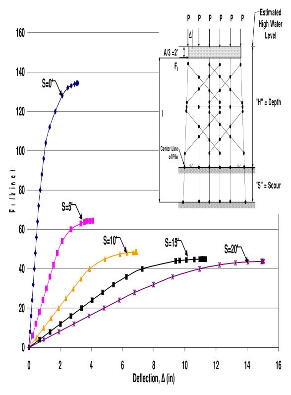
Figure B.105 HP12x53 Two-Story Double X-Braced 6-Pile Bent with H=21', P=100kips and A=6' Pushover Analysis Results
