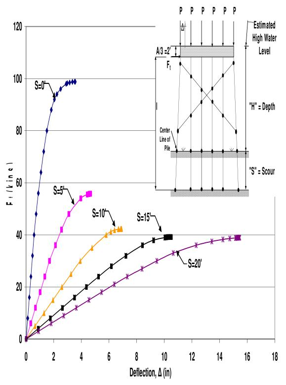
Figure B.82 HP12x53 Single X-Braced 6-Pile Bent with H=13', P=120kips and A=6'
