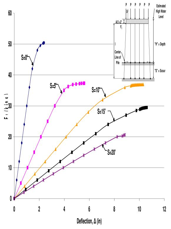
Figure A.73 HP10x42 Unbraced 6-Pile Bent with H=10', P=100kips and A=6'
