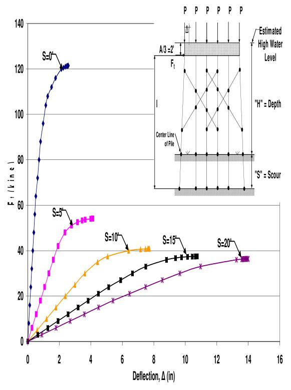
Figure B.94 HP12x53 Double X-Braced 6-Pile Bent with H=17', P=120kips and A=6'
