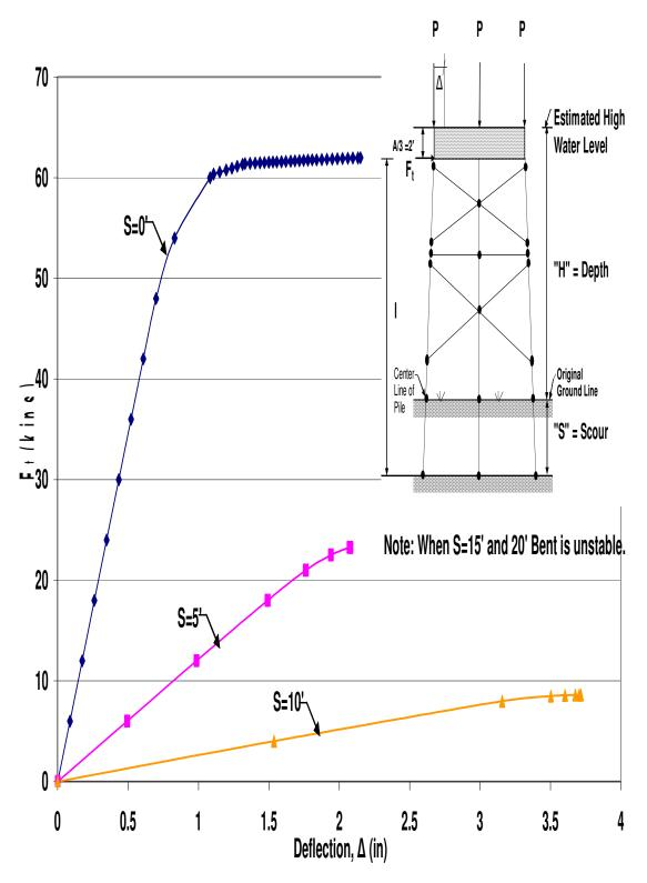
Figure B.24 HP12x53 Two-Story X-Braced 3-Pile Bent with H=25',P=160kips and A=6'
