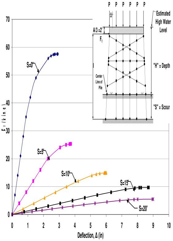
Figure A.99 HP10x42 Two-Story Single X-Braced 6-Pile Bent with H=21', P=140kips and A=6' Pushover Analysis Results
