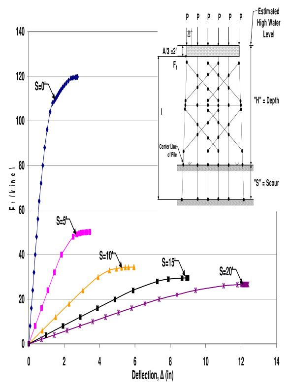
Figure B.111 HP12x53 Two-Story Double X-Braced 6-Pile Bent with H=25', P=140kips and A=6' Pushover Analysis Results 342
