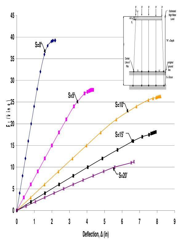
Figure A.51 HP10x42 Unbraced 5-Pile Bent with H=10', P=140kips and A=6'
