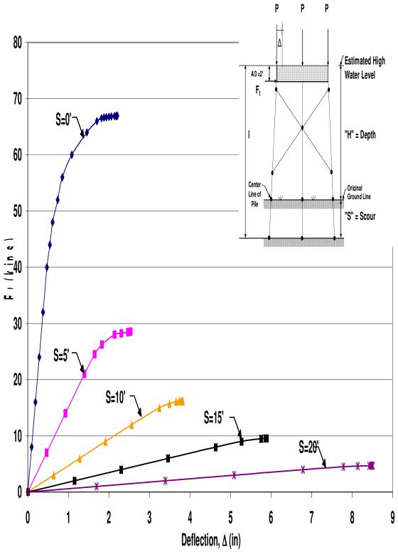
Figure B.9 HP12x53 X-Braced 3-Pile Bent with H=13', P=100kips and A=6'
