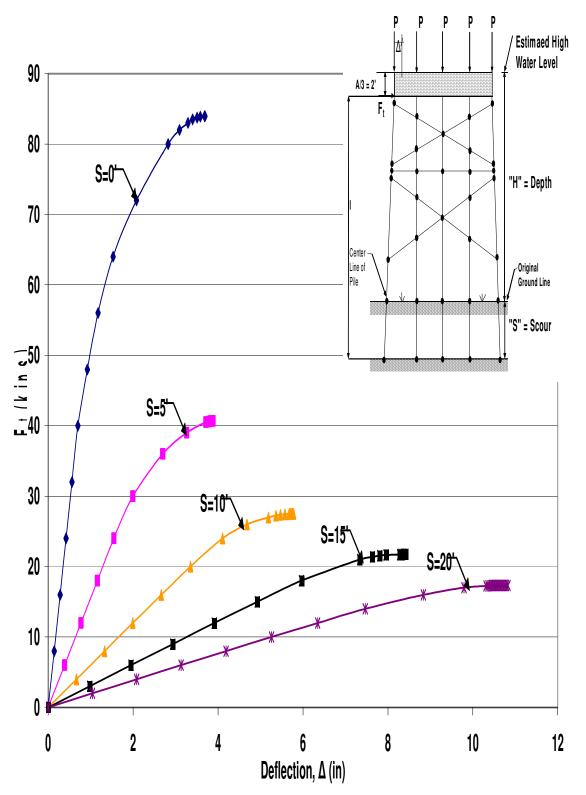
Figure B.68 HP12x53 Two-Story X-Braced 5-Pile Bent with H=21', P=160kips and A=6'
