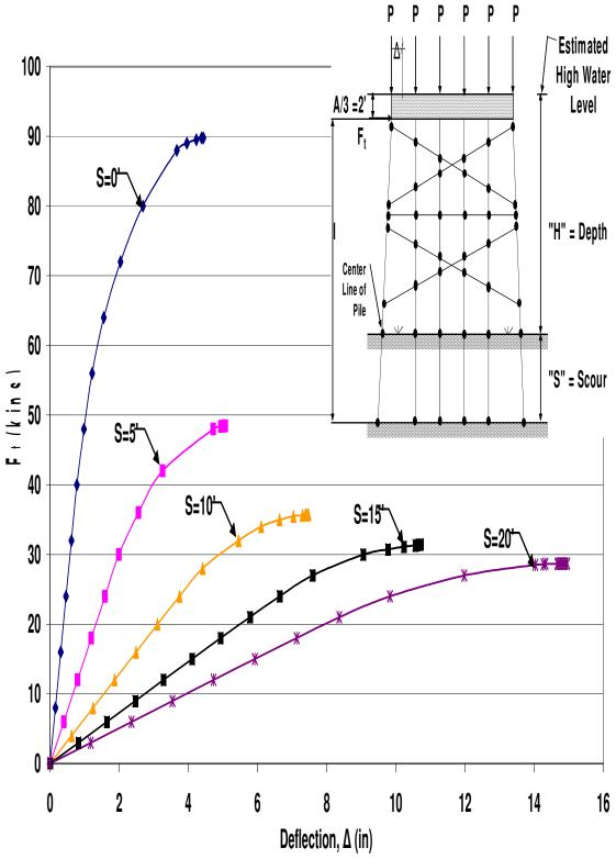
Figure B.102 HP12x53 Two-Story Single X-Braced 6-Pile Bent with H=25', P=120kips and A=6' Pushover Analysis Results
