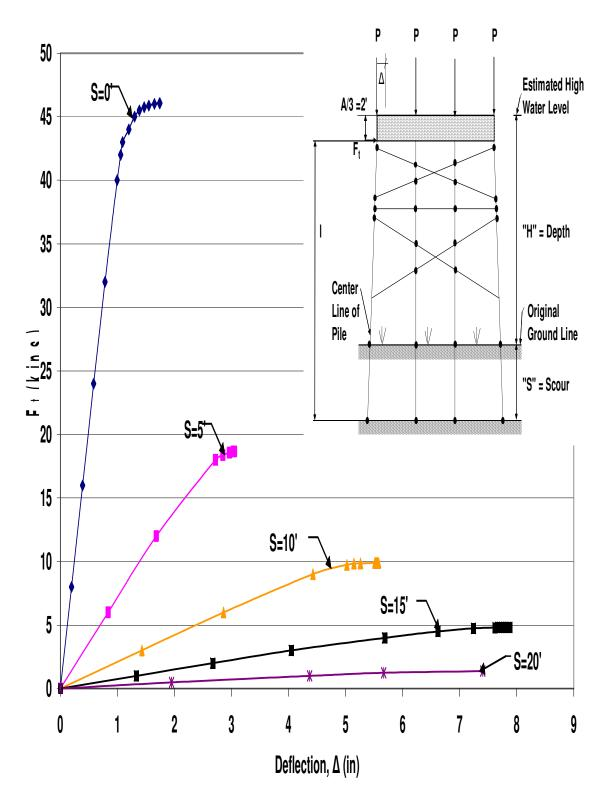
Figure A.46 HP10x42 Two-Story X-Braced 4-Pile bent with H=25',P=120kips, and A=6'
