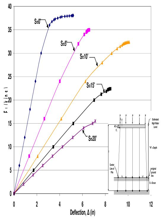
Figure A.53 HP10x42 Unbraced 5-Pile Bent with H=13', P=100kips and A=6'
