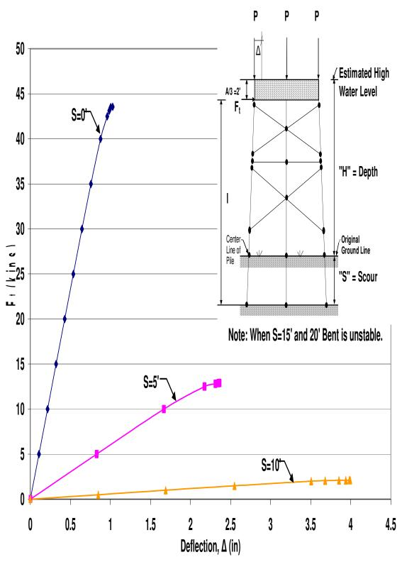
Figure A.22 HP10x42 Two-Story X-Braced 3-Pile Bent with H=25', P=120kips, and A=6'
