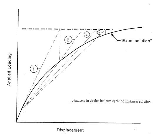
Figure 2.12 Direct Iteration Solution Procedure (GTSTRUDL 2002)
