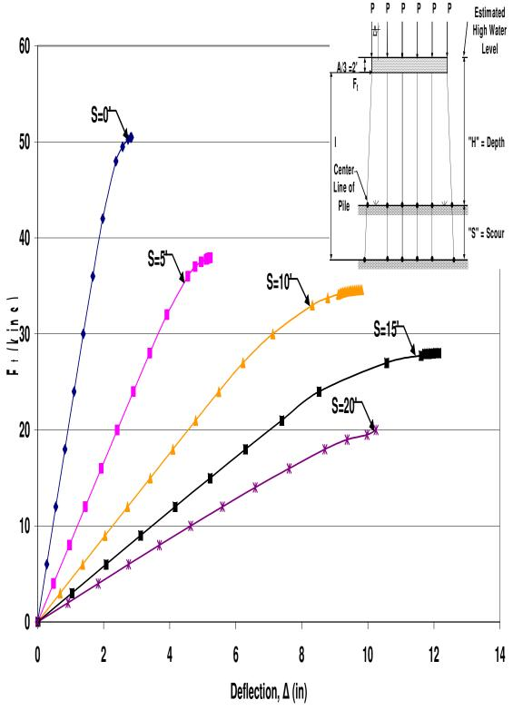
Figure B.80 HP12x53 Unbraced 6-Pile Bent with H=13', P=160kips and A=6'
