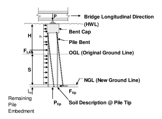
Figure 4.9 Evaluation of Bent Pile "Kick-Out" Load from Extreme Flood/Scour Event
