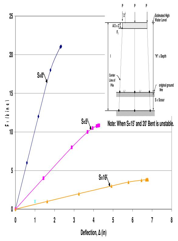
Figure B.8 HP12x53 Unbraced 3-Pile with H=13', P=160kips and A=6'
