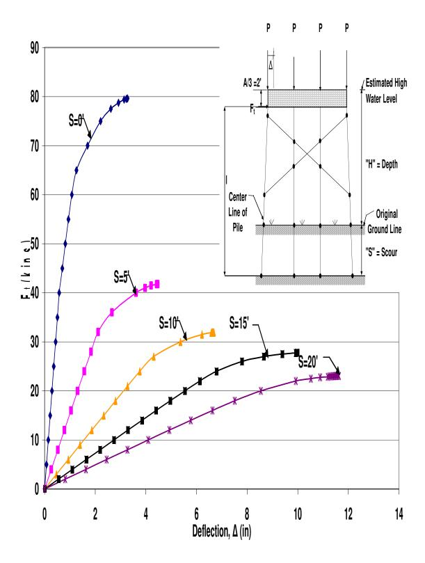
Figure B.37 HP12x53 X-Braced 4-Pile Bent with H=17', P=100kips and A=6'
