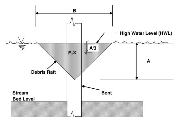
Figure 2.4 Debris Raft for Bent Design (AASHTO 1997)
