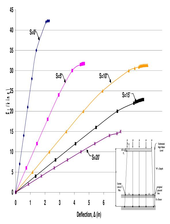
Figure A.50 HP10x42 Unbraced 5-Pile Bent with H=10', P=120kips and A=6'
