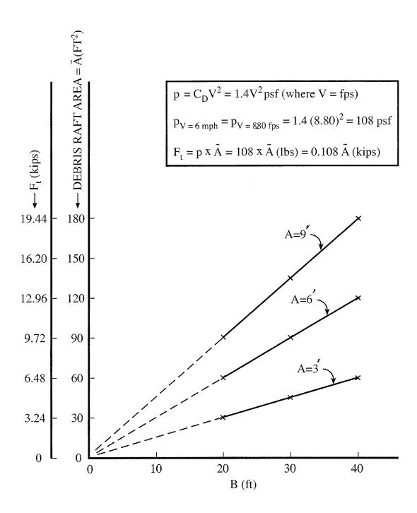
Figure 4.6 Bent  $F_t$  Force for Various Debris Raft Dimensions for  $V_{Design} = 6mph$
