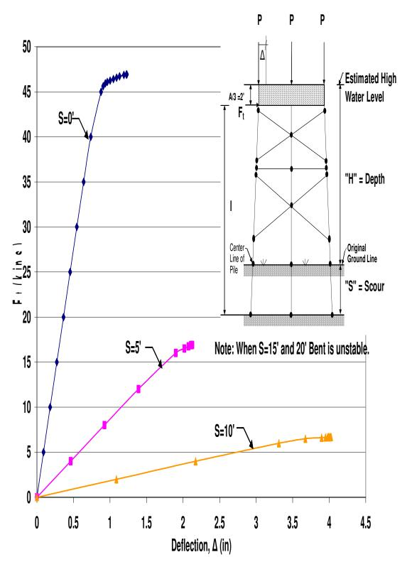
Figure A.17 HP10x42 Two-Story X-Braced 3-Pile Bent with H=21', P=100kips, and A=6'
