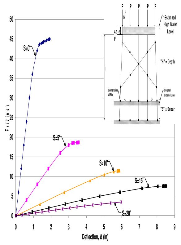
Figure A.64 HP10x42 X-Braced 5-Pile Bent with H=17', P=160kips and A=6'
