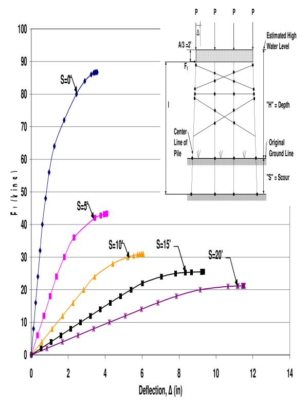
Figure B.41 HP12x53 Two-Story X-Braced 4-Pile Bent with H=21', P=100kips and A=6'
