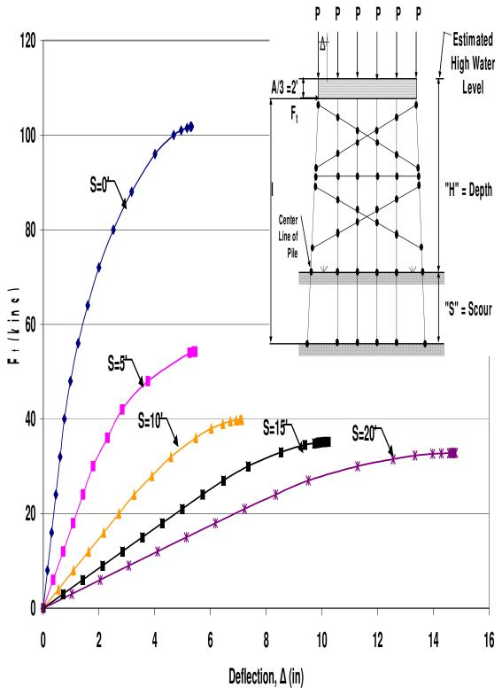
Figure B.98 HP12x53 Two-Story Single X-Braced 6-Pile Bent with H=21', P=120kips and A=6' Pushover Analysis Results 329
