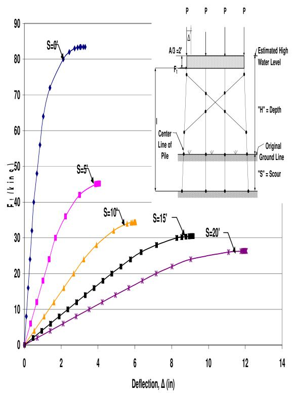
Figure B.33 HP12x53 X-Braced 4-Pile Bent with H=13', P=100kips and A=6'
