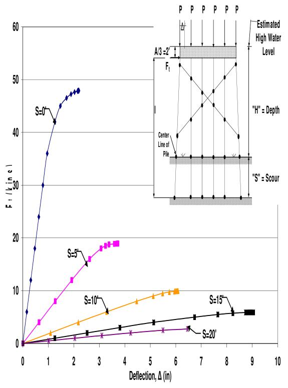
Figure A.88 HP10x42 Single X-Braced 6-Pile Bent with H=17', P=160kips and A=6'
