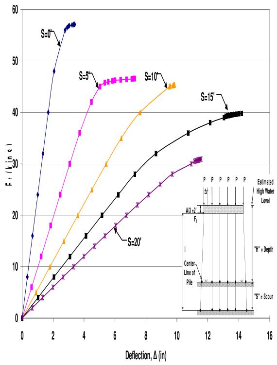
Figure B.78 HP12x53 Unbraced 6-Pile Bent with H=13', P=120kips and A=6'
