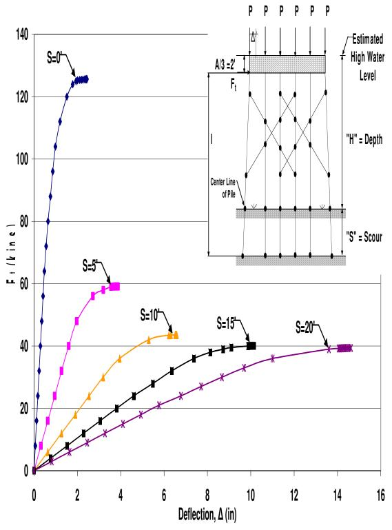
Figure B.90 HP12x53 Double X-Braced 6-Pile Bent with H=13', P=120kips and A=6'
