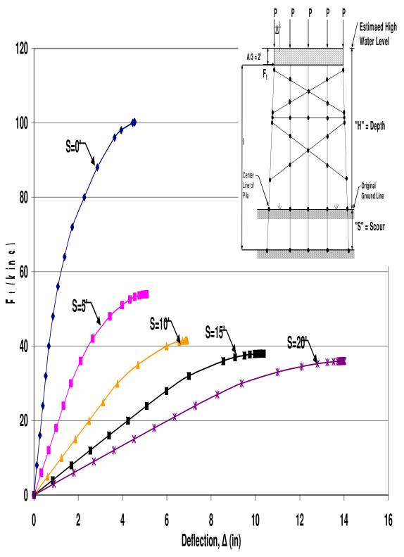
Figure B.65 HP12x53 Two-Story X-Braced 5-Pile Bent with H=21', P=100kips and A=6'
