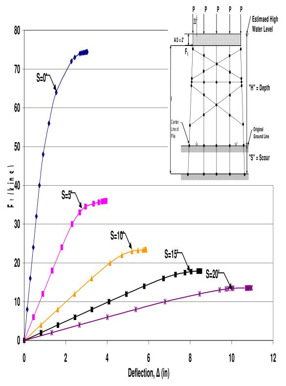
Figure B.72 HP12x53 Two-Story X-Braced 5-Pile Bent with H=25', P=160kips and A=6'
