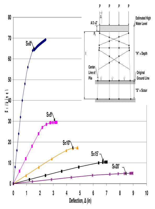
Figure B.48 HP12x53 Two-Story X-Braced 4-Pile Bent with H=25', P=160kips and A=6'
