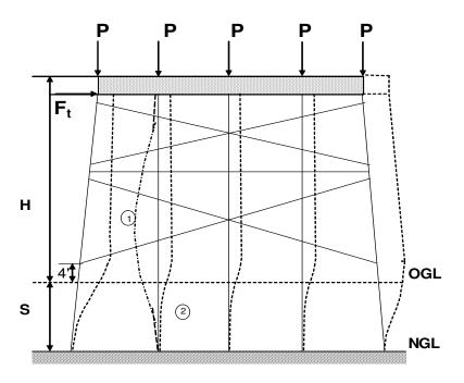
Figure 4.2 X-Braced Pile Bent Sidesway Buckling or Pushover Failure Load
