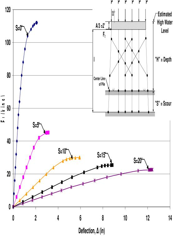
Figure B.96 HP12x53 Double X-Braced 6-Pile Bent with H=17', P=160kips and A=6'
