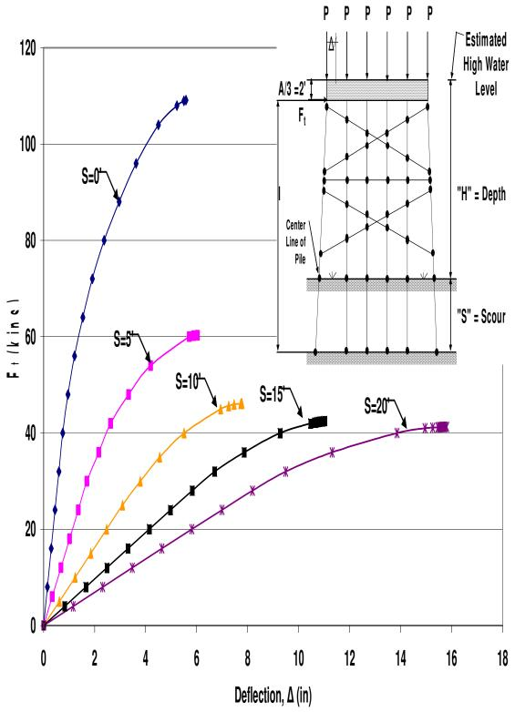
Figure B.97 HP12x53 Two-Story Single X-Braced 6-Pile Bent with H=21', P=100kips and A=6' Pushover Analysis Results 328
