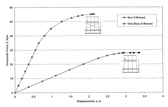
Figure 4.7 GTSTRUDL Pushover Analysis Results for HP10x42 4 Pile Bents, Bents Pinned at Ground, H=13ft, S=0ft
