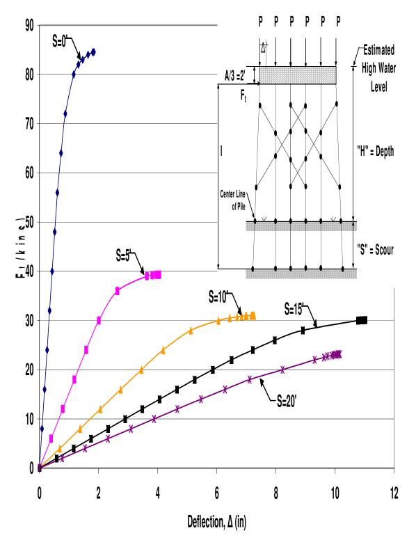
Figure A.89 HP10x42 Double X-Braced 6-Pile Bent with H=13', P=100kips and A=6'
