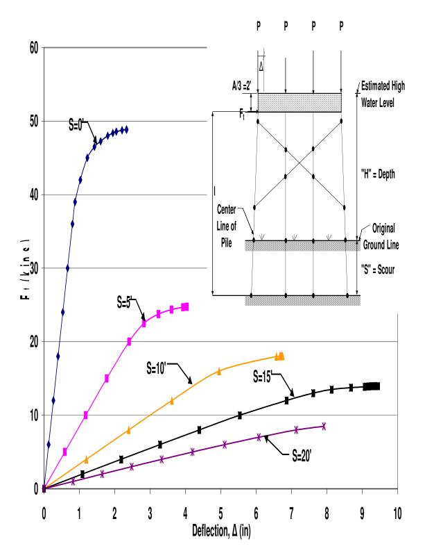
Figure A.37 HP10x42 X-Braced 4-Pile Bent with H=17', P=100kips and A=6'
