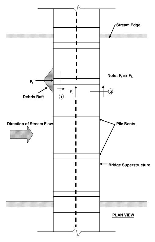
Figure 2.6 Typical Pile Bent Supported Bridge over a Stream
