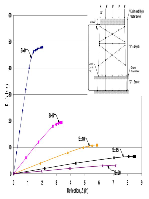
Figure A.71 HP10x42 Two-Story X-Braced 5-Pile Bent with H=25', P=140kips and A=6'
