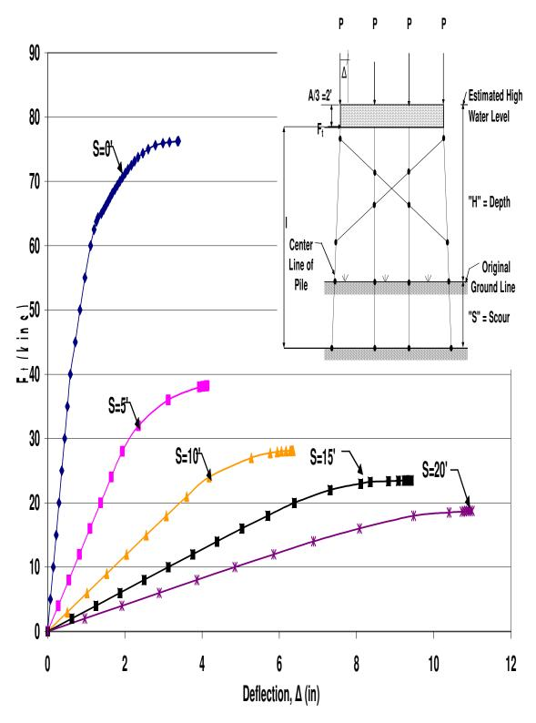
Figure B.38 HP12x53 X-Braced 4-Pile Bent with H=17', P=120kips and A=6'
