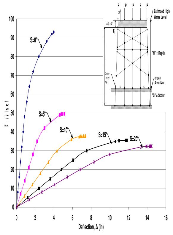
Figure B.69 HP12x53 Two-Story X-Braced 5-Pile Bent with H=25', P=100kips and A=6'
