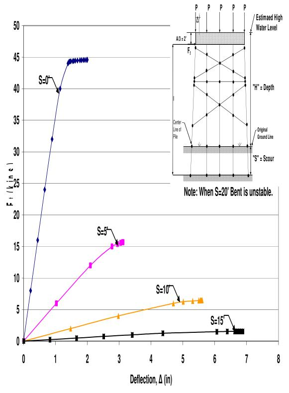
Figure A.72 HP10x42 Two-Story X-Braced 5-Pile Bent with H=25', P=160kips and A=6'
