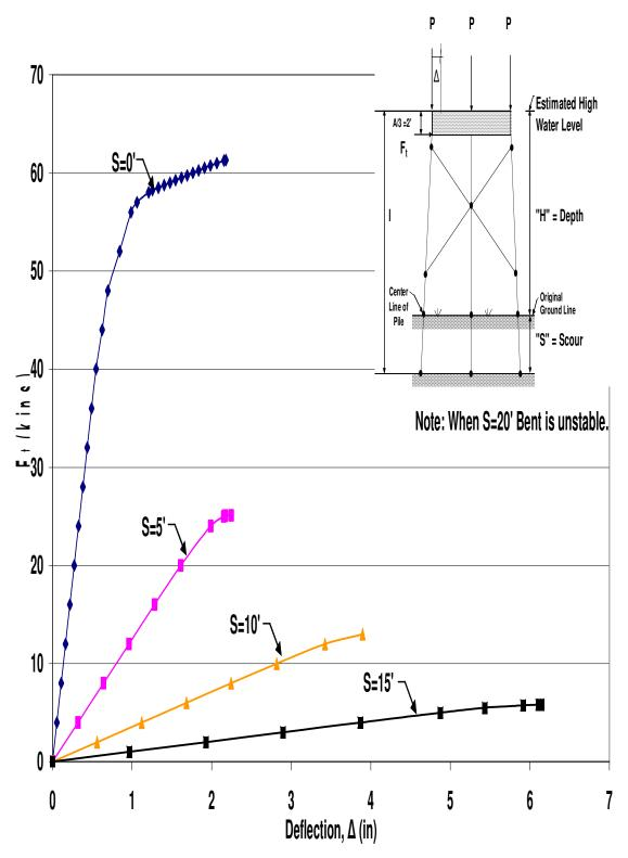
Figure B.14 HP12x53 X-Braced 3-Pile Bent with H=17', P=120 kips and A=6'
