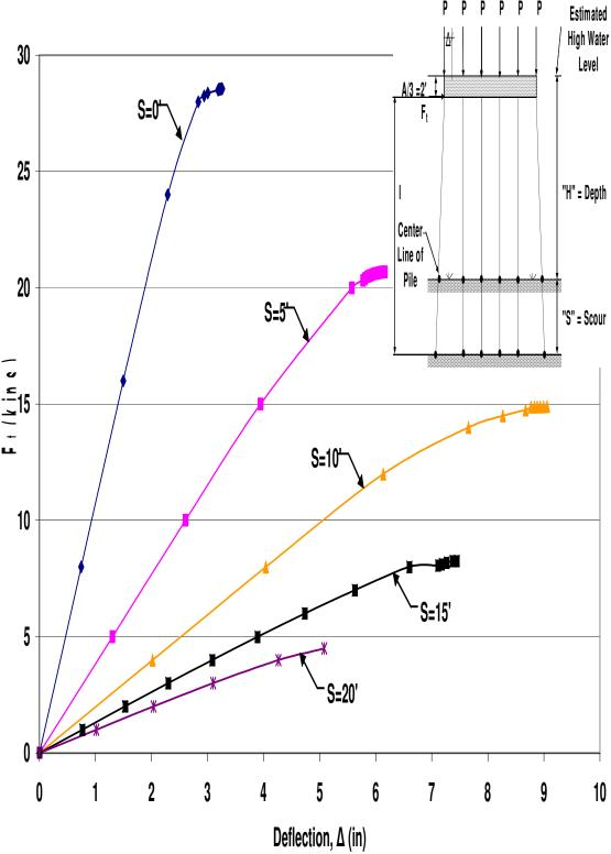
Figure A.80 HP10x42 Unbraced 6-Pile Bent with H=13', P=160kips and A=6'
