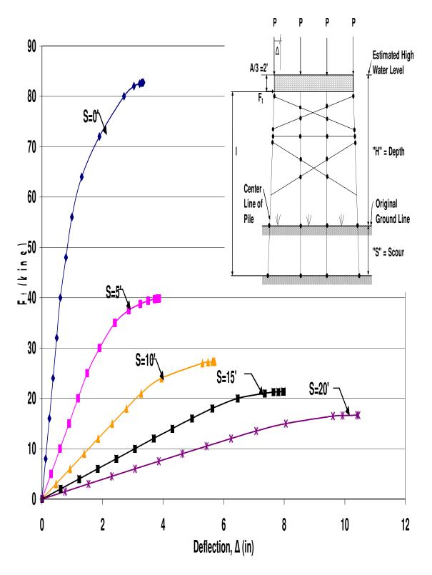
Figure B.42 HP12x53 Two-Story X-Braced 4-Pile Bent with H=21', P=120kips and A=6'
