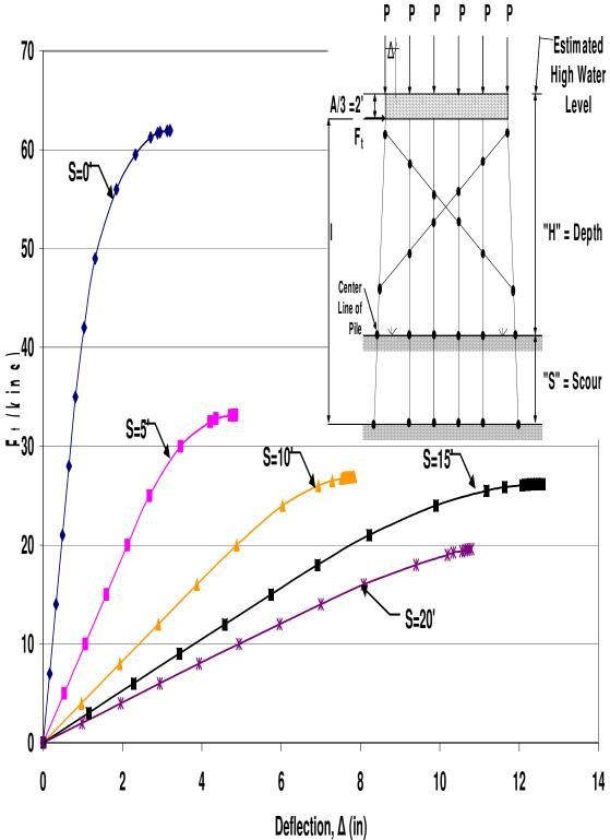
Deflection,  $\Delta$  (in) Figure A.85 HP10x42 Single X-Braced 6-Pile Bent with H=17', P=100kips and A=6' Pushover Analysis Results  $_{202}$
