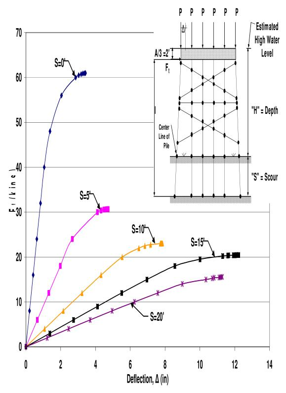
Figure A.101 HP10x42 Two-Story Single X-Braced 6-Pile Bent with H=25', P=100kips and A=6' Pushover Analysis Results
