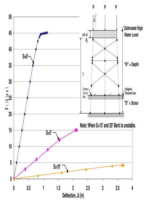
Figure A.18 HP10x42 Two-Story X-Braced 3-Pile Bent with H=21', P=120kips, and A=6'
