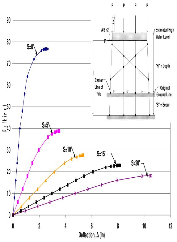
Figure B.35 HP12x53 X-Braced 4-Pile Bent with H=13', P=140kips and A=6'
