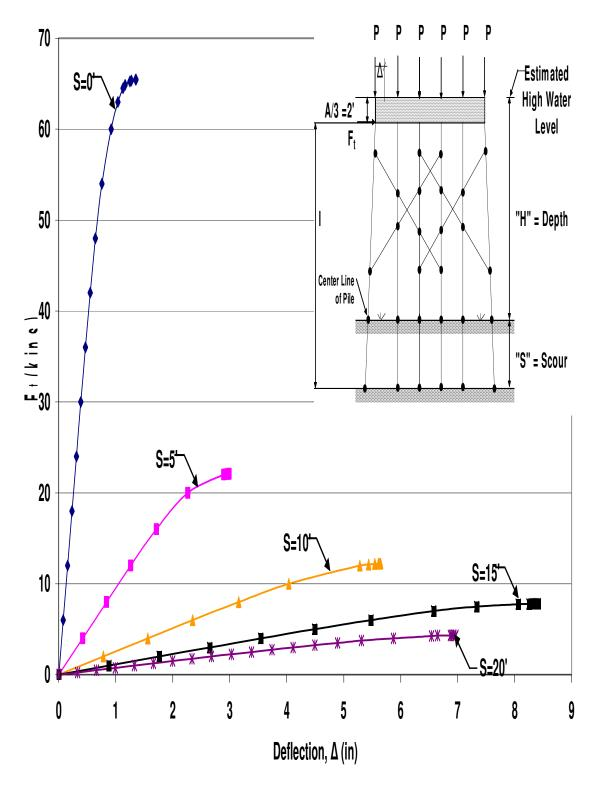
Figure A.96 HP10x42 Double X-Braced 6-Pile Bent with H=17', P=160kips and A=6'
