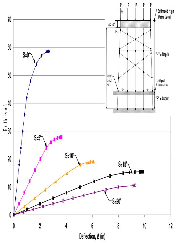
Figure A.66 HP10x42 Two-Story X-Braced 5-Pile Bent with H=21', P=120kips and A=6'
