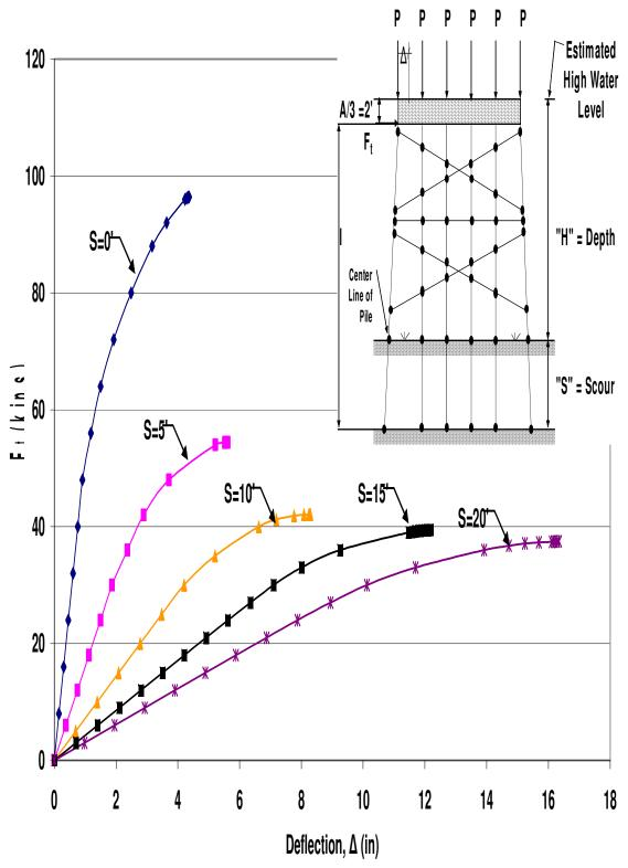
Figure B.101 HP12x53 Two-Story Single X-Braced 6-Pile Bent with H=25', P=100kips and A=6' Pushover Analysis Results 332
