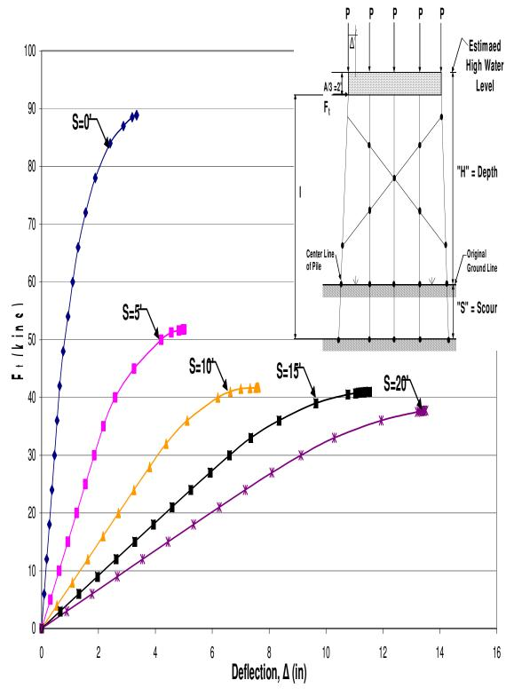
Figure B.61 HP12x53 X-Braced 5-Pile Bent with H=17', P=100kips and A=6'
