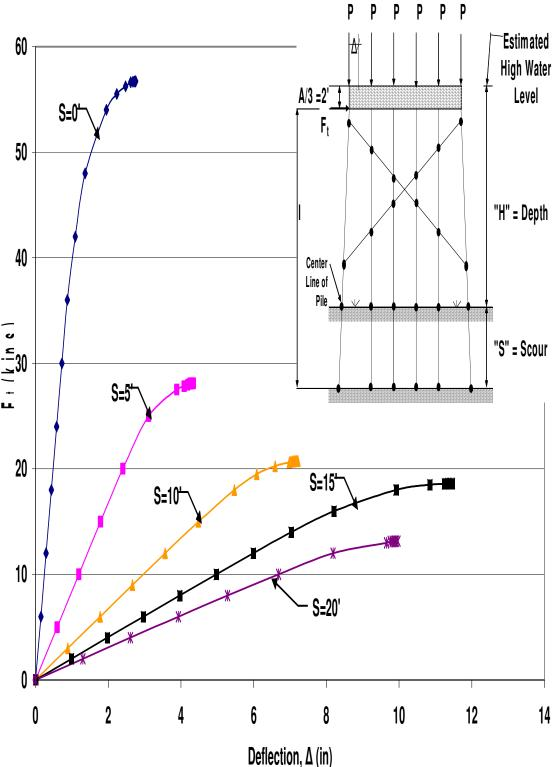
Deflection,  $\Delta$  (in) Figure A.86 HP10x42 Single X-Braced 6-Pile Bent with H=17', P=120kips and A=6' Pushover Analysis Results  $_{203}$
