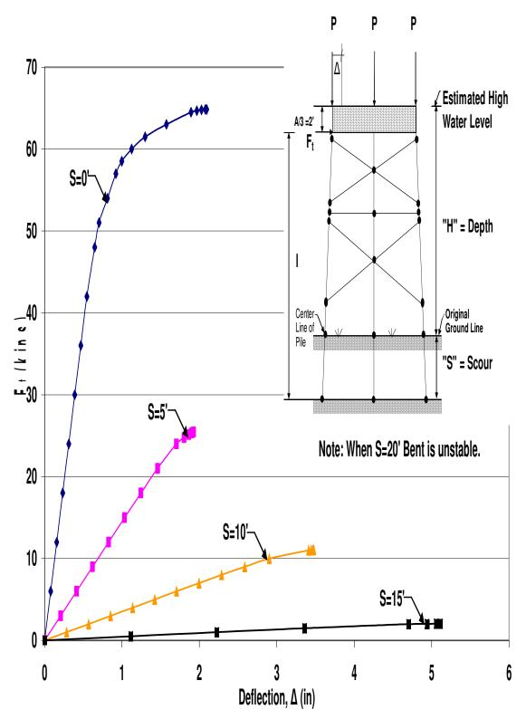
Figure B.20 HP12x53 Two-Story X-Braced 3-Pile Bent with H=21',P=160kips and A=6'
