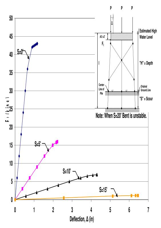
Figure A.9 HP10x42 X-Braced 3-Pile Bent with H=13', P=100kips and A=6'
