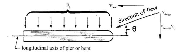
Figure 4.8 Plan View of Pier Showing Stream Flow and Lateral Pressure (AASHTO 1997)
