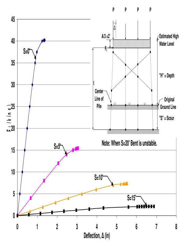
Figure A.40 HP10x42 X-Braced 4-Pile Bent with H=17', P=160kips, and A=6' Pushover Analysis Results
