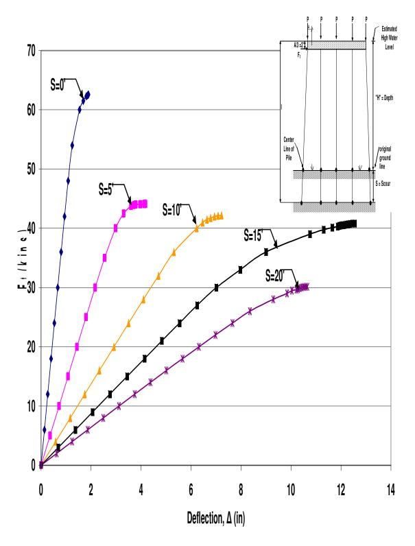
Figure B.51 HP12x53 Unbraced 5-Pile Bent with H=10', P=140kips and A=6'
