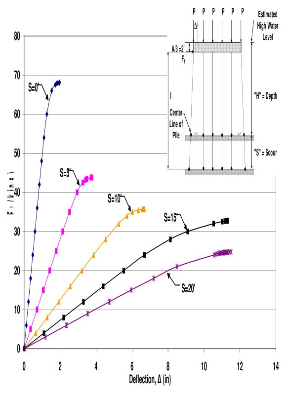
Figure B.76 HP12x53 Unbraced 6-Pile Bent with H=10', P=160kips and A=6'
