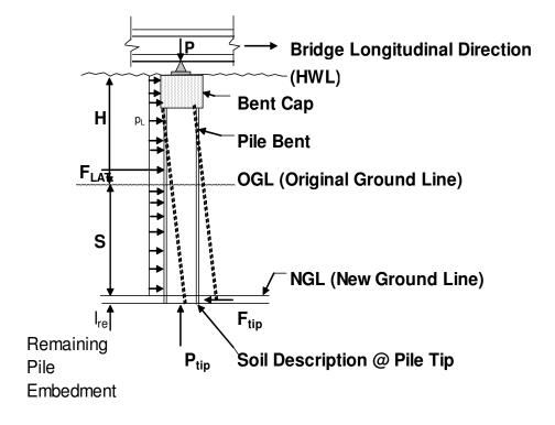
Figure 4.3 Evaluation of Bent Pile "Kick-Out" Load from Extreme Flood/Scour Event
