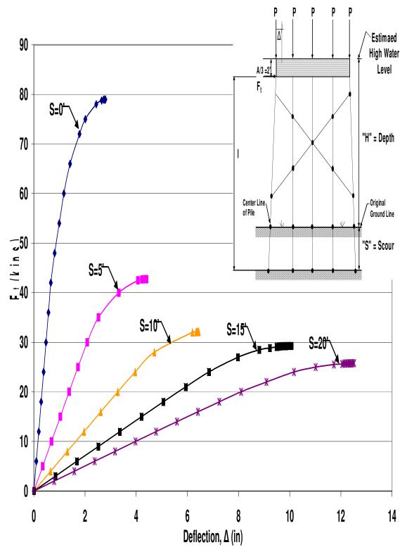
Figure B.63 HP12x53 X-Braced 5-Pile Bent with H=17', P=140kips and A=6'
