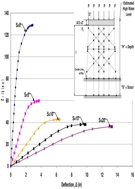
Figure B.106 HP12x53 Two-Story Double X-Braced 6-Pile Bent with H=21', P=120kips and A=6' Pushover Analysis Results
