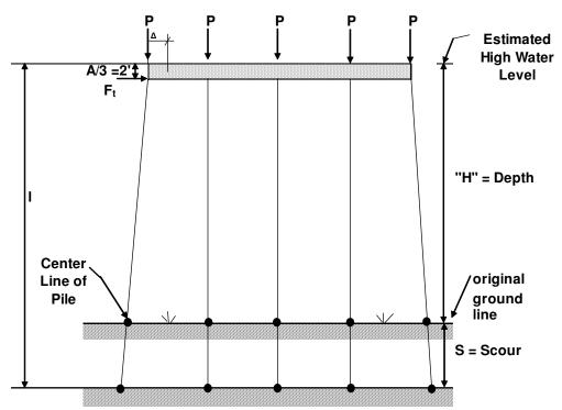
Figure 3.5 Typical Unbraced Bent and Typical Loading Conditions
