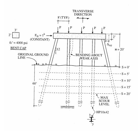
Figure 2.14 Pile Bent Analyzed to Determine P- $\Delta_{top}$  Curve in Transverse Direction
