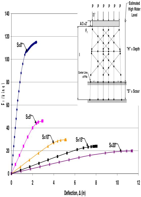
Figure B.112 HP12x53 Two-Story Double X-Braced 6-Pile Bent with H=25', P=160kips and A=6' Pushover Analysis Results
