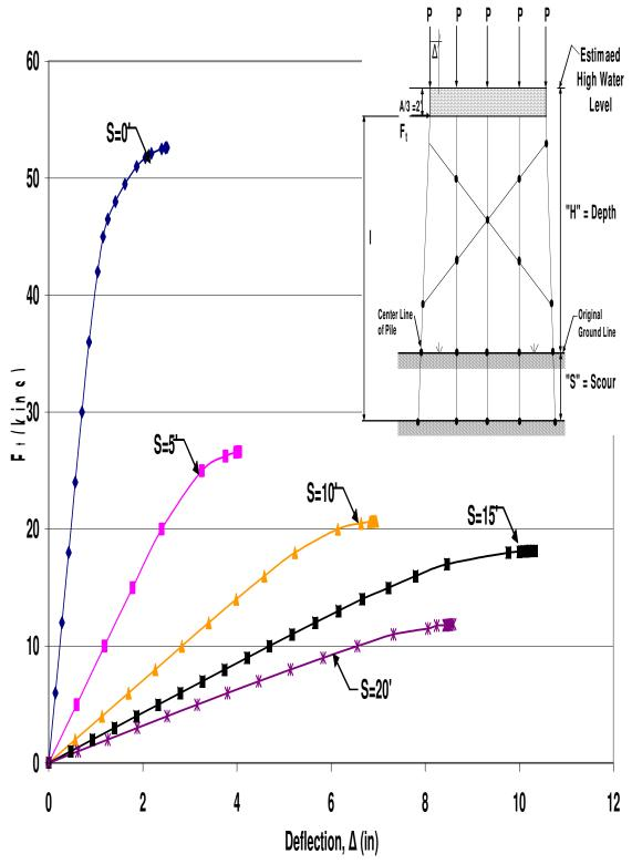
Figure A.62 HP10x42 X-Braced 5-Pile Bent with H=17', P=120kips and A=6'
