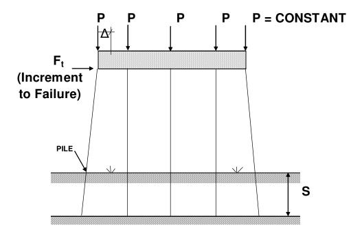
a. Gravity + Flood Water Loaded Pile Bent
