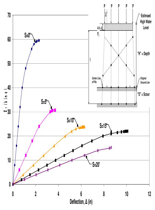
Figure A.58 HP10x42 X-Braced 5-Pile Bent with H=13', P=120kips and A=6' Pushover, Analysis Results
