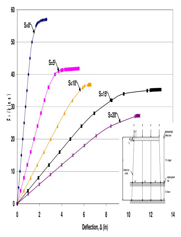
Figure B.25 HP12x53 Unbraced 4-Pile Bent with H=10', P=100kips and A=6'
