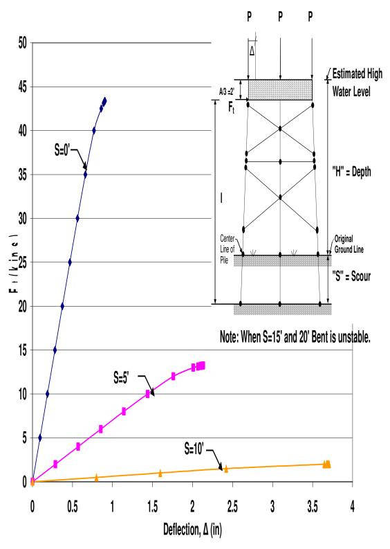
Figure A.19 HP10x42 Two-Story X-Braced 3-Pile Bent with H=21', P=140kips and A=6'
