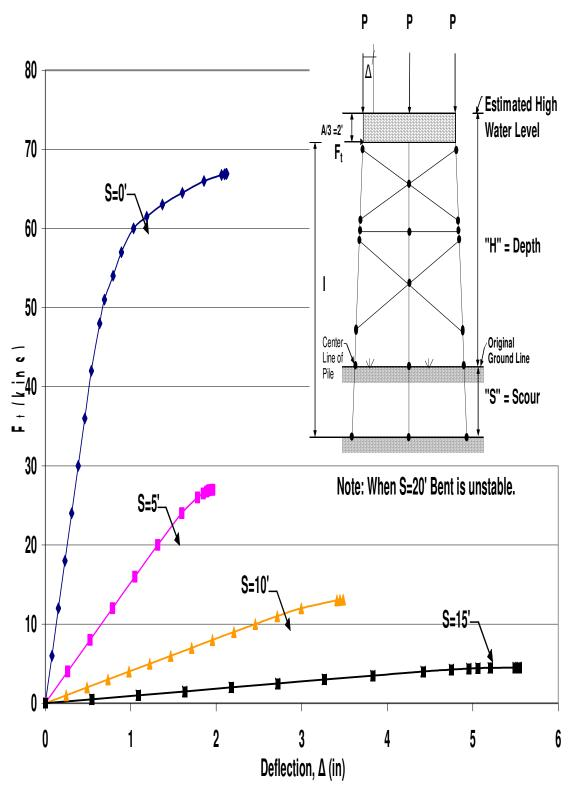
Figure B.19 HP12x53 Two-Story X-Braced 3-Pile Bent with H=21',P=140kips and A=6'
