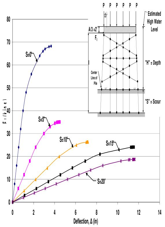
Figure A.97 HP10x42 Two-Story Single X-Braced 6-Pile Bent with H=21', P=100kips and A=6' Pushover Analysis Results
