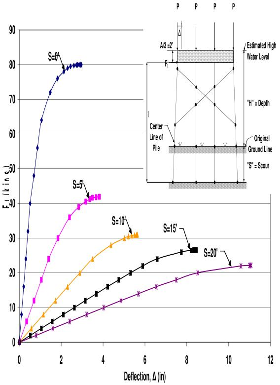
Figure B.34 HP12x53 X-Braced 4-Pile Bent with H=13', P=120kips and A=6'
