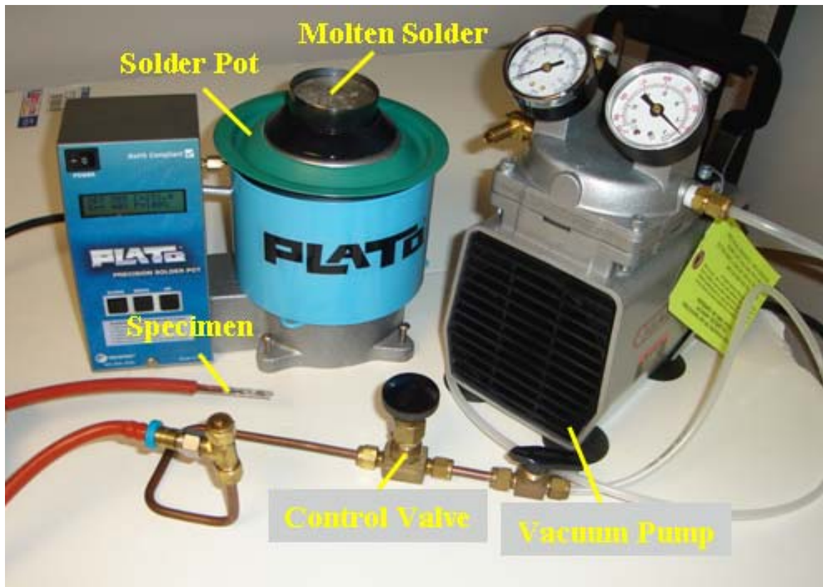
Figure 59: Bimaterial Cu-solder specimen preparation set-up with control valve of vacuum pump
