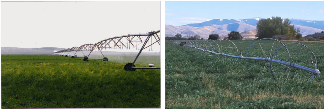
Figure 2.2 Linear and wheel line irrigation system
