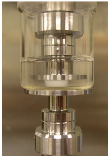
Figure 4.3 DMA experimental setup for testing the compressive mechanical properties of swollen hydrogels immersed in deionized water at room temperature
