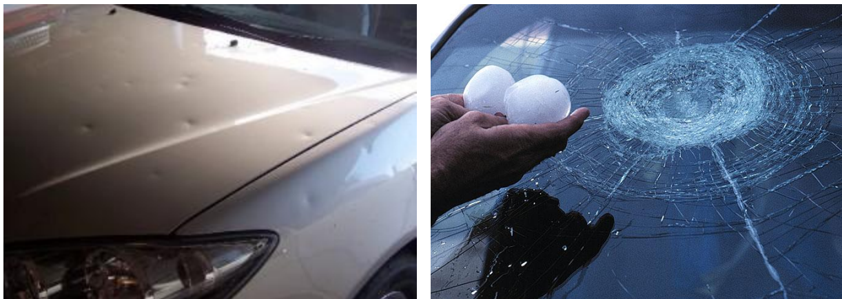
Figure 3 Vehicle damage caused by hail
