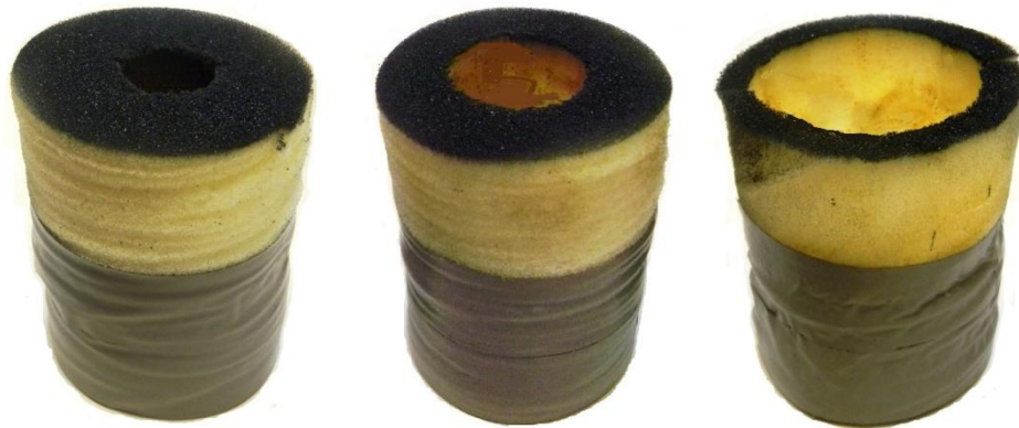
Figure 34 Foam sabot for varying diameter projectiles
