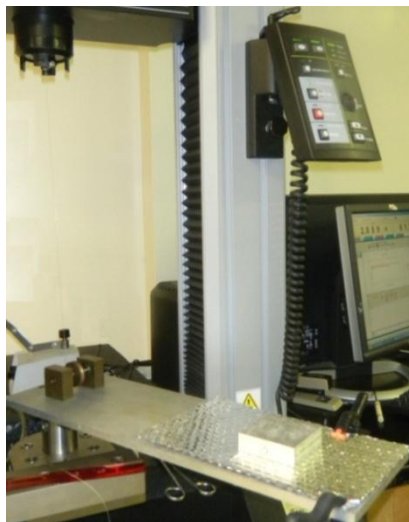
Figure 17 Friction test fixture
