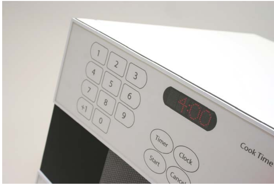
Detail shot of contact switches and clock.
